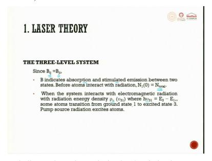
So, here  $B_{ij}$  = $B_{ji}$ . B indicates absorption and stimulated emission between two states. Before atoms interact with radiation  $N_1(0)$ =  $N_{total}$ . When the system interacts with electromagnetic radiation with radiation energy density,  $\rho_{\upsilon}$  ( $\upsilon_{31}$ ) where  $h\upsilon_{31}=E_3-E_1$ , some atoms transition from ground state 1 to excited state 3. Pump source radiation excites atoms.
