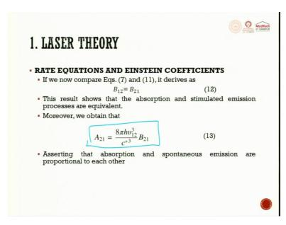
So, I was talking to you about two level system and three level systems. In two level system, for stimulated emission to produce a laser beam or amplifying light the stimulated emission rate must be higher than the spontaneous emission.
