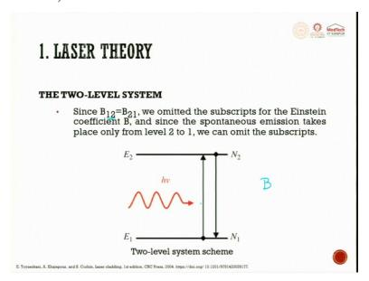
So, this is a two-level system. Since  $B_{12}$  and  $B_{21}$  are equal, we omit the subscript for the Einstein coefficient B and since the spontaneous emission takes place only from level 2 to 1 we can omit the subscript one to two or two to one, that is why we write it as B a constant, so this is two level system.
