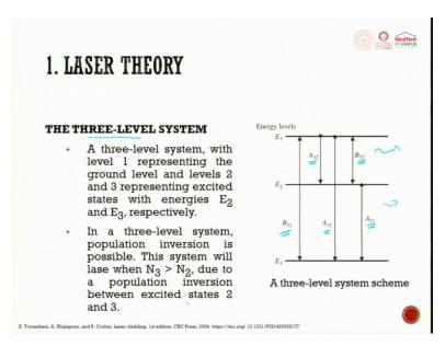
So, as I told you there are three level systems also. In a three level system population inversion is possible. This system will lase when N3 is greater than N2 due to the population inversion between the excited state 2 and 3.
