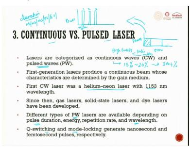
When we go to the next level of understanding of laser, we should try to understand what is continuous laser and what is pulsating laser. So, the continuous laser versus pulsating laser. Continuous means it is like this so, you have a constant power coming up this constant power. If you have a very high energy, then you can use it for sintering or melting but this is continuous. When we have a same laser but now what we do is we chop it off and we try to have the same energy here.
