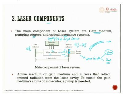
When we try to look at the lasing components, main components of the lasing system are gain medium, pumping source and optical resonance. Optical resonance is nothing but where there is a back and forth movement going on, gain medium means where you try to focus and gain things, pumping source means what tries to excite the ground level.
