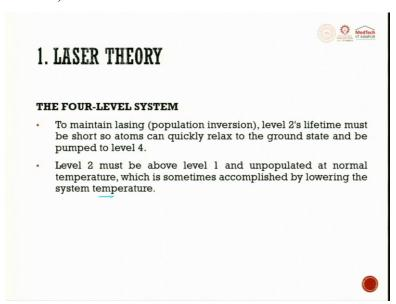
So, to maintain lasing, level 2 lifetime must be shorter. So, atoms can quickly relax to the ground state and go back to the level 4, level 2 must be above level 1 and unpopulated at normal temperature which is sometime accomplished by lowering the system temperature. So, this is where we use heat management as a tool.
