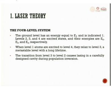
So, the ground level has an energy equivalent to  $E_1$  and is indicated by 1, the levels 2, 3, and 4 are excited states and their energy levels are  $E_2$ ,  $E_3$ , and  $E_4$  respectively. When level 1 atoms are excited to level 4 they relax to level 3 and a meta stable level with a longer lifetime. So, that means to say it has a longer lifetime. From 3 to 2 it causes lasing action and then it tries to come down.
