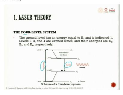
So, you have also four level as I told you. So, from here it gets excited to this level, from here non radiative fast decay happens up to 3. So, from here it goes, lasing action happens here, from here to here it goes down. So, you can see pumping action and lasing action, when it goes to this level. So, here non radiative fast decay will happen, it will try to be more efficient when we use a four level system.
