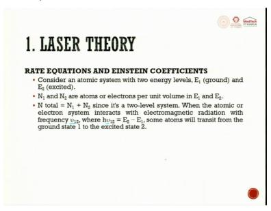
So, the rate equation and the Einstein coefficient which are always used. So, consider an atomic system with two energy levels  $E_1$  and  $E_2$  the number of atoms present are  $N_1$  and  $N_2$  are the atoms or the electrons per unit volume in  $E_1$  and  $E_2$  the total  $N=N_1+N_2$  since it is two level system, you can also have three level system, four level system.
