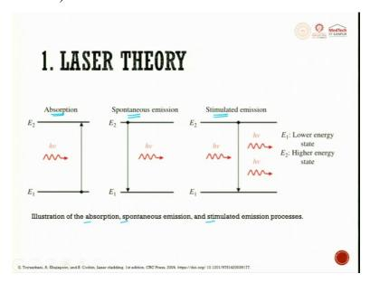
So, this is what I have explained. So, just one quick recap of it, from E1 it goes to E2 this is what is the pumping happening. So, this is called as the absorption phase the next one is called as the spontaneous emission. So, from the top it drops down, when it drops down it tries to give out, hu that is spontaneous.
