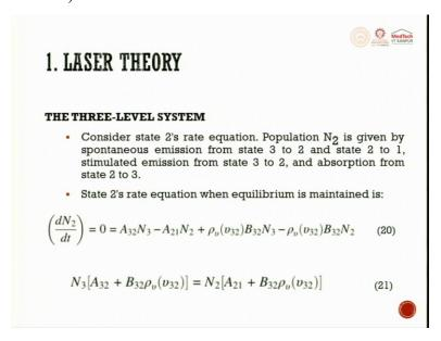
So, three levels. So, the second rate equation is given by the spontaneous emission from state 3 to 2 and state 2 to 1. So, the stimulated emission from 3 to 2 and absorption from 2 to 3. So, the state two rate equation when equilibrium is maintained will be like this:
