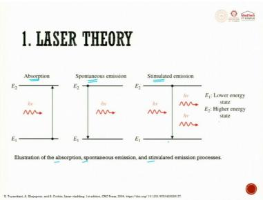
When the incoming photon induces the emission, the process is called as stimulated emission. In stimulated emission the emitted photon matches with the stimulated photon phase in terms of phase, frequency and polarization.
