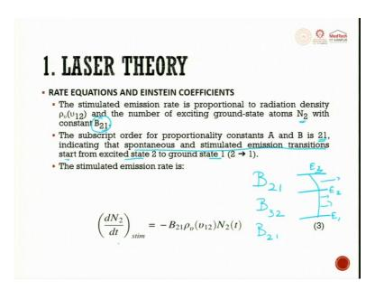
So, this stimulated emission rate is proportional to radiation density. Radiation is what comes out. Radiation density and the number of excited ground state atoms  $N_2$  with respect to a constant is called  $B_{21}$ . The subscript order for proportionality constant A and B is 21 indicating that spontaneous and simultaneous emission transition starts from excited state 2 to the ground state 1 that is why we call this constant  $B_{21}$ . The stimulated emission rate is:
