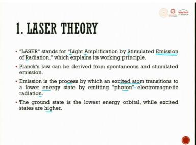
When an electron jumps so this is a lower level, this is a higher level, you have an atom here this, when you try to hit it with a photon this gets excited. So, from lower to higher it cannot stay in the higher for a longer time. So, it will come back to the lower. So, when it is coming back it is called as emission.
