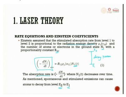
Einstein assumed that the stimulated absorption rate from level 1 to level 2 is proportional to the radiation energy density and the number of atoms or electrons in the ground state  $N_1$  which is proportional to a constant called  $B_{12}$ .
