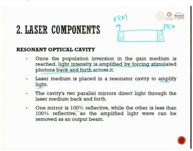
Once the population inversion in the gain media is reached, the light intensity is amplified by forcing stimulated photons back and forth across, that is why I told you there is a medium. So, this is fully reflecting mirror, this is partially reflecting mirror.
