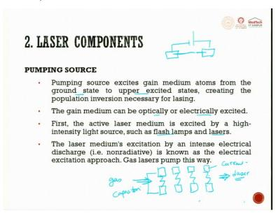
The pumping source excites gaining medium atoms from a ground state to an upper excited state creating population inversion necessary for lasing action. The lasing media can be optical or electrically excited. You can use a very high power and then also you can do like an arc.
