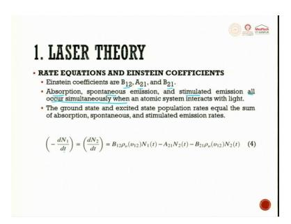
So, now  $B_{12}$ ,  $A_{21}$  and  $B_{21}$  are all Einstein coefficients which can be directly pulled out from some literature you can get these constants, absorption, spontaneous emission and stimulated emission all occur simultaneously when an atomic system interacts with light. The ground state and the excited state population rate equals the sum of absorption, spontaneous emission and stimulated emission.
