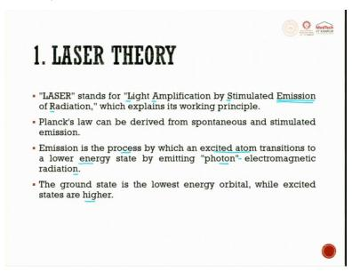
Laser stands for light amplification by stimulated emission of radiation. Planck's law can be derived from the spontaneous and simultaneous emission. Emission is nothing but a process by which an excited atom transitions to a lower level by emitting photons-electromagnetic radiation, emission is a process. The ground state is called as the lower energy orbital while the excited state is called as the higher one we will see that in detail in the next slide.
