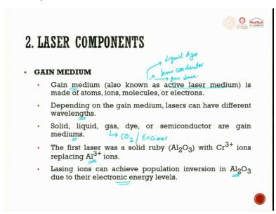
Gain medium, also known as active laser medium is made of atoms, ions, molecules or electrons. Depending on the gain medium, the laser can have different wavelength. So, this is what, so you can have a semiconductor laser, you can have a gas laser, you can have a liquid dye laser, all these things are now the gain medium.
