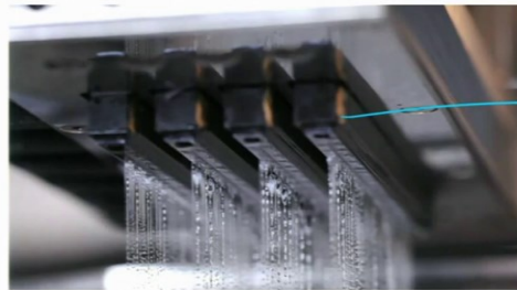
Binder jetting technology in Action
