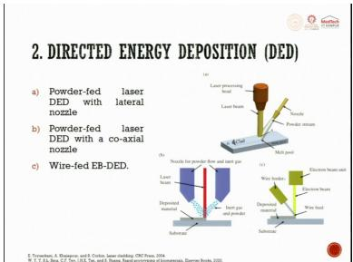
By articulating the nozzle or substance, here you will see that there will be a nozzle, and these nozzles will be articulated. So, by articulating the nozzle or substances the filler material confocal point follows a predefined 3D path to deposit neighboring track, predefined 3D path.
