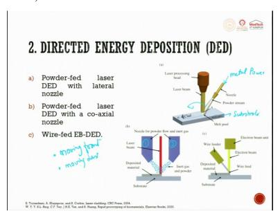
There are three techniques which are used, in generally three techniques which falls under Direct Energy Deposition, DED. One is powder fed laser DED with lateral nozzle. Next one is powder fed laser DED with coaxial nozzle. The third one is wire fed electron beam DED method.
