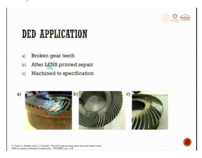
So, DED finds lot of application in broken gear teeth, which you cannot replace the entire casting. So, you will try to do some modification here and try to bring it back to the original version. So, after LENS is a process, we will see that in detail later. After lens printed repair or machined to specification, these are the places where you will see the DED finds lot of application.
