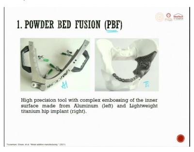
So, high precision tool with complex embossing of the inner surface made from aluminum and lightweight from titanium are shown here, which is all build by powder bed fusion method.
