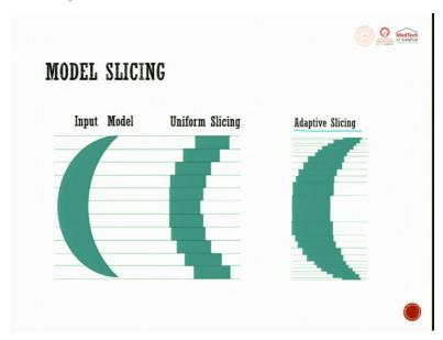
So, this is the input one this is uniform slicing. So, here whatever might be the curve change, I tried to slice it in a very uniform manner. So, you get a uniform slice, but when we try to do adaptive slicing, wherever there is a change in geometry more than a particular sub slope change, we try to slice it, we try to fix that slope angle and if it crosses that slope angle immediately a slice is drawn.
