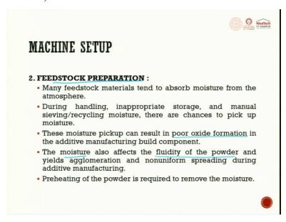
Then feedstock preparation, many feedstock materials tend to absorb moisture. So, we have to be careful. Even the metal powder can absorb moisture during handling inappropriate, storing and manual sieving recycling moisture, there are chances to pick up the moisture so they all can happen. And once the moisture is picked up, when we do SLS or SLM process, there is a problem of generating porosity.
