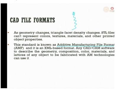
STL which is very commonly used is nothing, but stands for Stereolithography. It is the most common AM format, this file format specifies ASCII or binary representation of 2D and 3D objects surface geometry. The only thing which is missing in STL is it will not have any colour or texture details.
