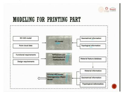
Modelling for printed parts you will have 3D CAD model you can also extract it from point cloud data, this point cloud data comes from the reverse engineering where in which you use a laser and you try to scan the details. So that is point cloud data. So, that is given to an STL
