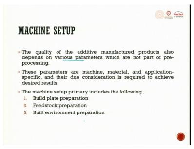
When it goes to the machine setup, the quality of the additive manufactured product also depends on various process parameters and not on part pre-processed preparation. These parameters are machine, material, application specific, and their due consideration is required to achieve the results.
