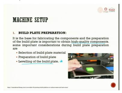
So, this is build plate preparation. So, this is the build plate. When we do DED, build plate is important, even when you do material extrusion. It is the base of the fabricating, the component, and the preparation of the build plate is important to obtain high quality components.
