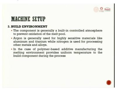
Build environment. The component is generally a built-in controlled atmosphere to prevent oxidation of the melt pool. Argon is generally used for highly sensitive material like aluminium and titanium while nitrogen is used for processing of other metals and alloys. In case of polymer based additive manufacturing, melting environment provides uniform temperature to the build component during the process. So, build environment is also very important.
