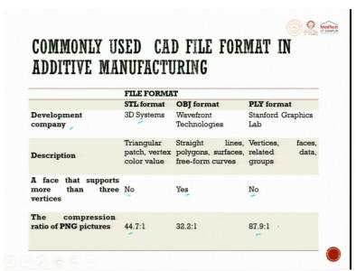
Commonly used CAD file formats in Additive Manufacturing developed by the company 3D systems is STL format. OBJ format is by wavefront technologies and the PLY format is by Stanford graphic lab. We use triangle patches, and vertices colour values in STL format, when you go to OBJ we use straight polygon and freeform surfaces, Straight Line, Polygon surface and freeform curves. When we talk about PLY format, vertices, faces related data and groups are used.
