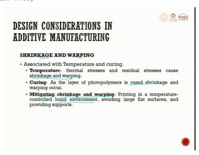
So, when we try to design additive manufacturing, some of the challenges are shrinkage and warping. They both are associated with temperature. So, we would like to look at temperature
