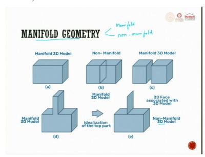
There is another interesting thing in CAD, which is manifold geometry. So, in manifold geometry you have manifold 3D model. So, this is a manifold 3D model, this is a non-manifold 3D model. So, you can have manifolds so you split it down and then you have manifold 3D model like this. So, then in ideation on the top place, you will have something like this. So, 2D phase is associated with a non-manifold 3D model.
