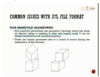
So, what are non-manifold geometries? Non-manifold geometries are geometrical topological terms that allow all disjoining lumps to exist in their own logical body, it can be simply understood with manufacturability.
