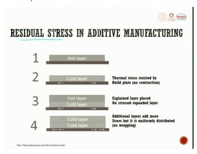
So, there is always residual stress, which is getting imbed in the part while printing through additive manufacturing, especially polymer, as well as metal is concerned. So, what we do is we always have a hot layer. So, there is a hot layer we keep, and then we also try to have cold layer.
