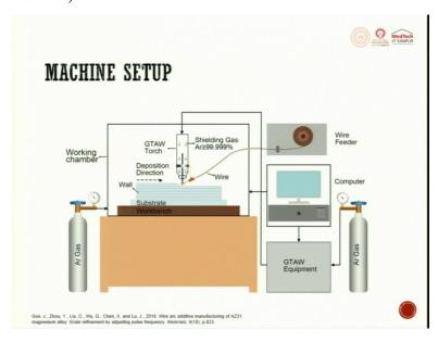
So, this is the machine set up. You can have a wire which comes here. You can have a shielded gas. This is for wire, DED. You can have powder. So, you will have argon where in which they maintain the working chamber temperature and pressure such that the oxidation does not happen.
