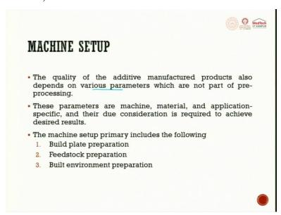
Three important steps in machining setup is build plate preparation, feed stock preparation, and built environmental preparation.
