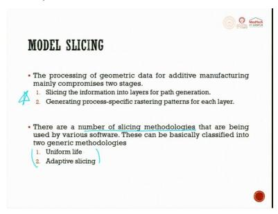
Now, let us move from STL into slicing model. The process of slicing of geometric data for additive manufacturing mainly composes of two stages. One is slicing the information into layer for path generation, next one is creating process specific rastering pattern for each layer, these two are very important, when we are trying to do slicing, you will have these two till now whatever we studied about STL everything is done.
