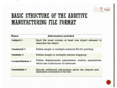
So, the basic structure of Additive Manufacturing file format is going to be object, material, texture, constellation and meta data. So, object in each file must contain at least one object
