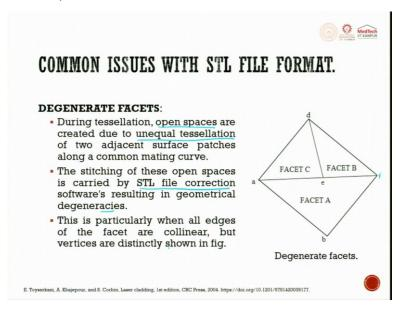
Next is you can have degenerated facets, Degenerated facets means during tessellation, your open space are created due to unequal tessellations. Open spaces have to adjust and surface patches along your common mating surface, you will have mating surface, you will have unequal tessellation stitching of these open space carried out by STL file correction software resulting in geometrical degeneracy.
