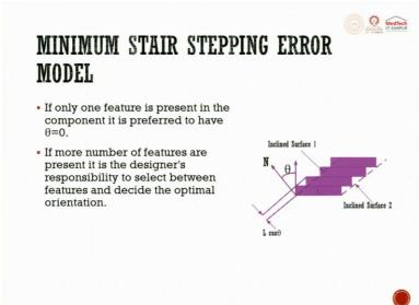
How do we calculate the Minimum Stair Stepping Error model? We are trying to calculate the staircase effect. So, staircase consider a planar volume, the stair stepping volume is the sum of each stair. Each stair step, which is a function of surface area and inclination that surface makes with the build a plane. So, this is the staircase.
