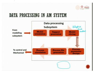
When you look into the data processing in AM systems, from the model subsystem you will try to have model orientation, then support generation, then you will have model slicing, then process parameter, design process, file generation, process simulation and then you try to get the final part to control and mechanical.
