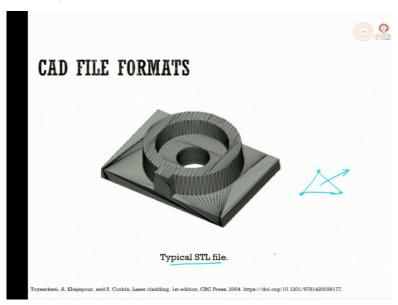
This is a typical CAD drawing. In this, CAD drawing have been converted into STL files, you can see here that these the object is converted into several soft small facets and these facets are linked. So, each facet finally if you look in detail, it will be like this we will have three vertices and a normal. So, this is a STL file when you store the file a \*.STL, \*.AMF then you will get all this information for STL files.
