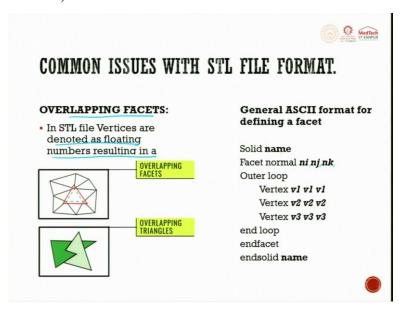
There can be other issue of overlapping facets. For example, the STL file vertices are denoted as floating numbers resulting in overlap facets. So, if you see here, generally ASCII format defines a facet solid name facet  $n_i$ ,  $n_j$ ,  $n_k$  over the outer loop is v1x,y,z, v2x,y,z then v3x,y,z. So, end of loop this is how the ASCII format file looks like for a facet.
