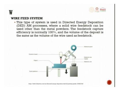
Wire feed system wherever till now, we were talking about powder you are today using wire. So, it is easy for you to transport the wire and melt and deposit it. So, a wire feeding system is nothing but feeding a wire instead of a powder and using laser for melting and trying to adhere to form parts.
