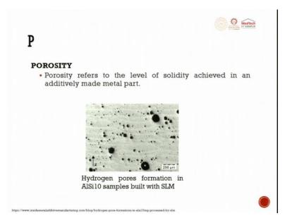
Porosity- Porosity refers to these all holes which are getting formed to the level of solidity achieved in the additively made metal parts. So, you can have porosity because of hydrogen per cent or any other foreign material which are present.
