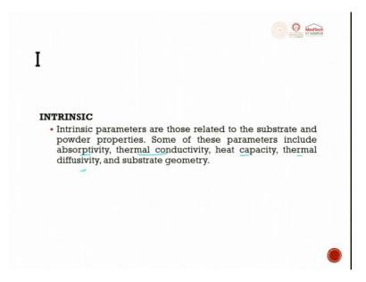
Intrinsic properties. For any given material there are extrinsic properties and intrinsic properties. Intrinsic parameters are those related to the substrate and powder properties. Some of the parameters include absorptivity, thermal conductivity, heat capacitance, thermal diffusivity and substrate geometry.
