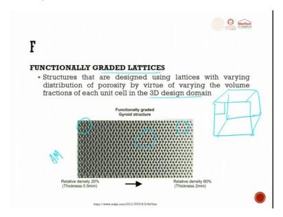
Functionally graded lattice, so, when we start looking into building up a solid object, we will now divide the solid object even in material sciences to unit cells. So, now, if you start playing with the properties changing the properties of lattice, so, this unit cell is called as lattice right. So, if you are trying to play or change this lattice, then you are trying to get
