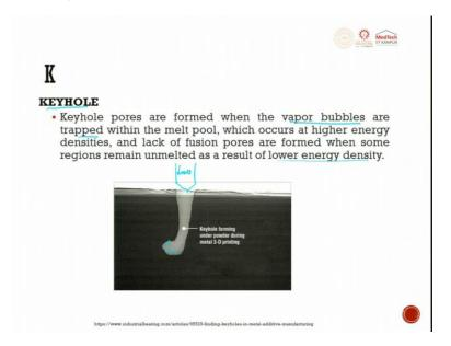
While the laser interacts with the material, we always have something called a keyhole process. This is a laser, which is hitting the surface, laser hitting the surface. So, keyhole pores are formed when the vapor bubbles are trapped within the melt pool, which occurs at a higher energy density and lack of fusion pores are formed when some of the regions remain
