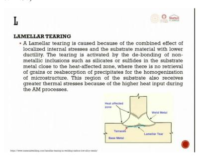
What are Lamellar tearing? Lamellar tearing is caused because of the combined effect of localized internal stresses and the substrate material with lower ductility. This tearing is activated by de-bonding of a non-metallic inclusion such as silicate or sulfide in the surface. So, these are the Lamellar tearing, these are traces, tearing is caused because of a combined effect of localized internal stresses and substrate material with lower ductility.
