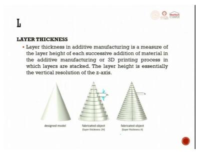
Layer thickness- layer thickness you can have varying layer thickness in additive manufacturing as a measure of layer height of each successive addition of material in additive manufacturing or 3D printing process in which layers are stacked. So, layer thickness is what is the layer thickness it has, you can have the same layer thickness all across the component, and you can have varying layer thickness across the components. So, that is called as adaptive slicing methods.
