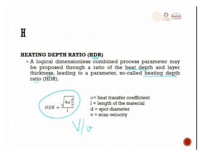
Heating depth ratio which is another important one which is called as HDR it is again a logical dimensionless combined process parameter may be proposed through a ratio of heat depth and the layer thickness, effective layer thickness, nominal layer thickness here, there is one more heat depth by layer thickness. So, this is another parameter so-called heating depth ratio. So, this can be derived by this formula.
