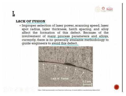
Lack of fusion, improper selection of laser power, scanning speed, laser spot radius, layer thickness, hatching spacing, alloying affects the formation of this defect, because of the involvement of many process parameters and alloys. Currently, there is no general available methodology to guide engineers on how to avoid these defects. Lack of fusion is another major thing which happens due to process parameters in laser.
