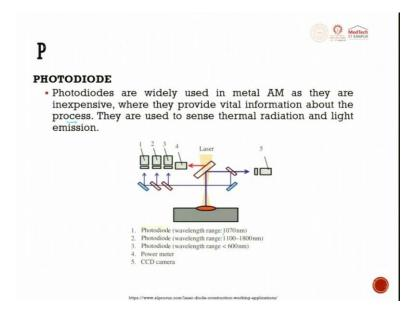
Photodiodes, photodiodes are widely used in additive manufacturing, as they are inexpensive when they provide vital information about the process. So, photodiode talks about the intensity of the profile, all these things are wavelength, intensity of the profile, then the peak distribution, all these things are directed by the photodiode.
