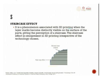
When we are trying to do layer by layer approach you will always have here something like a staircase which is getting formed. So, this defect is called a staircase defect or effect, it is a phenomenon associated with 3D printing when the layer marks become distinctly visible on the surface of the part giving the perception of the staircase. So, this is called the staircase, the staircase effect is omnipresent in 3D printing irrespective of the technology chosen.
