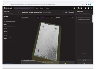
Let me come back to the screen where the component is shown already internal view is seen and then print is well, let us see the internal structure of the component. So, let me try to see the part settings at the right side. Copy this part to modify its settings. There are three options general, setting and infill. In the general option it is only showing the material that is to be printed here, material, then we have the furnace type that is Sinter 2, we have printer type.
