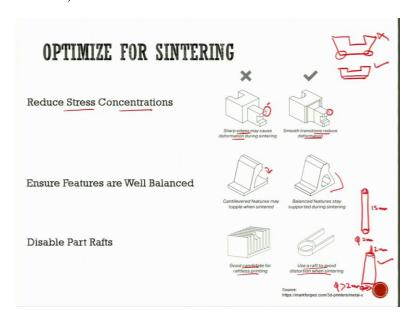
Now, for sintering there are certain suggestions, reduce the stress concentrations because in the sintering contraction has to happen, in the contraction the edges here you can see this, this edge here and this edge here this is a chamfered edge. So, we smoothen the transition to reduce the deformation, in the sharp edges may cause deformation during sintering because this sharp edges would induce in themselves, the thermal stresses.
