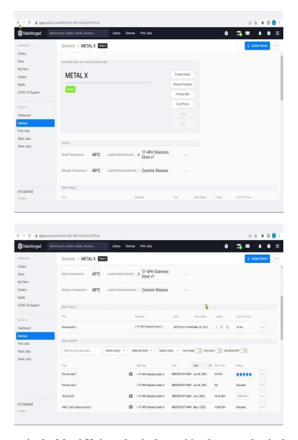
So, if I need to see in the Metal X that what is the position here or what is the situation here. So, in the screen it is showing that temperature metal temperature is 45 °s, release temperature 48 °s of the print right now and the loaded material is this and this is the position or the status of the metal X printer that is showing the pattern is ready because the stainless steel is already loaded there.
