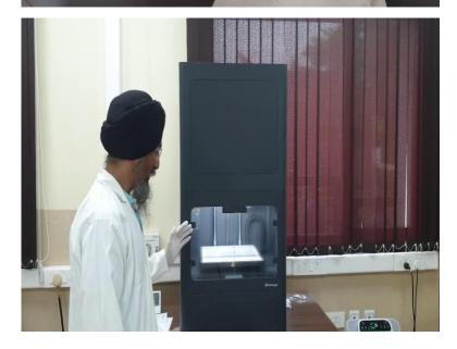
So now we are again back to that position where we will show you how we open the printer, how does operation start and the steps in that? First step is creating vacuum, vacuum is very important, so that the layer, this material gets stick to the plate. So, he has opened the window now. We will show you the description.
