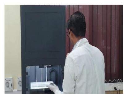
So, So, wherever we need more precision or more close features or small features that orientation of the print is always put in X and Y direction. For example, if I have to print this injection, if I need better resolution on this side, a bit on the height side I will put it in this direction because in X Y, X and Y direction the resolution or the precision will be better, in Z direction the precision is little lower.
