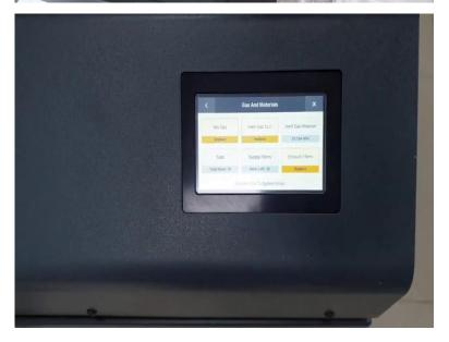
Sinter now we have move to the third section of the printing setup, that is this sinter. We have Sinter-2 setup here, which is the biggest sinter that the company has produced till date. Now, we will show you how do you open this sinter. The sinter is a big furnace actually. Its temperature can rise up to thousands of degrees.
