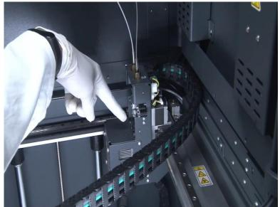
So, let us now come to the main printer volume here. So, if we come to the manual control here it is showing print bed metal nozzle, some options are being shown here. Home bed, if I click home bed here, it will try to do homing for the bed. Homing for the bed means it should try to bring bed to a position and try to see whether the nozzle and the bed head could work to the all the extremities.
