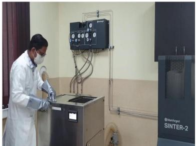
Where is taking straight to the wash section. You can see Markforged wash one, wash one is the well section. He is wearing mask, why, because wash has two major sections, one is the dry section, one is wet section. Wet cleaning is done to a chemical that is known as Opteon SF79. It is a liquid that is put. In that wet section this component is left to be dipped to be completely soaked for several hours.
