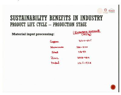
So, in the material input processing another data set that is provided in the same publication, they have given the embodied energy in metal powder materials. For example, the materials that have given are copper, aluminum, steel and zinc along with nickel. So, it is given the energy that is embodied energy in mega joules per kg. This energy is maximum for aluminum, which is in the range of 160 to 230 mega joules per kg.
