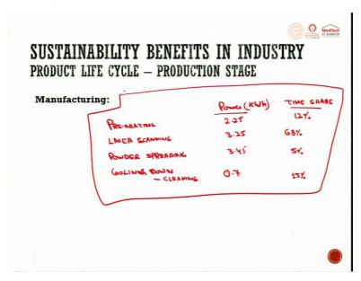
Now, in manufacturing if we try to compare the different steps in manufacturing. For example, the four steps how do they draw and time shared in the fabrication stages. So, let me say the first step is preheating, same researchers give the comparison or the study of the power consumed and the time shared, it has taken in the power.
