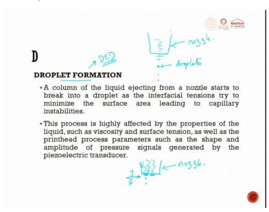
Droplet formation the column of liquid ejected from the nozzle starts to break down into droplets. Say for example, when there is a liquid which comes out of the nozzle assuming that the liquid comes out from the nozzle. So, then what is injecting from the nozzle, it starts to break down into droplets these are all droplets, breaks down into droplets as the interfacial tension tries to minimize the surface area leading to capillary instability.
