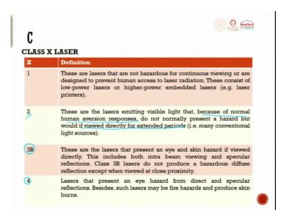
So, when we try to define about laser, laser is defined by various class. So, you can have class 1, class 2, class 3 B, class 4. So, you have to understand which of the class laser is integrated into the machine and what it can and what it cannot do, when we talk about Class A or class 1 laser, these lasers are nonhazardous for continuous viewing or are designed to prevent human access to labor radiation. These consists of low power lasers or high-power embedded lasers. example laser printers.
