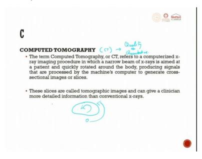
CT or computer tomography, this is exhaustively used for qualitative parameter and quantitative parameter. So, here what happens is, it is a non-destructive way. So, refers to a computerized X ray image procedure in which a narrow beam of X ray is aimed at a patient and quickly rotated around the body producing signals that are processed by the machines computer to generate cross section image or slices.
