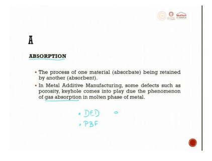
The first important phenomena, which happens in metal additive manufacturing is absorption. The word itself clearly says absorb, absorption the process of one material being retained by another. In metal additive manufacturing some defects such as porosity, keyhole comes into play due to the phenomena of gas absorption in molten phase of metal.
