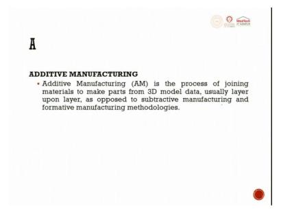
Additive manufacturing- multiple times we have seen that definition additive manufacturing is the process of joining materials to make parts from 3D model data usually layer upon layer as opposed to subtractive manufacturing and formative manufacturing methodology.
