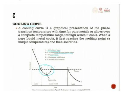
When we are trying to talk about metals or ceramics, when you try to heat the metal, the most important thing which comes into existence is the cooling curve. A cooling curve is a graphical presentation of the phase transition temperature which is a temperature versus time graph. So, when you try to hit or melt a powder, the curve with respect to temperature follows like this. So, A B is a cooling of liquid.
