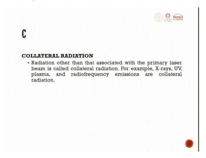
Collateral radiation- radiation other than the associated with the primary laser beam is called as collateral radiation. For example, X- ray, UV, plasma, and radiofrequency emissions are collateral radiations which are created in a small extent while the process happens.
