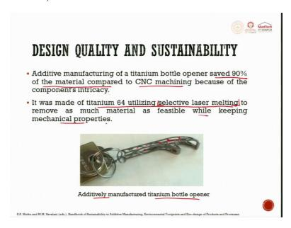
Now additive manufacturing of a titanium bottle opener as an example here, if you could see. This saved 90 percent of the material compared to a CNC machining because the material which was there in the subtractive manufacturing, so, there is no material in between just having the proper optimized material only wherever the stress concentration is more, it is designed accordingly.
