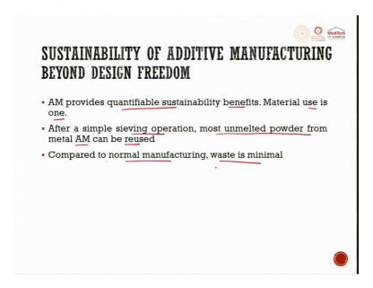
Sustainability of additive manufacturing beyond design freedom. what do we have? It provides quantifiable sustainable benefits. Material use is one of those only. Other than this, we have simple sieving operation, that is most unmelted powder from the additive manufacturing can be reused. Compared to normal manufacturing, the waste is minimal. So, there is a general flow for the design of additive manufacturing.
