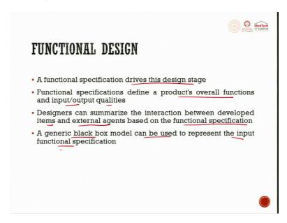
Now, next step in this is how does this derive the design stage? A functional specification drives this design stage. The function specifications define a product's overall functions and input and output qualities. The designers can summarize the interaction between the developed items and external agents based upon the functional specification. When I say functional specification like for example, this bottle opener, the function was just to open the bottle, number one primary function.
