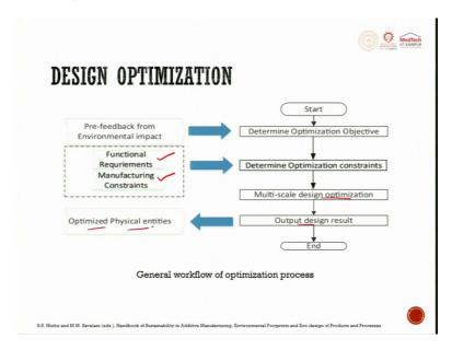
In the design optimization, the pre-feedback from environment is taken that acts as an impact input. This is how the workflow of optimization goes. So, this goes as input and that determines the optimization objective in the flowchart.
