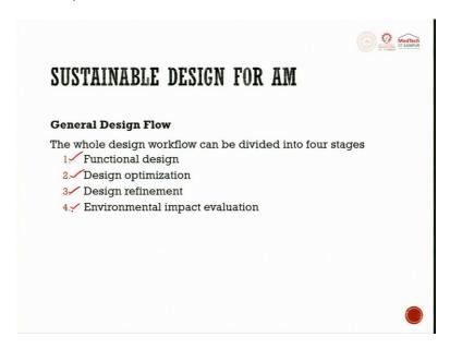
The whole design workflow can be divided into four major stages that is a functional stage, design optimization, design refinement, environmental impact evaluation.
