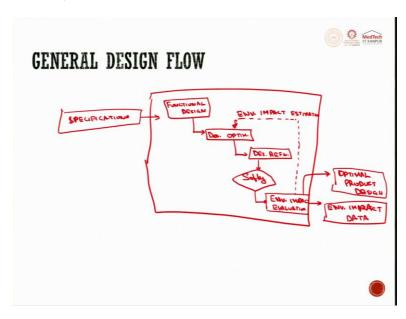
If I try to see these stages, so how does it go? So, we have the specifications as the input. This is a general flow or we have designed requirements or specifications, these goals as an input to my manufacturing system or my design system. So, where functional design is there and we have physical entities, which enter to the design optimization, so which further provides that design refinement and then we have the diamond box, which says that the safety of all functions is put or not.
