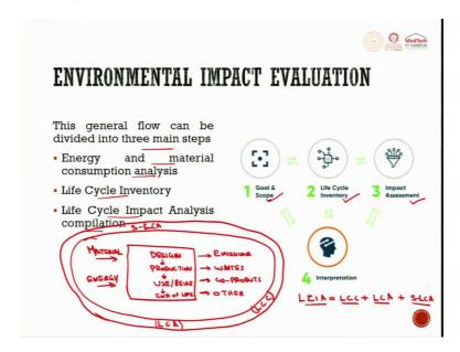
In the environmental impact evaluation, the general flow that can be divided into three main steps as it is given here, the energy and material consumption analysis, the life cycle inventory, a lifecycle impact analysis compilation. For that we need to identify our goal and scope of the analysis or the assessment that we are going to do, we need to understand the lifecycle inventory of the component or the product under study.
