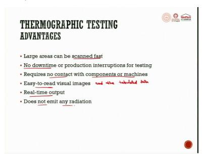
So, there are certain advantages of this. For example, large areas can be scanned fast. No downtime or production interruptions for testing. Directly, we can get the thermal images. Also, the temperature along with the images can be gotten in the directly quantitative form. So, we can get the quantitative data, temperature is varying from time A to time B, for example from 0 to 60 seconds, the temperature has risen from  $10^0$  to  $30^0$ , if we are heating something very rapidly or so.
