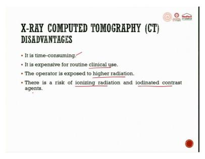
The disadvantages would be, it is time consuming because multiple images are to be taken and the body or the component is to be rotated sometimes. It is expensive for routine clinical use. The operator is exposed to higher radiation. There is a risk of ionizing radiation and the iodinated contrast agents. Whatever it is, the X-ray CT technology provides higher resolution. That is, it can distinguish the tissue having differences of less than 1 % of their physical densities.
