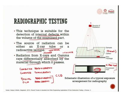
So, there are certain non-contact methods. The first one is radiographic testing. As the name itself says, it sends the radio signals, that is, it sends the sonar signals and its tries to see what the defect is, what is the flaw in the part under inspection. So, there is a radiation source, so radiography involves a technique that is suitable for the detection of internal defects within the volume of the examined part.
