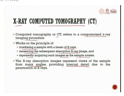
Next, and the last technique in this lecture series on non-destructive testing to be discussed is X-ray computed tomography. Computed tomography or CT refers to computerized X-ray imaging procedure. It works on the principal, that is irradiating a sample with a beam of X-rays,
