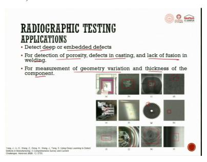
Now, its applications are overwhelming. It detects deep or embedded defects, for detection of porosity, defects in casting and lack of fusion in welding, for measurement of geometric variation and thickness of the component. It has multiple applications. You can see different applications for the radiographic test which are given. The surface that is small, pores here. The small cracks here, the broken gear, so many applications are here.
