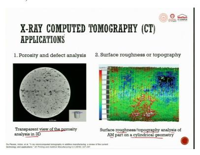
So, it has certain advantages. That is, the quality of the images that we get is useful in having the feel of the defect in the color form, in the shape. The porosity and effect analysis, you can see transparent view of the porosity, analysis in a 3D form. Then surface roughness topography analysis of an additive manufactured part on a cylindrical geometry using the topography and using the X-ray computed tomography.
