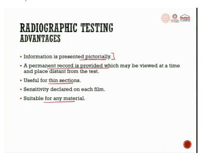
The advantages of this are the information is presented pictorially. The visual inspection then comes into play after this to understand the picture of the image. The permanent record is provided which may be viewed at a time and placed distant from the test. It is useful for thin sections. So, sensitivity is declared on each film. It is suitable for any material irrespective of ferromagnetic, paramagnetic, or so, or non-ferromagnetic, plastic. It can be applied to any material.
