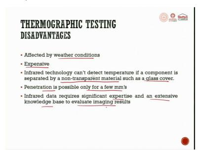
The demerits would be, it is affected by weather conditions or environmental conditions, the cameras are expensive. A simple thermal camera that is having a range up to 700<sup>0</sup>, that we have gotten here in IIT Kanpur is costing 3,60,000 rupees. So, it is not very economical technology to be used by everyone.
