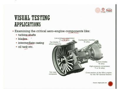
Also examining the critical aero-engine components, for example, turbine shafts, blades, intermediate casing, oil tank, low pressure compressor, titanium alloy, so this all, from outside, whatever we could look. The intermediate casing, the oil tank, turbine, and this is generally visually inspected.
