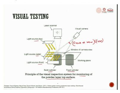
So, this is a visual inspection system, that has camera and laser scanner as well to identify, to monitor the powder layer of the top surface in metal additive manufacturing. So, it is a visual camera. This is the window of the camera, or I would say, the Field of View the FoV, it is also called FoV of the camera.
