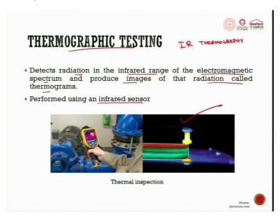
Next is the thermographic testing. Thermograph testing is having plethora of application. For example, in machine tool cutting itself, whenever the temperature is to be measured, temperature measurement instruments or temperature sensors are available from -25° to 2000°, and the temperatures could be measured to identify the kinds of the temperature change, how drastically the temperature is changing.
