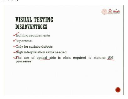
Disadvantages are, I showed you illumination or the lighting requirements that are always there. It is always a superficial test, which means, just by looking at surface, the information we are trying to put on an inference is based upon the experience only. Which is at times correct, based upon the package of experience of the engineers working upon.
