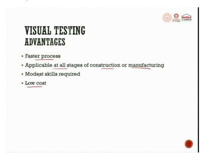
Advantages are, it is a faster process, it is applicable to all the stages of construction or manufacturing, modest skills are required, that is, very few skills are required, at least to have the retrieval information. So, it is a faster process. It does not require any sophisticated apparatus, and it is very inexpensive method, low cost.
