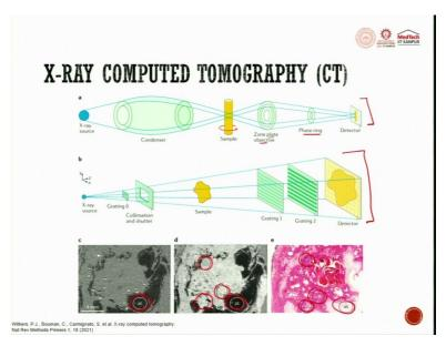
So, this is a schematic here. X-ray source is there, there is a condenser, and this is a sample. Sample is rotating from each side. The images are being captured by the detector, which lets the image of the ray to pass through a zone plate, that is, the objective, then a phase ring.
