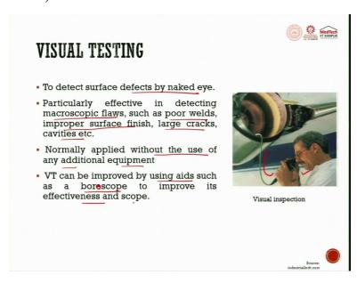
Next is visual testing. As you can see here, just by visualizing, an experienced operator, an experienced engineer could test that how is my material behaving, how is my system behaving.
