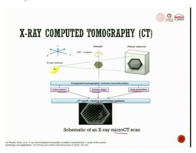
So, this is again a schematic of an X-ray micro-CT scan, that has a planar detector. So, it is a tube control sample stage and data acquisition that helps us to get the CT result that is viewed and further analyzed.
