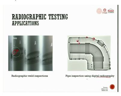
One of the other applications which is given here is the porosity in the weld inspections. You can see the film has recorded the area which are darker, which determines, or which reflects the
