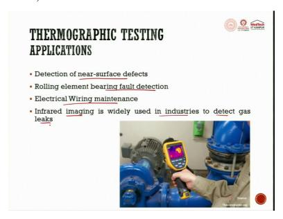
The applications of thermographic techniques in testing are, it detects the near-surface defects, the rolling element bearing fault detection could be taken using the thermal cameras. The electrical wiring maintenance, wherever the connections are weak, the wires would heat because the current is passing through, and there is a thermal flux that is coming out of it or leaking out of it. Infrared Imaging is widely used in industry to detect gas leaks as well.
