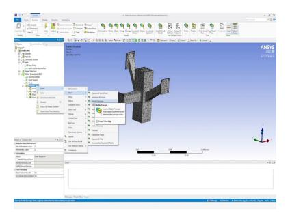
So, we can select from material assignment, 17 4 pH stainless steel. Based upon this material, we will try to see how the stress concentration flows. So, now we can come to mesh. I will now generate a mesh over it. I will just click mesh here. To have a structural analysis, this is one of the most important steps, to create mesh.
