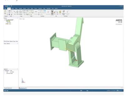
And this model is ready now for 3D printing. So, this is how we have the topology optimization conducted on a very simple kind of structure. We developed a CAD model, we try to develop the mesh using Ansys software. We tried to add the static deformation model out of it. Then, we transfer that model for topology optimization, tried to have the material only wherever is required, smoothen that.
