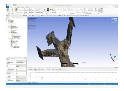
So, this is how it shows that the material could be there, or the component could be there. So, wherever the material is not required, it has removed the material from that part. So, that was the base model. And this one is optimized based upon the density. So, it can be reduced around 50% of the material.
