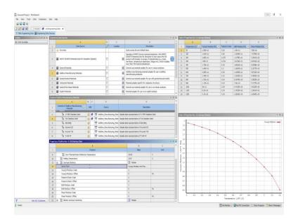
First, we come to the engineering data. To add the material here. In our library here, we can have different property, physical properties, linear, elastic, hyper elastic, then plasticity, creep life. Different kinds of the toolboxes are here from which we can put the features, the parameters that we are going to use or that we are going to fix as a range or as a fixed or constant.
