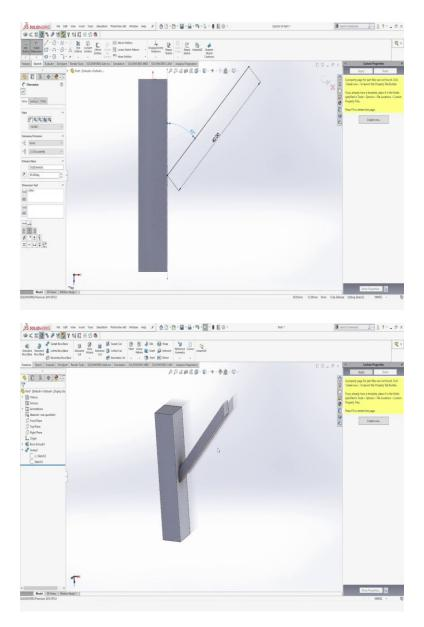
So, I can just select a surface or sketch. I just selected the surface, then I selected a sketch. I just drew an axis line here. So, the different corners are set so that this axis comes to the midpoint. So, then we have snaps here. There are multiple ways to put snap here, that what the points are to be snapped, point snap, center snap, midpoint snap, quadrant snap, intersection snap, near a snap, grid snap.
