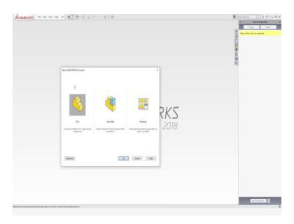
This is Solidworks 2018. So, it contains number of modules. Designing, simulation for different purposes. So, this is the main page of Solidworks when we open it. If we select, there are options which come. We can open a new part, a drawing or assembly. So, these can be opened with 2D representation, that is, the drawing, with 3D representation could be taken in part and assembly.
