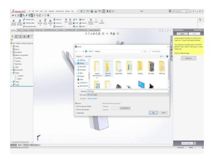
Now, if we check this, make it normal, and on this perpendicular surface, or an adjacent surface to them, another arm would be drawn, first while drawing the center line, then we can make a circular rod or rectangular load based on our choice. So, for a circular arm, we can specify the radius of the arm. That means, the radius is 2.5. So, it will make the diameter as 5 mm.
