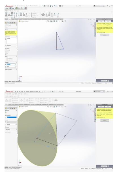
So, also, revolve command is also there, another example. So, in a 30 minute lecture, we cannot explain the complete software features. So, just to give the basic information, I am just trying to make, a triangle is made. This triangle could be rotated along its
