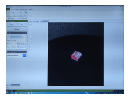
So, we can see this in the screen itself that it is coincided closer. Now we have come close to the computer screen and we have seen that the frames which are being produced, the fringes of the frames which are being produced or being put on the object we could see that, you can see this cross, the intersection point of the cross is the center of the scanner.
