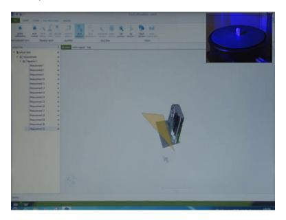
Menu bar we have various tools here in the selection tab, we have lasso tool, lasso tool means we can cut using this tool the non required or unwanted area. So, we should delete the points which are not required otherwise the file size will be so heavy that it will not be easy to handle. So, we select this and try to clip everything using clip tool that is given in the selection tab. So, it is a clearer data.
