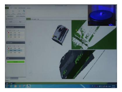
So, now the 3 points are scanned and aligned here so, it takes time. It is the skill of the operator, the one who is scanning that how close, how less time does he or she takes to produce the object closest to the pattern or the final object that is required.
