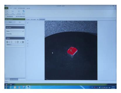
You can see the object on the screen only now, we have position that is to be filled now, we have access control as well in which rotation could be controlled. Rotation we kept at 00 only the position is to be set. So, to have minimum 36 readings we can have 360/10 that each 10 degree it would keep on recording the data.
