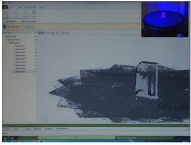
So, the scanning is happening now. The scanner is started it has started to stack scanning now the object, so it is trying to connect the frames, the previous one and they are recent one, it is trying it keeps on, keeps on trying to align and capture the data simultaneously.
