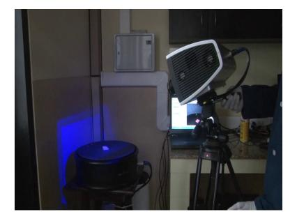
To capture the object correctly, it must be kept as close to center of the rotary table and also the two dots which is the focus of the light coming from the scanning camera is to be adjusted close to the center.
