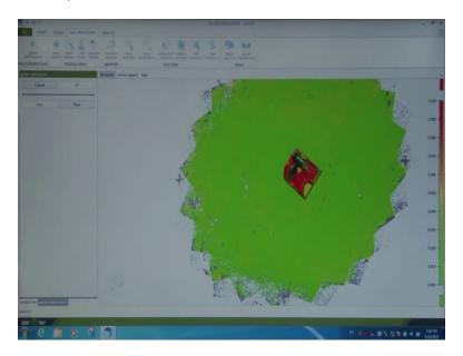
Now, the extra features which are there again, we can move using the lasso tool as we did it before so, we go to the bar data processing bar, we have global optimization, the ribbon here and again try to do the global optimization. So, the green boundary here shows the object is in the same orientation as of the scanner.
