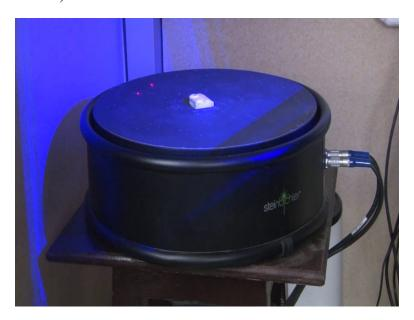
Now, we have the second major part of the 3D scanner equipment setup which is the rotary table this rotary table is controlled by the controller box, this is also a Steinbichler controller box. So, the data that we put or that we get from here is obtained in real frame.
