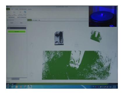
Now, in this case, we have changed the orientation of the object because in the previous scan there are certain portions which were not clear. So, in the second orientation, we have started the scanning again, it is now showing successful, successful means the previous scan and the recent scan that has been taken both orientations are matching.
