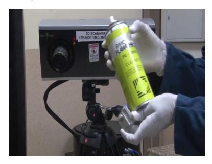
Now, if time sometimes the object is to be cleaned, then PC 5021B cleaner is used so that we remove all the dust particles and object to be scanned is completely clean. Sometimes the object is also shiny like this, aluminium is shiny so it does not capture the light and the data is not captured properly.
