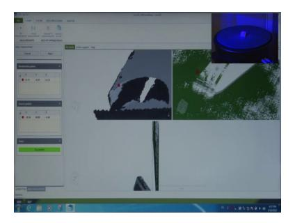
See the two points are matched. So, first we need to do the manual alignment as close as possible. we just click two points here which we think are closer. So, to select the points generally the edges the corners are taken, the two points you can see red point on the scan that was not previously and the current scan. I will product scan A and scan B through the other line.
