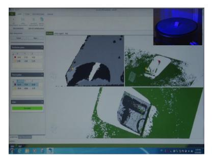
We can also see whether how close the object is to the previous scan. We can see it is showing close almost occluded. So, let us take another point third point so, to put the third point is to pick a place. We can pick at this surface here, at this surface at around this place, the result is there in the lower window frame that did not match much. So, another point is taken at a different location.
