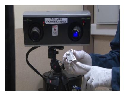
This is the object that we are going to scan today this is also known as the 3D scanning specimen object. This object you can see it has curvature, the straight surfaces which is priming pocket slots, dome, cavity dome, corners, fillet radius so we will try to use this object to scan the different kinds of the intensities of the scanning process.
