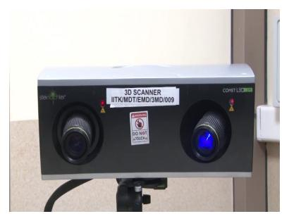
So, this is a 3D scanner that is kept at med tech facility IIT, Kanpur. You can see the sticker that is an ISO 13485 compliant sticker IITK MDT EMD 3 MD 009. Whatever we scan through this object, we get the real data of that object.
