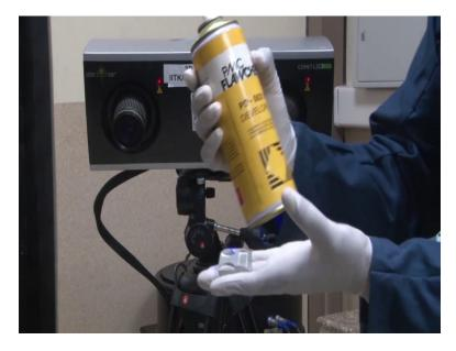
So, we use the developer which is PD visor 31B which is a white colored chalk coated developer, we spray it over the object so that the refractive index does not come into play.
