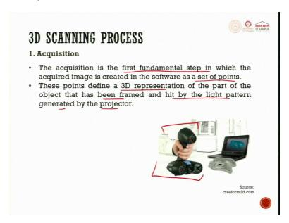
The acquisition is the first fundamental step in which we acquire the image that is created in the software as a set of point, it is in the acquisition process only when we need it to the scanner, this is a handheld 3D scanner. We need this equipment only for the data acquisition, once the acquisition is done, then everything happens on the software in your computer.
