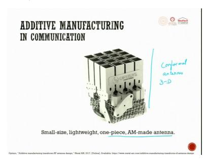
So, next in terms of communication, it is a small size lightweight one-piece additive manufactured antenna. This is exhaustively used today, there are conformal antennas which are three dimensional is being made. So, earlier they used to make it planar, now, they are making it three dimensional.
