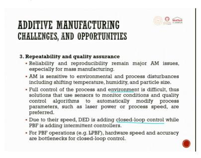
So, repeatability and reliability. We are nowadays looking for closed loop control system. In the closed loop control system we are looking at environmental conditions like temperature around and the dust around. (Refer Slide Time: 20:16)
