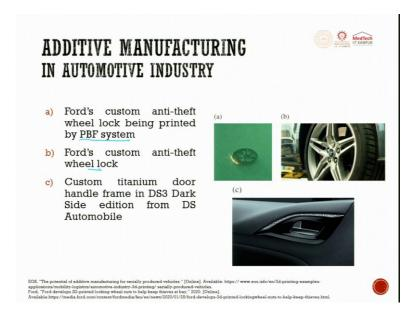
Next, when we look at the automotive, such complex small thin features can be printed. So, Ford customized anti-theft V lock was being printed by powder bed fusion system. You can also have customized wheel locks. So, if you have to customize, you have to use automotive metal additive manufacturing, then custom titanium door handle frame with DS3 dark side edition from DS Automotive.
