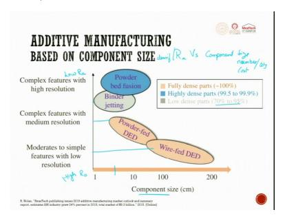
So, when we look at the additive manufacturing based on component size, if you look at this side, you have powder bed fusion. So, in the y axis, you will have complex features with high resolution and at the bottom you have moderate to simple features with low resolution, resolution here we talk about so I can convert in terms of Ra, this is poor Ra or low Ra, this is good Ra or high Ra good. So, I will convert it into high Ra value and I will make this into low Ra value.
