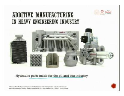
Additive manufacturing in heavy engineering industry, several hydraulic valves are getting manufactured in one go. So, you will have so many channels which are getting integrated.
