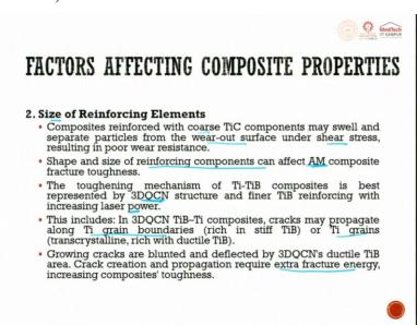
When we talk about the size of reinforcing element, composite reinforcing with coarser TiC components may swell and separate particles from the wear out surface under shear. So, pull out will happen very easily. So, under shear stress it will come out resulting in poor wear resistance. So, we will always look for a small finer TiC component.
