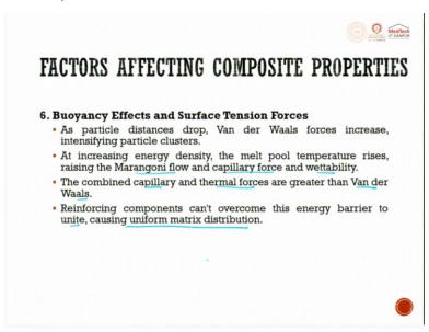
As the particle distance drops, Van der Waals forces increase, intensifying particle clustering. At increasing energy density, the melt pool temperature rises, rising the Marangoni flow and the capillary force and wettability. The combined capillary and thermal forces are greater than the Van der Waals force. Why is that important? You can go back here. As the particle distance drop the Van der Waals force increases, intensifying particle clustering.
