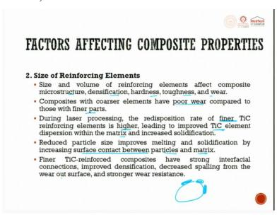
Next is size of reinforcing element, size and volume of reinforcing element affects the microstructure densification, hardness, toughness, and wear. If the size between the metal powder and the reinforcing are in some ratio, if the matrix powder size is large and the reinforcing is small, then it becomes a little easy for getting the required achievement.
