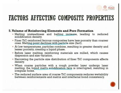
The melting unsteadiness and balling increases leading to reduced solidification density. What is balling? We discussed when we talked about the various parameters. Finer TiC reinforced ferrous composite have lesser porosity than coarser ones, melting point declines with particle size. All at low temperature particles combined resulting in greater density and lesser porosity creating a liquid phase. Because of liquid phase it can flow, it can get consolidated.
