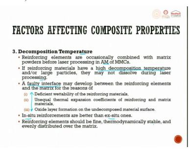
The third point of discussion is going to be composite temperature. Composite temperature or decomposition temperature. The reinforcing elements are occasionally combined with matric powder before laser processing in AM process. If reinforcing material have a high decomposition temperature and a large particle, they may not dissolve during the laser processing. If they are high decomposition temperature, then they will not dissolve during the laser processing.
