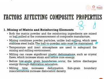
When we talk about mixing of the matrix and reinforcing agents, both the metal powder and the reinforcing ingredients are mixed, or ball milled at the commencement of the composite manufacturing. The mixing combines powder particle unlike ball mill which uses stainless steel balls. The ball to powder ratio must be maintained, that is an important factor which is called as ball to powder ratio.
