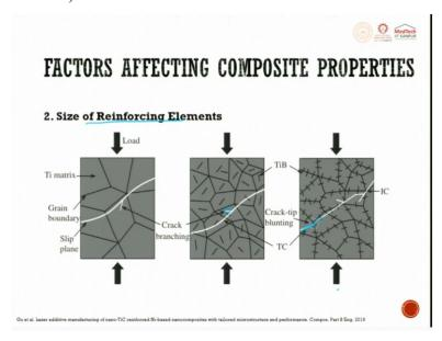
So, this is what it is a load there. So, you have Ti matrix. These are all the grain boundaries, and this is a slip plane which happens. So, you can see here is the crack branching. So, right these are crack branches which are there. So, in the same way when I have a load with TiB and TC so, TiB is this. So, you have TiB which is there and then you see the crack that is going the branching whatever happens and how does it go. So, these are all crack branching.
