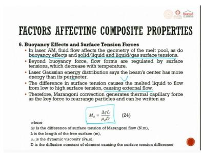
When we discuss about buoyancy effects and surface tension in laser additive manufacturing fluid flow affects the geometry of the melt pool and do buoyancy effects and solid liquid, liquid gas surface tension. So, this is important. There is a buoyancy effect. Beyond buoyancy force, flow forms are regulated by surface tension, which decrease with temperature.
