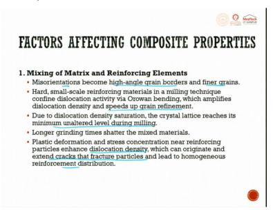
Misorientation become high angle grain border and finer grains. Misorientation is also an important parameter, when it tries to be milled for a longer time, it undergoes misorientation. Hard, small scale reinforcing material in a milling technique confined dislocation activities via Orowan bending, which amplifies dislocation density and speeds up the grain refinement.
