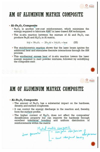
When we try to mix iron oxide in aluminum, so, we can also make such composites. Fe<sub>2</sub>O<sub>3</sub> is another low-cost reinforcement which minimizes the energy required to fabricate AMC in laser based additive manufacturing techniques. The in-situ reaction, whatever it is, so that
