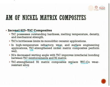
Now we will move on to nickel-based alloys. Nickel based alloys are Inconel 625 reinforced with TiC. TiC possesses outstanding hardness, melting temperature, density and mechanical strength. TiCs brittleness, limits its monolithic ceramic application. In high temperature, refractory wear and surface energy applications, TiC strengthened nickel matrix composites perform very well.
