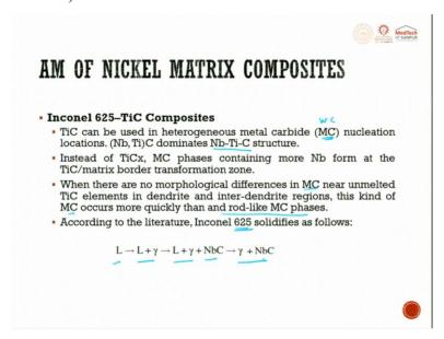
When we look at the entire thing TiC can be used in heterogeneous metal carbide, MC that can be WC, TiC, TaC, SiC, nucleation location Nb TiC dominates Nb TiC structure. Instead of TiC<sub>x</sub>, MC phase containing more niobium form at the TiC matrix border transformation zone. When there are no morphological differences in metal carbide, nearly unmelted TiC elements in dendrite and inter dendrite region, this kind of MC occurs most quickly than the rod like structure in this.
