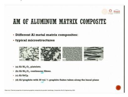
Next is Nickel, wherever it is high temperature and where they do not bother much about density, they go for nickel matrix composites. When we talk about metal matrix composites where aluminum is the matrix so, we see various types of microstructures. We see here
