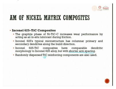
The graphite phase of Ni TiC C, we are bringing the C through the graphite phase. Increases wear performance by acting as an insitu lubricating between friction or during friction. Inconel 625's typical microstructure has columnar primary and secondary dendrite along the build direction.
