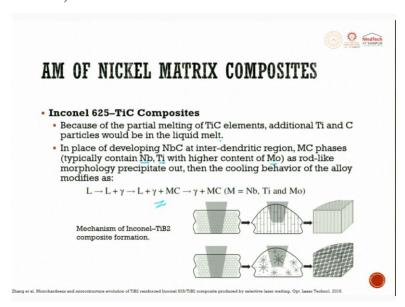
Inconel 625 TiC composite, because of the practical partial melting of TiC element, additional Ti and C particles would be in the liquid melt. In place of developing NbC at inter inter dendritic region, metal carbide phase containing NbTi and higher contents of Mo has rod like morphology precipitates out then the cooling behavior of the alloy is written like this.
