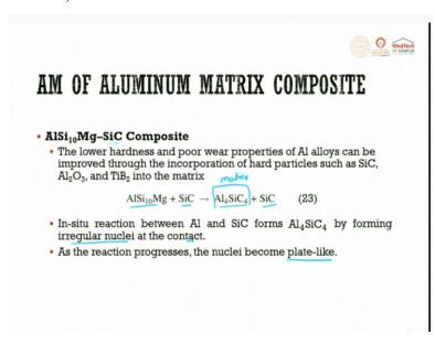
AlSi<sub>10</sub> Mg with SiC composite, lower the hardness, poor wear properties of aluminum alloy can be improved through the incorporation of hard particles such as Si<sub>3</sub>, SiC, Al<sub>2</sub>O<sub>3</sub> and TiB<sub>2</sub> into the matrix.
