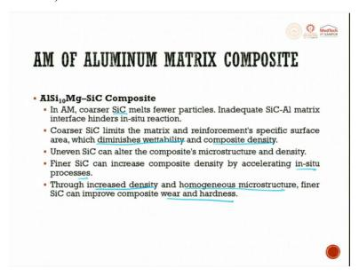
In AM, coarser SiC melts fewer particles. Inadequate SiC-Al matrix interface hinders the insitu reaction. Coarse SiC limits the matrix and reinforcement specific surface areas which diminishes wettability and composite density. So, diminishes wettability and composite density. Uneven SiC can alter the composite microstructure and density.
