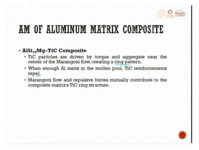
TiC particles are driven by torque and aggregate near the center of the Marangoni flow creating a ring pattern. So, this is the same thing when you see, when iron also TiC ring pattern, the same thing. Al melts in the molten pool, TiC reinforcement repels them. Marangoni flow and repulsive forces mutually contributes to the composite matrix TiC ring structure.
