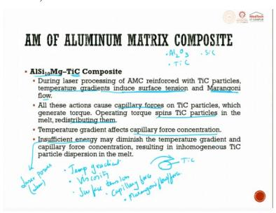
Now, AlSi Mg with TiC, we saw with alumina. Then now we are going to see with TiC. We also saw with SiC, the previous one was SiC. During laser processing of additive manufacturing composite reinforcement with TiC particles temperature gradient induced surface tension and Marangoni flow is very important.
