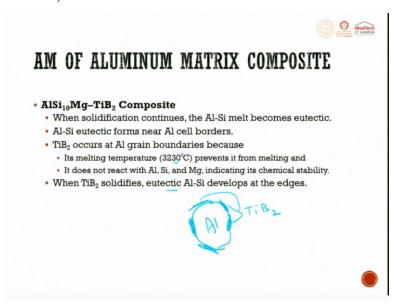
When the solidification continues, the Al-Si melt becomes eutectic. Al-Si eutectic forms near Al cell boundaries. TiB<sub>2</sub> occurs at Al grain boundaries because Al grain boundary you will
