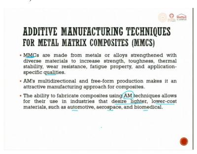
So, MMCs are made from metal or alloys strengthened with diverse material to increase strength, toughness, thermal stability, wear resistance, fatigue property and application specific qualities. That is why we try to go for metal matrix composites. Additive manufacturing multi directional and freeform production makes it an attractive manufacturing approach for composites.
