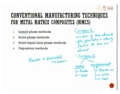
When we talk about conventional manufacturing techniques for metal matrix composite, it can be through liquid phase method, solid phase method or it can be a combination of solid liquid phase method, the last thing can be deposition. So, these are the four predominant techniques, the process names can be there, but the basics of the process falls in this four only.
