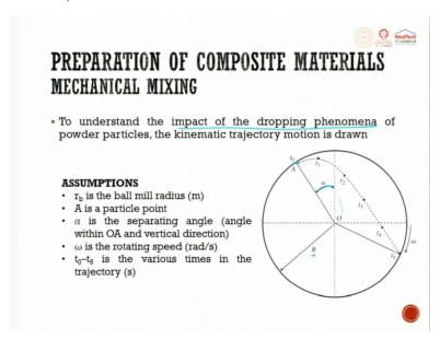
To understand the impact of the dropping phenomena of a powder particle, the kinematic trajectory motion is drawn here. You can see this is what is the kinematic trajectory motion,  $r_b$  is the ball mill radius, A is a particle point and  $\alpha$  is the separating angle between OA and the vertical direction this is the angle, this is the point. So,  $\alpha$  is a point here.
