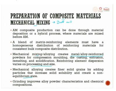
When we are discussing about preparation of composite material, we will always use mechanical mixing method. This mechanical mixing method is using a ball mill. AM composite production can be done through material deposition or a hybrid process. Whereas materials are mixed before AM. A blend of matrix reinforcing element must have a homogeneous distribution of reinforcing material for consistent bulk composite distribution.
