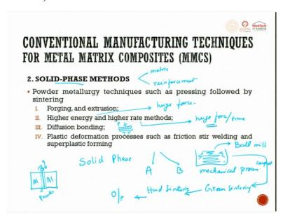
Next let us move to solid phase methods. In solid phase methods, what we have is we have a powder metallurgy technique such as pressing, followed by sintering. Solid, so that means to say both the material, matrix and the reinforcement are made out of or are powders. And they start with these two powders and then they go undergo a sintering cycle. So, the powder metallurgy technique such as pressing, followed by sintering is very, very common.
