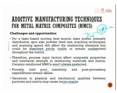
For laser based moving heat source, because the laser will be moving along the bed, moving heat source, laser power, intensity distribution, spot size, powder feed rate, scanning techniques and scanning speeds will affect the reinforcing element that could be dissolved partially, totally or remain undissolved throughout the matrix.
