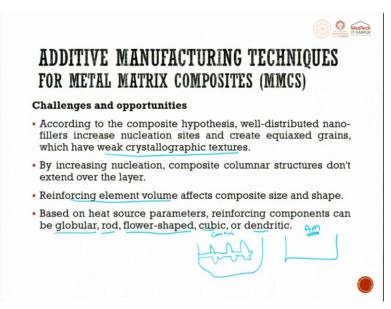
So, the challenges and opportunities according to the composite hypothesis, well distributed nano fillers, increase nucleation sites and create equiaxed grains which has weak crystallographic textures. This is a biggest challenge, which we have to make sure. So, well distributed nanofiller increase nucleation sites yes, and creates equiaxed grains that is also yes, which have weak crystallographic textures.
