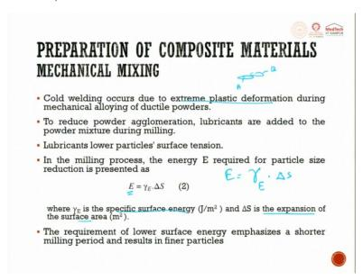
The other one is cold welding. In cold welding occurs due to extreme plastic deformation during mechanical alloying of ductile powders. What is cold welding? So, cold welding is you have one powder, you have another powder so, now, when there is a hammering happening, so, extreme plastic deformation happens and these two fellows join. So, this is A, this is B, metal powder.
