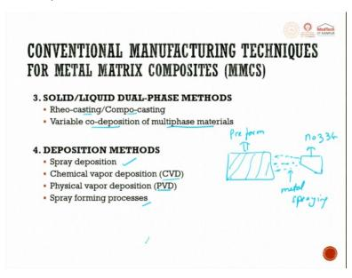
The next one is called a solid liquid dual phase casting. This is Rheo casting or combo casting, here you take it to a mushy state and then you try to disperse it, the liquid will be
