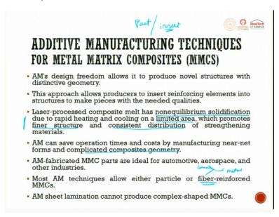
So, additive manufactures design freedom allows it to produce novel structures with distinctive geometry. This approach allows producer to insert reinforcing element into structures to make pieces with the needed qualities. Laser processed composite melt has non-equilibrium, we have already covered equilibrium and non-equilibrium solidification due to rapid heating and cooling on a limited area which promotes finer structure and consistent distribution of strengthening material.
