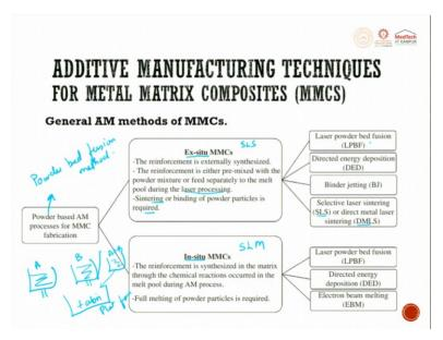
So, when we look into general additive manufacturing methods of metal matrix composite, you can start with a powder based additive manufacturing. So, what is powder based, you are talking about powder bed fusion method. So, here you have a container filled with A powder, container filled with B powder, you can try to mix on the platform where fabrication. This is a fabricating platform. So, fabricating platform, so you can have a mixture of this and this getting it done.
