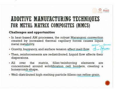
In heat based additive manufacturing processes, the robust Marangoni convection created by increased thermal capillary forces causes liquid metal instability. So, what causes instability, it is a robust Marangoni convection. It is also a good idea to go back and refer to what is Marangoni convection used in casting as well as in metal matrix composite, you please go through the literature you will understand more.
