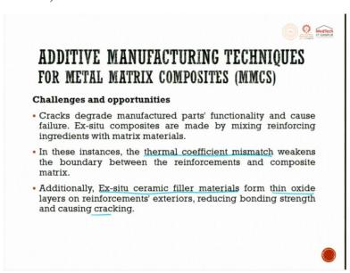
The cracks, degrade manufactured parts functionality and cost failure. Ex situ composites are made by mixing reinforcing ingredients with the matrix composite. In these instances, the thermal coefficient mismatch, this is very important. That is what I said, thermal property problems. The thermal coefficient mismatch weakens the boundary between the reinforcement and the composite matrix.
