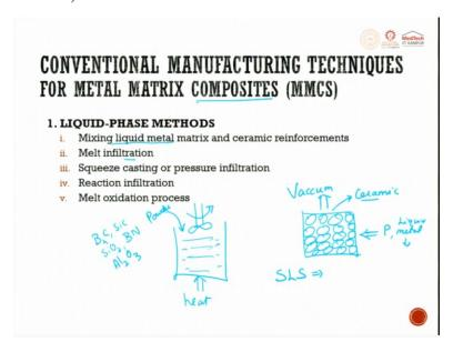
When we talk about liquid phase method, the mixing liquid metal matrix and ceramic reinforcement happens here. So, we try to mix liquid metals so liquid metals, it is not at room temperature, it happens at very high temperatures, these two are mixed or two a liquid metal matrix, whatever is there, aluminum alloy, you try to mix up a reinforcing agent. So that is what is called as liquid phase.
