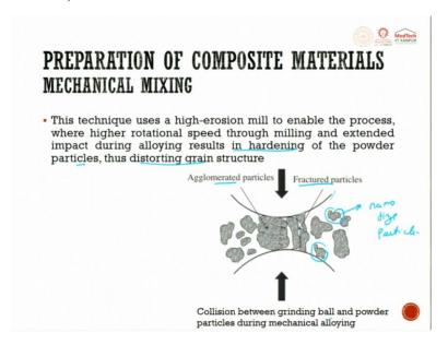
So, this technique uses a high erosion mill. This is collision between the grinding ball and the powder particle during mechanical alloying. So, you will have one ball, you have another ball, two balls and they will be rotating and they will be also trying to collide with each other. So, you will have the powder particle which comes in between when it has got maximum strain harden.
