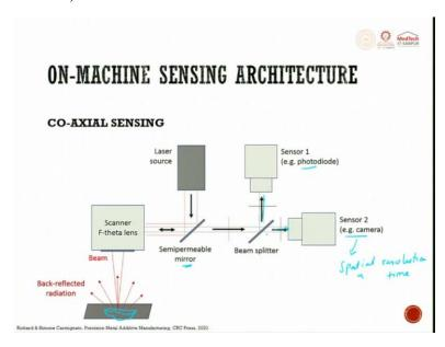
So here it talks about the melt pool. So you can use the f-theta lens. So here you have a semi permeable mirror, so the light hits and the light transfers here. So you have a beam splitter which is there. So the beam splitter splits the light to the camera as well as and then it comes back and then it gets reconstructed. So this is all co-axial.
