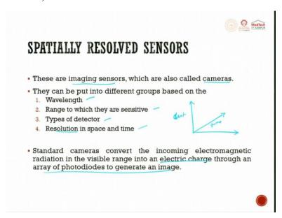
When we are talking about the spatially resolved sensors, these are image sensors which are also called as cameras, they can be put into different groups based on wavelength, range to which they are sensitive, type of detectors, and resolution space and time, resolution and time is seconds, resolution in space is microns. So you can have a resolution in space and time you
