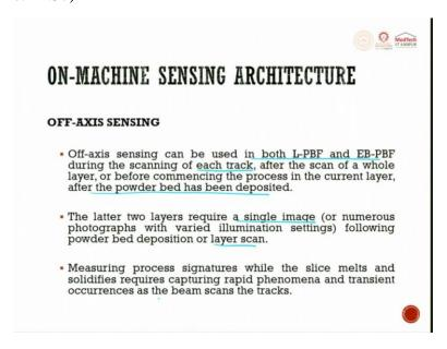
Next let us go to off axial sensing. Off axial sensing can be used in laser powder bed fusion and electron beam powder bed fusion. During the scanning of each track after the scan of your hole layer or both commencing the process in the current layer after the powder bed has been deposited, it can be used in both this and this scanning of each track after the scanning of a whole layer, so here in the current layer it is done. The latter two layers require a single
