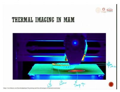
So this is a thermal imaging of MAM when you see it in real use. So this is a laser which goes down and one layer of information and in that one layer of information melting is happening. So you are trying to use a thermal imaging camera and try to take a temperature. So here this is hot this is hotter. And while it is doing it you see here, what is the influence it is also trying to create a temperature high here it is below the bed.
