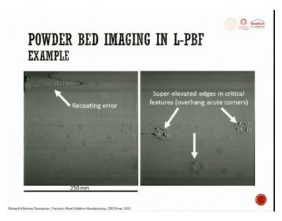
So this is powder bed imaging in laser powder bed fusion, you can see here recoater error, this is a recoater error and you can see here super evaluating yet just in critical features overhang acute corners.
