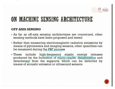
As far as the off axis sensing architecture are concerned, other sensing methods have been proposed and tested rather than measuring an electromagnetic radiation emission by means of pyrometer and image sensing other quantities can be measured during the powder bed fusion process. This includes high frequency elastic energy release produced by the formation of micro cracks, delamination and detachment from the support.
