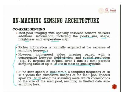
When we talk about this co axial sensing melt pool imaging with spatially resolved the sensor delivers additional information including pool size, pool shape, brightness and temperature mapping. Richer information is normally acquired at the expense of sampling frequency. Moment you have a higher sampling frequency you have lot of information a lot of information means lot of data, this data has to be processed so that is where is that difficulty.
