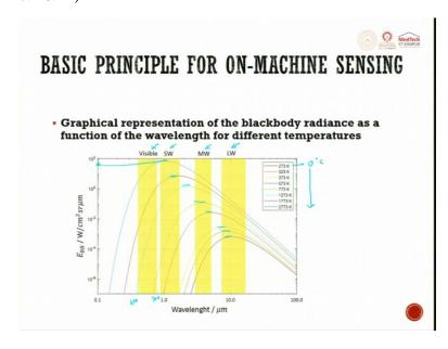
The graphical representation of a blackbody radiance as a function of the wavelength for different temperatures are already plotted and it is kept. So, now, you can see here at 0 degrees Celsius, you can keep going down to 773 Kelvin. So, you can see here, this is the wavelength and these are all the emissivity you can have.
