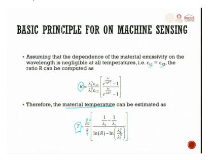
So, assuming that dependency of the material emissivity on the wavelength is negligible at all temperatures, that means to say,  $\varepsilon_{\lambda 1} = \varepsilon_{\lambda 2}$ . Epsilon lambda 1 is the peak for the same material, epsilon lambda 2 is the second peak for the same material. The ratio R can be computed easily. Therefore, the material temperature can be estimated by this formula T is:
