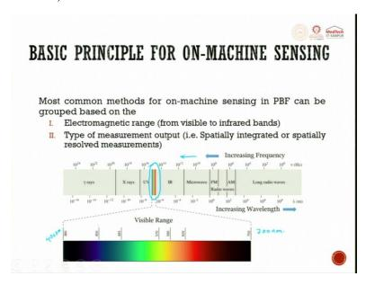
So, principles for online machine sensing, we will be trying to use this visual range. Most common methods for on-machines sensing of powder bed fusion can be grouped based on electromagnetic range from visible to infrared band. Type of measurement output can be spatially integrated or spatially resolved measurement can be done. So, we predominantly work on sensors, which work from 400 nanometer range to 700 nanometer range.
