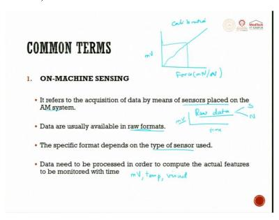
So, on-machine sensing, it refers to acquisition of data by means of sensors placed in the AM system. The data are usually available in the raw format. What I mean here raw format is, suppose you are trying to measure the force, you will always get the output with terms of milli voltage with respect to time. So, now, this is the raw data. From this raw data, you
