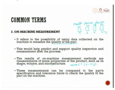
When we try to talk about on-machine measurement, it refers to the possibility of using the data collected on the machine to measure the quality of the part. Finally, what do you want is a quality of the part. You measure all these things. So, we call it as multi sensor fusion, is done where in which you have multiple sensors, S1, S2, S3, S4 you have multiple sensors.
