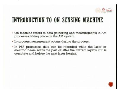
On-machine refers to data gathering and measurements in AM process taking place on the AM system. One is data gathering, the other one is measurement. So, you measure, you gather the data, you process the data and online you take a decision of the data to be done. For example, if there is a thin layer getting selectively sintered using laser beam powder bed fusion method.
