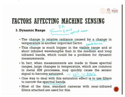
There are lot of dynamic changes which happens during the process. So, rather than measuring a static value, it is always good to measure a dynamic value. So, the dynamic range for every sensor is very very important. So, in the dynamic range, what we do is, we try to measure the change with respect to time.
