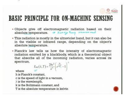
The objects give off electromagnetic radiation based on their absolute temperature. We are trying to hit that IR based sensors. So, objects give off electromagnetic radiation based on their absolute temperature. So, you will try to have your red hot one means a red display will be there, blue is lesser, whatever it is you can try to have, but here whatever you have is going to be an average temperature measurement.
