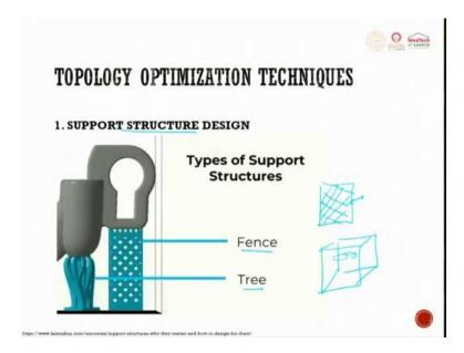
So when we try to see the support structure design, so we have two important things which you should note down, one is called as the fence and the other one is called as a tree type. These two are used for building; there are many more but these two are very common. So, when we try to use fence, it is almost a 2d plane. In a 2d plane you try to have the supports.
