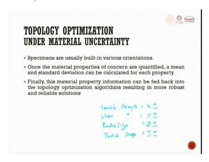
The topology optimization under material uncertainty. The specimens are usually built in various orientation. Once the material properties of concern are quantified, a mean and a standard deviation can be calculated for each property. For example, tensile strength will be X(+/-), so that is what they said, mean and standard deviation. They will say shear strength, Y(+/-), then they will say particle size Z(+/-).
