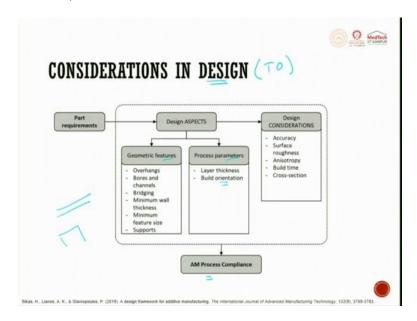
So, some of the considerations in design are the part requirement in the final use, the design aspects and the design consideration. When we talk about design consideration, accuracy, surface roughness anisotropy, build time, cross section; all these things come into existence. When we try to talk about design aspects we have two classifications, one is geometric feature, the other one is process parameter.
