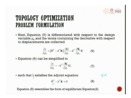
Next, the equation five is differentiated with respect to the design variable rho e and the term containing the derivatives with respect to the displacement are given in this. So, it is a simple math, so I am not getting into it. So, equation six, then you simplify equation six, then you try to put the lambda which satisfies the adjoining equation and then you try to get equation eight resembles the form of an equilibrium equation which we discussed in the stiffness matrix.
