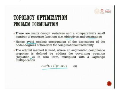
There are many design variables and a comparatively smaller number of response functions, so that is objectives and constraints. Writing the objective equation and the constraint equation is a challenge. If you truly understand the problem only you can easily write, otherwise if you make a wrong choice I am sure you will not land up with the good output what you require.
