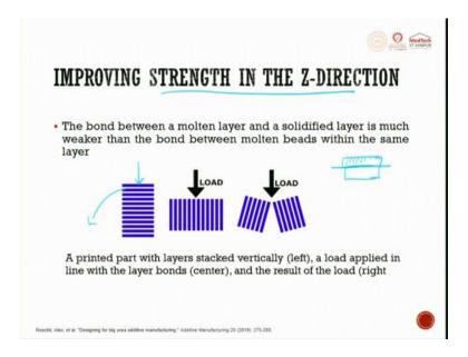
So, improving the strength in the Z direction, this is a direction loading, so the bond between a molten layer and a solidified layer is much weaker than the bond between molten beads within the same layer. I think you should be able to visualize, one layer, second layer, between this layer the bond is very weak as compared to within this layer.
