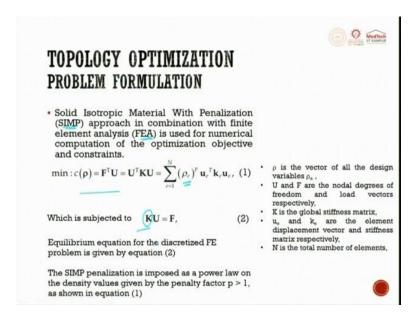
The solid isotropic material with penalization, it is called as a SIMP approach. Several approaches, I have taken one for this example is SIMP - Solid Isotropic Material with Penalization approach in combination with finite element analysis is used for numerical computation of the optimization objective and constraint. This is the objective, this is a constraint which is given.
