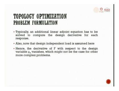
Typically, an additional linear adjoining equation has to be solved to compute the design derivatives for each response. Also, note the design independent load is assumed here. Hence, the derivative of F with respect to the design variable rho e vanishes, e is the element, which might not be the case for other more complex problems.
