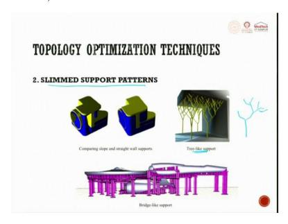
Next moving on to slimmed support patterns. You can see here how is it, when trying to do it comparing slope and straight wall support you are trying to build in slim supports patterns. In slim support patterns what we do is we try to follow a tree like support.
