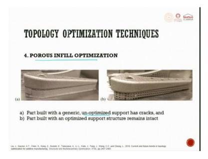
Next one is porous infill optimization. So porous infill optimization, you can see here in a part built with generic un-optimized supports have cracks, these are cracks which are getting build because of the un-optimized support. So, when we try to do porous infill optimization, because of this porous there was a heat exchange and because of this heat exchange the residual stresses are reduced.
