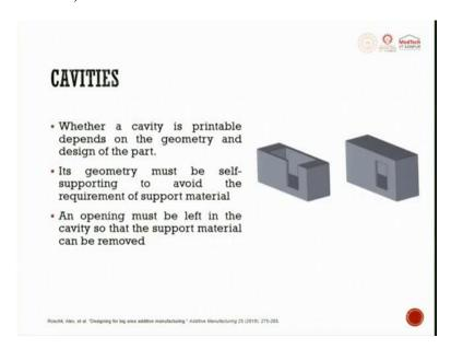
Next are cavities. When a cavity is printable depends on the geometry and the design of the part, when a cavity is to be printed. You cannot have a structure like this, rather than having a structure like this, you make a house, house like structure, this is much more advisable and easy and it is produced to meet out to your dimensional requirement. The geometry must be self-supporting to avoid the requirement of supporting material.
