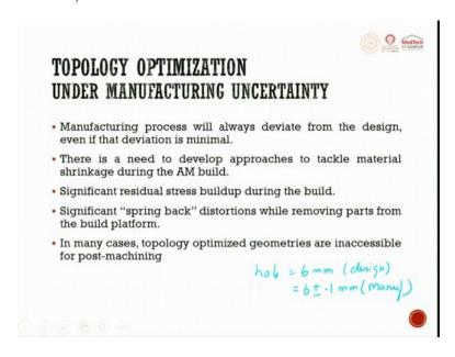
Manufacturing process will always deviate from the design, even if that deviation is minimal, it is accepted. We always try to make a hole of 6 millimeter diameter, but when you manufacture, this is designed, but when you manufacture it always becomes plus or minus 0.1 millimeter. This is manufacturing. Manufacturing process will always deviate from the design, even if that deviation is minimal it is accepted.
