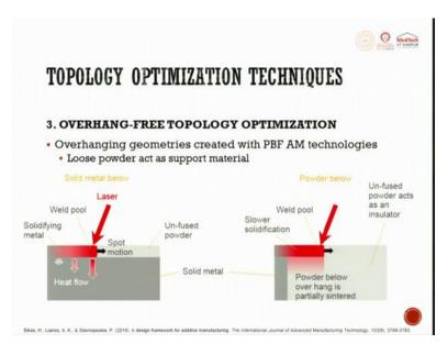
In overhang-free topology optimization the overhanging geometries created with powder bed fusion additive manufacturing technologies looks like this. So, you can see here this is the solidified metal, this is how the laser hits, this is the weld pool or the melt pool, this is the spot moving direction, this is unfused powder, this is where is the heat flow which happens on a solid metal.
