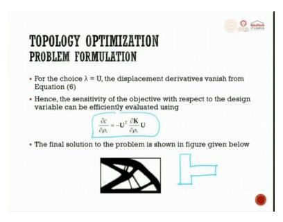
From the choice  $\lambda = U$ , the displacement derivatives vanishes from the equation 6. Hence, the sensitivity of the objective with respect to the design variable can be efficiently evaluated using this equation. So, the final solution to the problem is shown in this figure given below.
