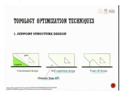
So, this is the support structure design. In support structure design, you have three different types, so the first one is called as unrestrained design. This is the part, this is the support you give and it is completely supporting the object. The other one is called as self-supporting design where in which the support is removed and the object itself while making tries to support itself.
