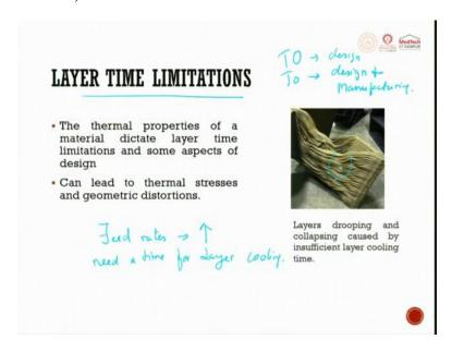
Layer Time Limitation - The thermal properties of a material dictate layer time limitation and some aspects of design. Layers drooping and collapsing caused by insufficient layer cooling time. This is very important. So what I am trying to say is the feed rates, you cannot keep on be increasing, because you need a time for layer cooling, you need a time for layer cooling and so this is also put in the optimization.
