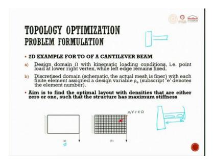
So, topology optimization problem formulation, one simple example I have taken. Let us do that for a 2D example for a topology optimization of a cantilever beam. So, design domain with kinematic loading condition, that is point load at lower vertex, while the left edge remains fixed. Next, discretize domain, the schematic is shown here, discretize the domain, the actual mesh is finer, with each finite element assigned a design variable row subscribing e denotes the element number.
