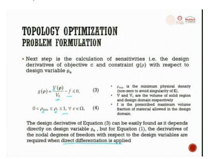
Now once you do that step the next step is the calculation of sensitivity that is the design derivatives of the objective c and the constraint g p with respect to a design variable rho e. So this is equation number three and equation number four, where rho min is the minimum physical density, V and V naught are the volume of the solid regions and design domain respectively, f is the prescribed maximum volume fraction of material allowed in the design domain. So, this is a maximum material.
