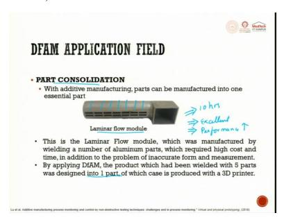
When we talk about additive manufacturing, the biggest advantage comes to it because of part consolidation. With additive manufacturing, parts can be manufactured into one essential part. If you want to make such independent small, small, small slots which is running along the direction then you will be finding it very difficult to machine. But whereas, if you decide the orientation properly, you can try to build these slots running along the direction so nicely.
