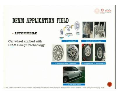
So, the initial design was this. After topology optimization, it was converted into this. The wheel cover or the rim or the spoke, the initial design was this fully made out of metal, then they did lot of topology optimization and finally they generated a beautiful pattern having lot of strength and ductility in the hub.
