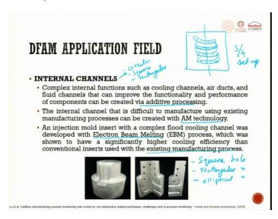
Internal channel forming. Suppose, you have a cylinder and inside the cylinder if you want to have grooves, you have to have grooves for application. So, these grooves, it is very hard for you to continuous grooves, if you, very hard for you to develop without splitting the component.
