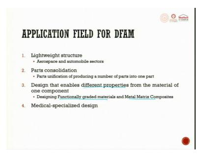
The application fields for DfAM are lightweight structures both in aerospace and in automobile sector it can be used. Then part consolidation, parts unification of producing a number of parts into one part. Part consolidation is a field where DfAM can be used. Design that enables different properties from the material of one component is also possible.
