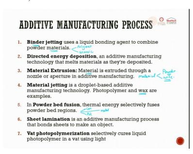
So, binder jetting is use a liquid bonding agent binder, binder means an adhesive. So, you play with a property of the adhesive, so, viscosity is controlled and then you try to drop at the place where you want the material to join, agent to combine the powder.
