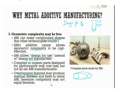
Complex jobs which are shown here can start with a square cross section and end with a circular cross section, if you want to manufacture this it is next to impossible starting with a square ending with a cross section of a circle and trying to have a smooth connect assuming that there is a fluid which is flowing inside.
