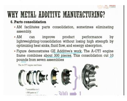
A simple example shown here is GE Additive manufacturing. They reduced 300 parts into 1, for their application because of that, they have cut down 10 pounds from 7 assemblies. So, now, so, if you do any weight reduction, it is going to be a huge saving when you are talking about aero industry.
