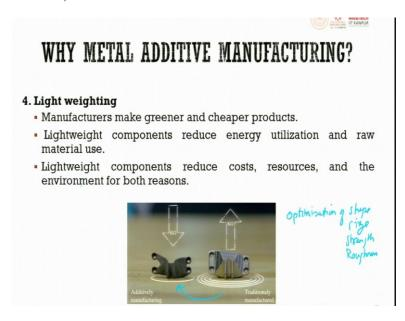
Lightweight, as you see from this, we have reduced to this. So, you can see here that the weight is reduced. This is what is the clamp, which is used. Now, they have made the clamp little more complex such that it can try to take load. So, there are optimization based on shape, size and strength.
