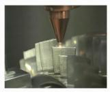
LDED used to rebuild turbine blades
