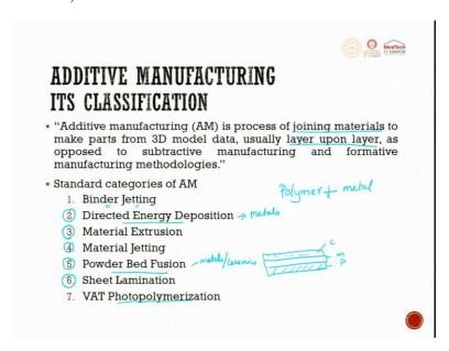
When we talk about the classification, first we will try to see definition for additive manufacturing. Additive manufacturing is a process of joining material. It can be polymer, it can be metal, it can be ceramic, it can be an alloy, it can be a composite. Joining of material to make parts from 3D Model data usually layer upon layer as opposed to subtractive manufacturing and formative manufacturing method.
