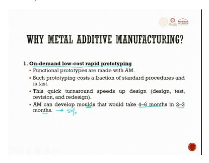
So, on-demand low-cost rapid prototyping functional prototypes are made with additive manufacturing such prototype costs a fraction of standard procedure and is fast this quick turnaround speed up design. Design, testing, revision, redesign all these things can happen. So, on demand low-cost rapid prototyping is possible. So, AM can develop molds that one point of time took 4 to 6 months now, it is getting done in 2 to 3 months.
