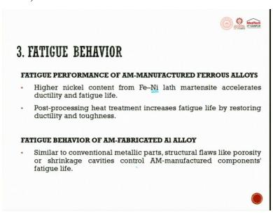
Next, higher nickel content from Fe-Ni lath martensite accelerated ductility and fatigue life, this is nickel because of nickel. The post processing heat treatment increases fatigue life by restoring ductility and toughness, post heat treatment post processing. The fatigue life of AM of aluminium alloy you can see similar to the conventional metallic part structural flaw like porosity or shrinkage cavity controls the additive manufactured part.
