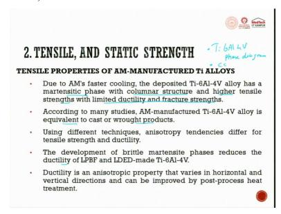
Due to AM's fast cooling the deposited TI-6AL-4V has a martensitic phase with columnar structure and higher tensile strength with limited ductility and fracture strength. All these lecture slides are being extracted from various research papers. So, that is why you see some of the things are abstract, but all these things you will be able to appreciate when you parallelly go through the TI-6AL-4Vphase diagram.
