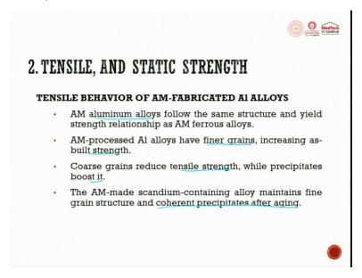
Additive manufacturing. Now, we are trying to talk about aluminium alloys follow the same structure and yield strength relationship as AM ferrous alloys. Almost in the same way whatever response ferrous gives I am not talking about in terms of exact magnitude, but in terms of comparison of ferrous alloy, which is conventional ferrous alloy additive manufacturing the behaviour you will get the same behaviour with respect to aluminium alloy also.
