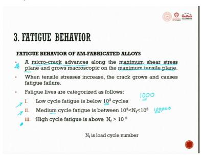
A micro-crack advances along the maximum shear stress plane this is very important micro-crack advances along a maximum shear stress plane and grows macroscopic on a maximum tensile plane very important point to note, micro-cracks advance along maximum shear strength plane shear stress plane and grows macroscopic on the maximum tensile plane. When tensile stresses increase the crack grows and causes fatigue failure.
