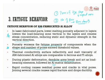
The laser fabricated part lowering melting porosity adjacent to layer lowers the load bearing zone vertical to the layer and creates a stress concentration reducing static and dynamic strength in the
