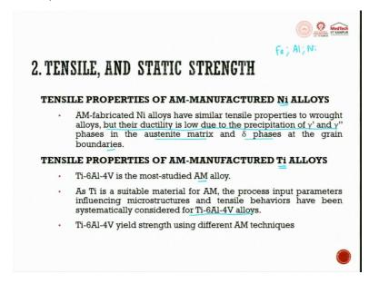
Tensile properties of additive manufactured nickel alloys, we have first talked about ferrous then we went into alloy aluminium and now we are going into nickel. Tensile properties of additive manufactured nickel alloys. AM fabricated nickel alloys have similar tensile properties to wrought alloy. But their ductility is low due to the precipitation of  $\gamma$ ' and  $\gamma$ " phases in the austenite matrix and  $\delta$  phases at the grain boundaries.
