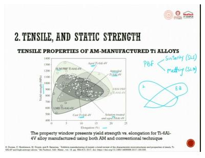
So, this is comparing about different techniques which are used for TI-6AL-4V. You can use selective laser melting technique. So, you have this is powder bed fusion selective laser melting. Powder bed fusion you have two techniques as I discussed earlier one is sintering and the other one is melting.
