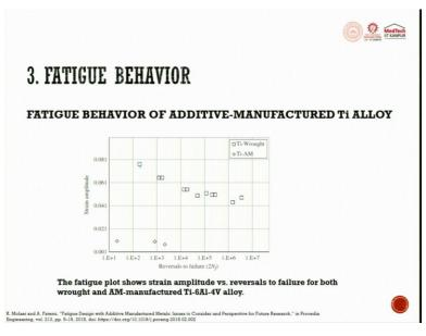
The fatigue behaviour of additive manufacture is shown here. So, you have strain accumulation and reversal or to failure you can see for titanium wrought it is here and for titanium additive manufacturing it is here.
