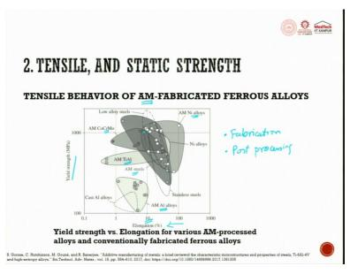
The tensile behaviour of additive fabricated ferrous alloys are listed here. So, this is predominantly called as Ash B curve. So, Ash B is a professor researcher, you can see such types of graphs comparing many different parameters. For example, in x axis here you have yield strength, y axis you have elongation, you can also try to have cost, he has drawn many things so, that you try to have better understanding.
