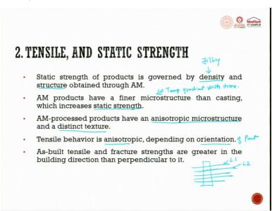
Tensile strength of products is governed by density and structure, density and structure, this density is the filling density which is governed by the structure what we use. Additive manufacturing products have a finer microstructure than casting, which we saw. Why? Because there is a temperature gradient with respect to time.
