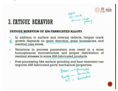
In addition to the surface and internal defects fatigue crack growth depending on the grain direction grain boundary and residual core stress, very important point it is not only because of the defect, crack and crack growing. It is also because of grain direction, grain boundaries and residual core stresses. These things also influences the crack propagation and reduces the fatigue behaviour of additive manufactured samples.
