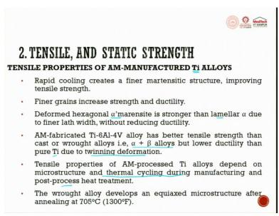
The rapid cooling creates a finer martensitic structure improving the tensile strength as far as Ti-Al alloys are concerned. Finer grains increase the strength and ductility hall petch effect. Deform the hexagonal alpha prime martensite is stronger than lamellar alpha due to finer lath width without reducing the ductility.
