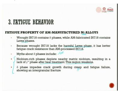
When we talk about nickel alloys as I told you ferrous aluminium then we will go to nickel and last we will see titanium. Wrought Inconel 718 contains  $\gamma$  phase while AM fabricated Inconel 718 contains laves phase. It produces a different phase itself because wrought Inconel 718 lacks the harmful laves phase.
