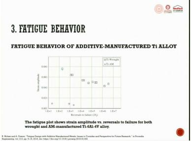
So, now for titanium alloys additive manufactured alloys have shorter fatigue life than wrought alloys. Internal defects which acts as micro notches and causes and cause stress accumulation greatly affect the AM alloy fatigue property. The post processing treatment removes or shrinks pores preventing them from fatigue failure.
