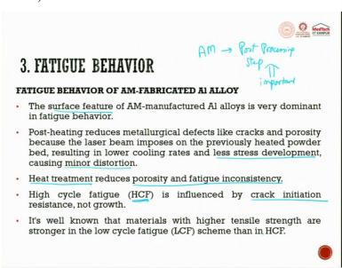
The surface feature of additive manufactured aluminium alloy is very dominating in fatigue behaviour surface feature. The post heating reduces the metallurgical defects like cracks and porosity, because the laser beam imposes on the previously heated powder bed resulting in lower cooling rates and less stress development causing minor distortion, less stress development. Heat treatment reduces porosity and fatigue inconsistency.
