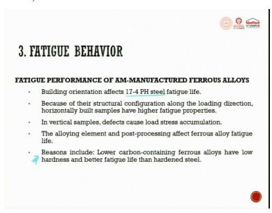
The fatigue performance of AM manufactured ferrous alloys are building orientation affects the 17-4 PH steel, this is a type of PH steel. You have to only worry about steel 17-4 PH steel fatigue life, because of their structural configuration along the loading direction, horizontal build samples have higher fatigue properties. In vertical samples that defects cause low stress accumulation.
