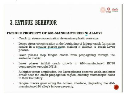
The fatigue behaviour of Ni alloys, the crack tip stress concentration determines the plastic zone size. Low stress concentration at the beginning of the fatigue cycle, fatigue crack formation results in smaller plastic zones making it difficult to break laves phase. Laves phase stop fatigue crack from propagating through the austenitic matrix.
