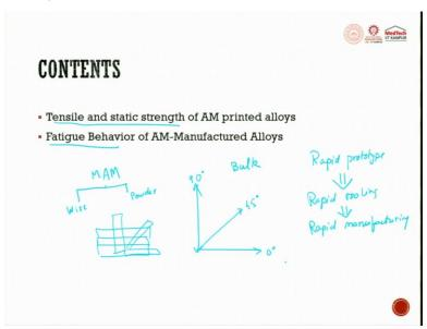
So, we would look at tensile and static strength of additive manufactured printed parts and then we will also look at fatigue behaviour, why are these two very important? Because, if you have a homogeneous material or a bulk material, so, if you do tensile test only in preferably three directions like for example, you do it in the 0 direction, then you do it in 90 direction and then you do around 45 direction, this is 0, maybe this is 0, this is 90 and you have 45°.
