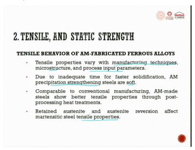
Tensile behaviour of additive manufactured fabricated ferrous alloys tensile properties vary with manufacturing techniques microstructure process input parameters with manufacturing technique, microstructure and process. So, what I am trying to say is, if it is electron beam, it will
