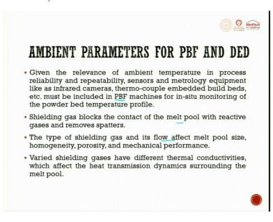
Given the relevance of ambient temperature in the process, reliability and repeatability and methodology equipment like as infrared camera thermocouple, embedded built heat beds etcetera must be included in the powder bed fusion. Shielding gas blocks the contact of the melting pool that reacts with the open gas.
