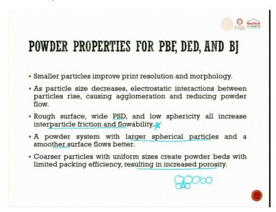
Smaller particles improve print resolution and morphology. As particle size decreases, electrostatic interaction between the particle rises, causing agglomeration and reducing the powder flow. Rough surfaces and wide particle size distribution and low sphericity all increase interparticle friction and flowability. This is very important.
