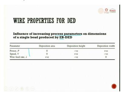
So here are the influence of increasing process parameters on dimension of a single bead produced by electron beam directed energy deposition. Power deposition area is 0, so deposition height is negative. And then the deposition width is positive. Speed. The deposition area is 0, so that means to say it is neutral. Then it is positive, means deposition height is more and then the deposition width is less.
