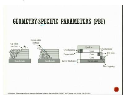
So when we talk about geometry-specific parameters, so you can see here build plate, upskin, this is the up-skin surface. This is the down-skin surface. Up-skin surface, down-skin surface, build plate. So here you can see overlapping down-skin, up-skin and you have coarse. This is the layer thickness.
