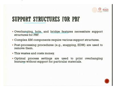
The last of this lecture support structures for PBF, overhanging whole bridge features necessitate support structure on powder bed fusion. Complex additive manufacturing components require various support structures. Post processing procedure are used to remove them, support structures which are built for overhanging holes and bridge features. This wastes and costs money. Optimum process settings are used to print overhang features without supports for particular material.
