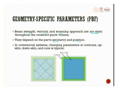
Beam strength, velocity, scanning approach are not static throughout the construction part volume, very important. It is not constant, not static. They depend upon the part geometry and position. The commercial systems change parameters at contours, up-skin, downskin, so this is the skin core. Up-skin, down-skin and the core is also changed layer by layer when it start building.
