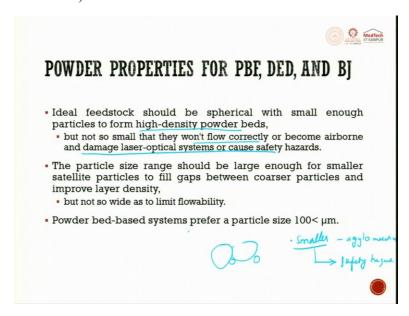
Ideal feedstock should be spherical with small enough particles to form high density powder bed. So what they try to say is you have larger powders, along with the larger powders you also try to have some amount of smaller powders. So this will try to go lock in the necessary positions and try to create high density powder bed but, not so small that they would not flow correctly or even air bound and damage laser optic system or cause safety hazard.
