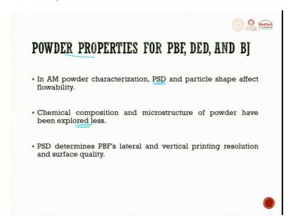
What are the powder properties? In additive manufacturing, powder characterization PSD and particle shape affect flowability. These two are very important. Particle size distribution. PSD and the particle shape effect affects the flowability. Chemical composition and microstructure of the powder have been explored less.
