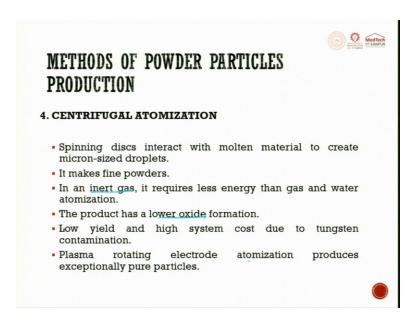
Spinning, so a droplet is drawn, so the spinning disc rotates, so the droplet goes to different places and it tries to create the powder. So spinning disc interacts with molten material to create molten size droplet. It makes fine powders, inert gas it requires less energy than gas or water, in inert gas.
