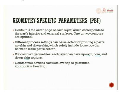
Contour is the outer edge of the layer which corresponds to the part interior and exterior surface. Different process setting can be selected for printing a part up-skin and down-
