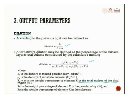
The other output parameter is going to be dilution. So according to the previous figure which is given,
