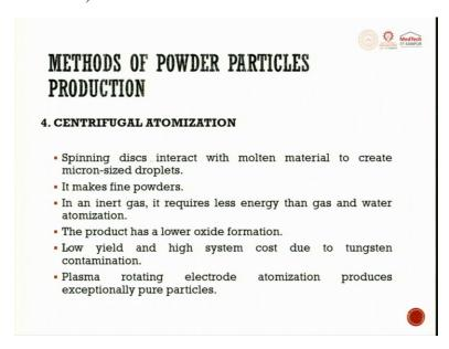
Centrifugal automation this is the last automation. So spinning disc interacts with the molten metal to create a micron size particle.
