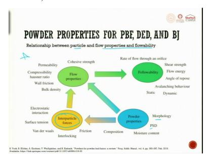
So if you try to take a relationship diagram between the particle and the flow properties and the flowability, you can see here flow properties, interparticle force, powder properties and flowability. So if you see here, flow properties goes to flowability. Rate of flow through an orifice, shear strength, flow energy, angle of response, all the three are important.
