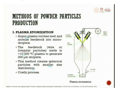
So the next one is going to be plasma. So you have a plasma torch, you have a plasma torch, melt wire spool is sent and then when the, both the plasma meet at this point, it tries to melt and then whatever comes out is, is the output of this melting. It gets shattered and you try to get small particles.
