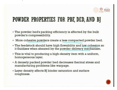
The powder bed packing efficiency is affected by the bulk powder compressibility. More cohesive powder creates less compaction, more cohesive powder, same, similar powders, it creates less compaction because there will be a space in between them. The feed stock should have high flowability and low cohesion. So it fluidizes when sheared by a powder bed mechanism.
