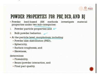
When we look at the powder properties for our powder bed fusion, directed energy deposition and binder jet, the powder bed based additive manufacturing methods investigate material property under two categories. One is powder particle properties, the other one is bulk powder behavior. So it falls into any one of these two categories. At the particular level, morphology includes powder size distribution, sphericity, surface roughness and skewness.
