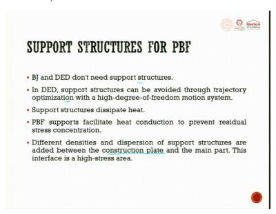
BJ and DED do not need support structures. In DED, support structures can be avoided through trajectory optimization. The support structures dissipate heat. The powder bed fusion supports facility, heat conduction to prevent residual stress concentration. Different densities and dispersion of support structures are added between the construction plate and the main part.
