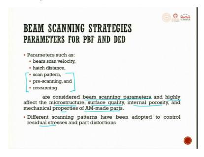
Beam scanning strategies is the next important parameter. So beam scan velocity, hatch distance, scan pattern, pre-scanning and rescanning are the other things which are important. So these three are very important. Scanning patterns, pre-scanning patterns, and rescanning patterns. Let us see that.
