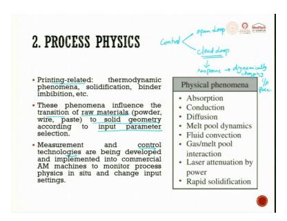
Process physics. Before getting into the process physics, these are some of the physical phenomena which generally dictate the laser process. Adsorption, conduction, diffusion, melt pool dynamics, fluid convection, gas metal pool interaction, laser attenuation by power, rapid solidification, these are all the physical phenomenas which try to dominantly play when we use laser or electron beam for additive manufacturing.
