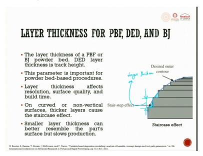
The layer thickness which have been all that I am talking about, this is called as the layer thickness. And this one is called as the staircase effect. Layer thickness of powder bed fusion or binder jet powder bed is the DED layer thickness is track height. This parameter is important for powder bed fusion procedures.
