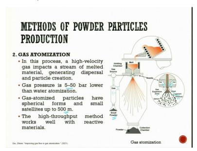
The next one is gas atomization. Gas atomization is very similar to that of your water. So you have a melt, so through this melt you will have a gas source which hits. So from here, all these things which are spraying here, these gases, so they will all try to spray in between the liquid, so it will try to settle down. And here, it will try to have lot of metal powders which are getting generated.
