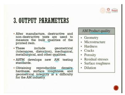
So what are the output parameters? After manufacturing, we try to do destructive and non destructive tests to measure the bulk qualities of the printed item. This include tolerance, distortion, mechanical, metallurgical and other qualities. Several ASTM standards are getting developed. Even now, ASTM standards for additive manufacturing are in a very, very prematured way.
