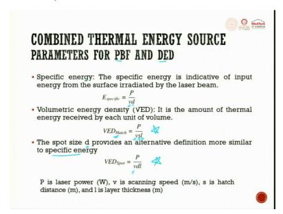
Combining the thermal energy source parameters for PBF and DED. These are some of the parameters. Specific energy, the specific energy is indicative of input energy from the surface irradiated by the laser beam.
