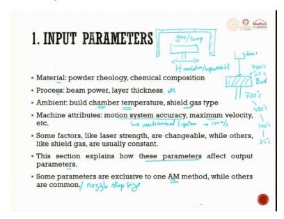
What is the physics? Here sintering and melting are the physics. What are the input parameters? Input parameters can be material. So when we talk about material, powder rheology, powder size, powder shape, powder topography, chemical composition, its electrical structures, all these things play a very important role.
