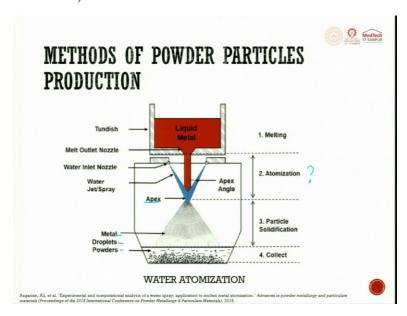
So this is how the water method is, water method is you have liquid metal coming, and then you will, you have a water inlet nozzle which sprays. So here also, it sprays. When it tries to spray on this, it instantly, there is an apex which is formed, and that, after that instant, it is all getting atomized. So you get a metal droplet powder which sperms and then it falls on top of it.
