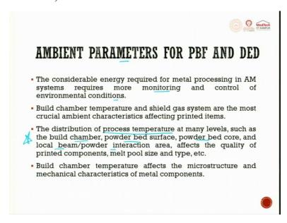
So the ambient parameters for powder bed fusion and directed energy deposition. Considerable energy required for the metal processing in AM system requires more monitoring and control of the environmental condition, build chamber temperature and shielding gas are most important crucial ambient characteristics.
