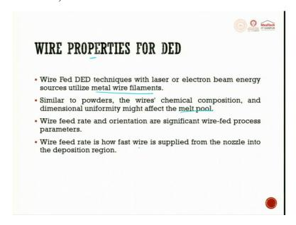
Now the last part of this lecture, wire properties for DED. Wire Fed DED technique with laser or electron beam energy source utilizes metal wire filament. Similar to the powder, the wire chemical composition and the dimensional uniformity might affect the melt pool. The wire feed rate and the orientation are significant wire fed process parameters. Wire feed rate is how fast the wire is supplied through the nozzle into the deposition region.
