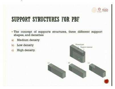
So these are all different support structures which are built. So a is medium dense, b is low dense, c is highly dense and this is a part, print part, there is a overhanging structure and this is a support structure.
