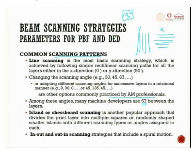
Line scanning is the most basic scanning strategy which is achieved by following simple rectilinear scanning path for all the layers either in the x-direction or in the y-direction, x-direction or in the y-direction, whatever it is. X-direction, this is x, and this is y. Changing the scanning angle from 30 to 45 to 67 etc. are also possible.
