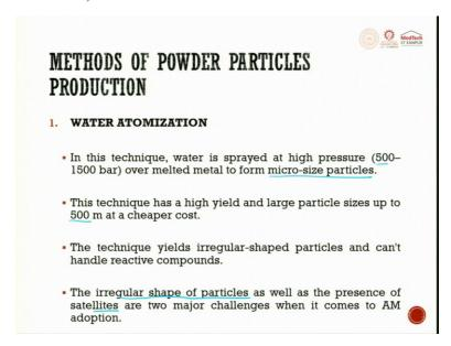
So water atomization, in this technique, the water is sprayed at a pressure of 500 to 1,500 bar over melted material to form micro sized particles. The technique has a high yield, and a large particle size up to 500 m at a cheaper cost can be made. The technique yields irregular shape particles and cannot be handle reactive components, this technique.
