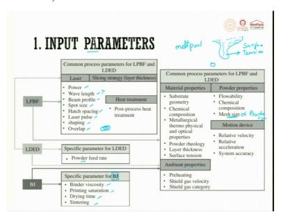
So these are the various input parameters for different processes. Let us take laser powder bed fusion. When we talk about laser, you have power of the laser, wavelength, that is  $\lambda$ , you have blue laser, green laser, red laser then you have beam profile. We saw the beam profile. So it can be TEM<sub>00</sub> mode, then Gaussian distribution mode, cowboy hat pattern mode, spot size is the least diameter, the smallest diameter which it can take.
