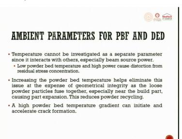
The temperature cannot be investigated as a separate parameter since its interaction with others, especially the beam source power. Lower powder bed temperature and higher power causes distortion from the residual stress concentration. Increasing the powder bed temperature helps eliminate this issue at the expense of geometric integrity as well as loose powder particles fused together, especially near the build area causing a part expansion.
