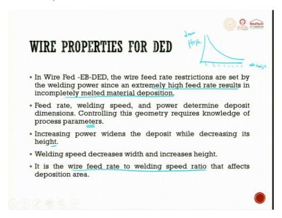
The wire fed electron beam directed energy deposition, the wire feed rate restrictions are set by the welding power since an extremely high feed rate results in incomplete pre melted material deposition. Very high speeds, incomplete melted metal deposition. Feed rate, weld speed, powder determination, deposition, dimension, cooling, this geometry requires a knowledge on process parameters.
