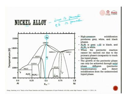
When we talk about nickel alloy, nickel alloy is pretty interesting. It is nowadays used in aerospace application you see at around about 2200 K, you find it as a liquid dropped down. So, you can see here at one phase it is Nickel, so, I dropped out and then I get into  $\beta$  phase. So, this  $\beta$  phase is different as compared to that of your  $\gamma$ ,  $\gamma$ .
