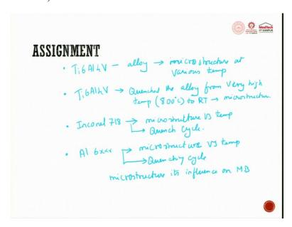
So, in this lecture I have few assignments for you. One is try to look for Ti 6Al 4V. So, try to look at this alloy and try to get its micro structure at various temperatures. Next try to see some literature on Ti 6Al 4V, where they have quenched the alloy from very high temperature, we are talking about  $800^{0}$ C to RT, room temperature. See the alloy microstructure.
