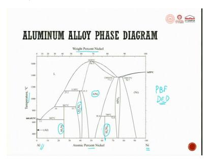
Next when we move into aluminium alloy phase, you can see weight of Nickel percentage is given here. So, you have temperature, you have atomic percentage of Nickel. So, this is used for aluminium and nickel getting fixed. So, this side is nickel and this side is aluminium, I have just taken an example of one particular alloy.
