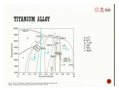
When you are looking at titanium alloy, it is titanium alloy you can see Ti 6Al V4 is the most common one which is used. So, you can see here when we are trying to change the aluminium composition with respect to titanium, let us assume it is dropping down somewhere here.
