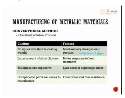
When we look at conventional methods, you have constant volume process. Under constant volume process you have casting and you have forging. In casting, there is no upper size limit in cast of weight. For example, big church bills can be made out of casting. Then large amount of alloy choices can be done by casting.
