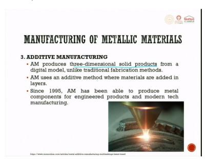
When you go to additive manufacturing, additive manufacturing produces three dimensional solid products from the digital mould unlike traditional manufacturing process, whatever is given in the drawing, you would convert it into STL file to slicing files.
