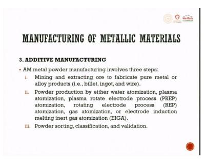
So, additive manufacturing, the metal powder manufacturing involves three steps. We have seen it in detail- mining and extraction, powder forming and powder sort classification and validation.
