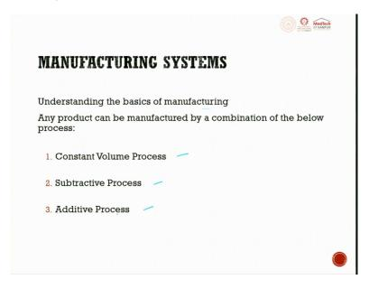
When you talk about manufacturing system, we first will try to understand the basics of manufacturing. Any product can be manufactured by a combination of the below processes, constant volume process, subtractive process and additive process. So, it can be one process, it can be one and two or it can be all the three together.
