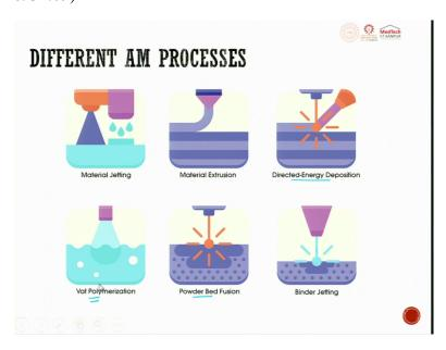
The material deposition can be done through extrusion, through material jetting, or through binder jetting. The difference between material jetting and binder jetting is binder is dropped, one after the other and the powder is agglomerated and then it tries to produce a layer. So, when we talk about material jetting, material in the jet form is dropped, so, that you try to get it. For example, wax.
