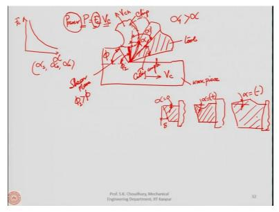
I showed it to you last time probably that if it is the cutting force and if it is one of the rake angles, so it goes like this meaning that as the  $\alpha$  increases, the  $F_c$  decreases. We always want the cutting force to be less. Power P is equal to  $F_c$  and the V<sub>c</sub>. So, if we can reduce  $F_c$ ,  $V_c$  being constant, in that case the power is reduced.
