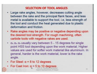
This is what it is written in this slide that the large rake angle however decreases the cutting angle, cutting angle is this angle, this is the cutting angle. Now this cutting angle is between the rake face and the flank face, this cutting angle decreases as we are increasing the  $\alpha$  that is the rake angle and the tool is becoming weaker because the tool is becoming thinner and less material is available.
