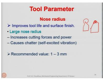
Now the nose radius. About the nose radius I told you that nose radius is given because sharp tool will always have a very high stress concentration around this point. Therefore, the tool is given a tool nose radius and that tool nose radius decreases the stress concentration around it and also improves the surface finish.
