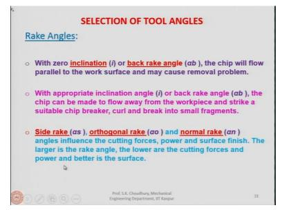
Let me remind you that last time what we discussed are the tool angles. We said that we have 3 sets of angles, namely one set of rake angles, one set of flank angles and one set of cutting edge angles apart from the tool nose radius. So, we have altogether 7 parameters, i.e. 2 rake angles, 2 flank angles, 2 side cutting edge angles and the nose radius by which a tool in any system is nomenclatured.
