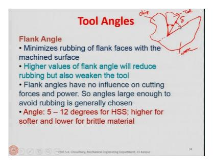
Now as far as the flank angles are concerned, a flank angle minimizes the rubbing of the flank faces with the machine surface. I will again draw this picture. Let us say I am not drawing fully the workpiece, this is the tool. This is the flank angle; this is the workpiece, this is the chip flowing, this being the tool.
