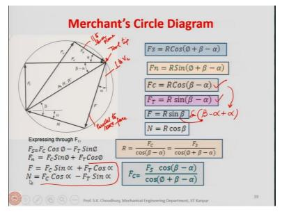
Now if we draw the circle with a diameter of R or R', they are the same, in that case the tips of all these components will be lying on the periphery of this circle because all these components F, N,  $F_s$ ,  $F_N$ ,  $F_c$  and  $F_t$  are the components of the one in the same resultant force R or R'.
