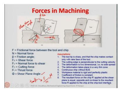
These are the forces in machining that are shown here. If we assume that the chip is a rigid body and it is moving at a constant velocity over the rake face of the tool with the cutting velocity  $V_c$ then the resultant of the forces acting on the chip from the tool through the rake face of the tool and the force acting from the workpiece through the shear plane of the process should be equal to zero. .
