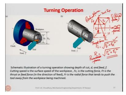
Here the turning operation is shown. This is the 3-jaw chuck, this is the workpiece mounted on the 3-jaw chuck. I will demonstrate this principle of the working in the laboratory when we will go to the lab. As you see here that the workpiece initial diameter is  $D_0$  and the diameter that we
