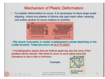
That is like as it is shown here. Initially the shear forces have been applied and because of this the layers of atoms have moved with respect to each other and now it has moved to such an extent or the magnitude of the force has reached to that extent that the plastic deformation started and upon removal of this forces we can see that the layers are not coming back to the initial position; they will stay here.
