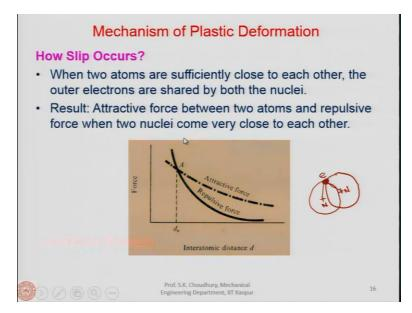
I am talking about this curve if you remember. So, this is the point where the tangent is shown here and this is the 0 point, means here at this point the attractive force and the repulsive force magnitude will be the same. Therefore, this distance shown here is called the equilibrium distance. Now suppose the atom has been moved from this position to this position at 'A'. 'Moved' means there is a shear force applied or strain rate applied.
