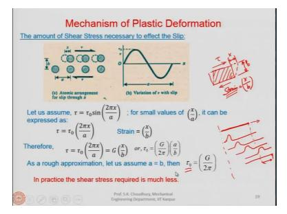
Next, let us see the amount of shear stress that is required for the deformation, meaning that how much force we have to apply for the plastic deformation to occur that we have to estimate because we have to accordingly design the machine because the machine tool ultimately will be involved in removing the material. What is that the movement of the atom we are talking about?
