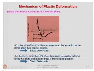
To continue with the mechanism of plastic deformation, elastic and plastic deformation can be explained in the atomic scale in the way that we have the net inter atomic force here along the Y-axis and along the X- axis we have the inter atomic distance. Now inter atomic force and inter atomic distance vary along this line. This is the nature of variation of inter atomic force with respect to the internet atomic distance.
