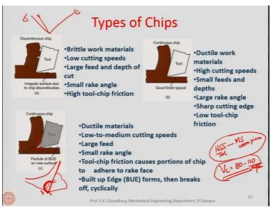
We will see the type of chips. Initially if you remember I told you that depending on the cutting parameters, work piece, combination of the work piece and tool material, and depending on the tool geometry, we will have different types of chips. And by the chip morphology or the type of the chip that is being produced during the process, you can diagnose many of the characteristics of the process.
