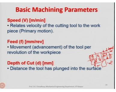
Now let us come back to the basic machining parameters. as we all know and I also told earlier that basic machining parameters are speed, feed and the depth of cut. Speed is normally taken in meter per minute that is that relates velocity of the cutting tool to the work piece that is a primary motion. Now the primary motion that is the cutting speed I narrated it earlier that in case of turning.
