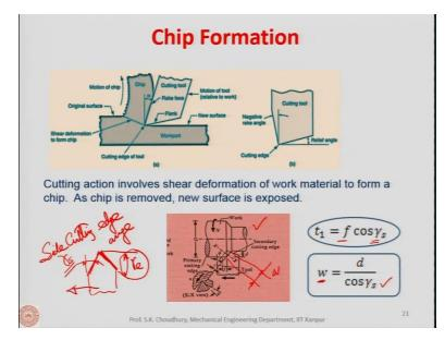
**Chip formation**: in the case of chip formation we said that this is the plastic deformation and finally it is the fracture which was shown in the stress strain curve or the force elongation curve, i.e. load elongation curve that after the point of instability it goes in a tri axial manner and it fractures means that it actually segregates. So, that is the chip formation. We are getting the chip.
