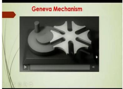
This mechanism it is another mechanism for transmitting the power from the input to the output shaft through the Geneva mechanism which is one of the most popular mechanisms when you have to transmit the power continuously rotating input drive input shaft when it transmits power to the output shaft which should be rotated not continuously but intermittently.
