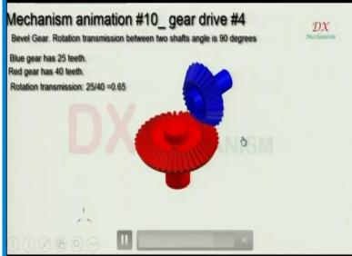
The next mechanism that is for transmitting the power through the gear drive. However, here you can see that the gears are bevel gears and these teeth of the bevel gear are cut at an angle, this is the input shaft on which the smaller gear is mounted and this is the output shaft where this red colour gear bevel gear is mounted. When we rotate them, as you can see that during the rotation this pulley which is this gear which is the input gear, this is transmitting the power to the output gear.
