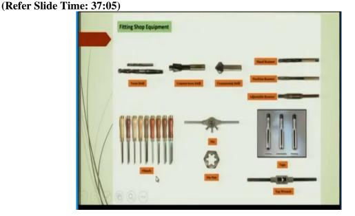
Other instruments or tools are twist drill. There are two different drills as shown here, one with diameter less than the other, both are twist drills. In this case you can see this is the portion which will be used to drill and as you know, the drill is used to make a hole, to drill a hole in a metal surface.
