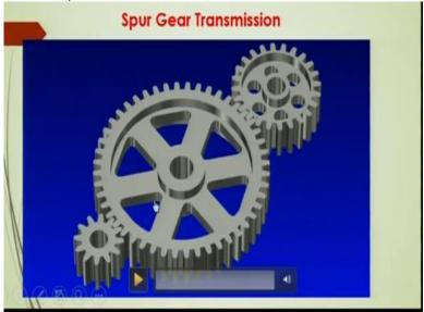
This is another mechanism. This is the gear train. Here all the gears are spur gears, there are 3 shafts one can be considered to be as the input shaft and this shaft on which this gear is mounted can be considered as the output shaft. The transmission is made, the motion is transmitted, power is transmitted from the input shaft to the output shaft through an intermediate gear.
