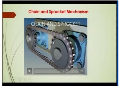
The next mechanism that you can see here is the chain and the sprocket mechanism which is similar to this belt drive mechanism only thing is that here the transmission is between the 2 sprockets or this is one sprocket, which is mounted on one shaft and this is another sprocket which is mounted on another shaft. This must be familiar to all of you because this is popularly used in the bicycle.
