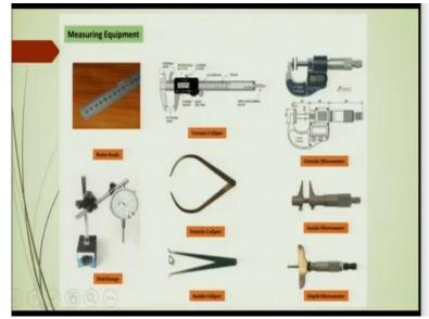
Next you can see the measuring instruments. This is the ruler scale, here you can see the vernier caliper. Vernier caliper is a precise instrument to measure the diameter of a cylinder or the external diameter of the cylinder or the internal diameter of the hole. External diameter can be measured by these jaws and internal diameter can be measured by these jaws and this is the scale.
