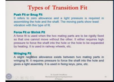
The types of transition fit can be push fit or snug fit, force fit or shrinks fit or wringing fit. These are the various types but all of them are transition fit depending on how much is the level of the transition in each of them. Here it is defined and that is defined based on the level of the transition in the fit.
