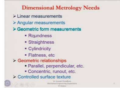
Dimensional metrology needs linear measurements, angular measurements, geometric form measurements, which include the roundness, straightness, cylindricity, flatness etcetera. And geometric relationship that is the parallel, perpendicular etcetera, concentric runout etcetera. These are the geometric relationship and for measurement will be this flatness, cylindricity, straightness, roundness and the control surface texture that I will come a little later.
