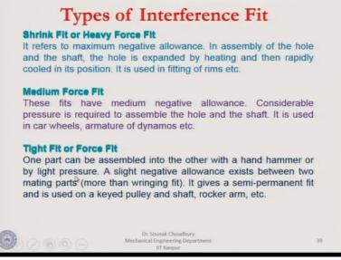
The types of interference fit also are different, shrink fit or heavy force fit where heavy forces are required. The diameter of the shaft is much more. Medium force fit and the tight fit or force fit are the different kinds of fits that are all interference fit.
