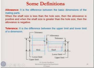
Now, here you can see what is allowance and what is tolerance? Allowance and the tolerance are given in this diagram. Let us say that this shaft goes into the hole. These 2 lines coincide, in that case we have a tolerance in the shaft as this much and tolerance in the hole as this much meaning the maximum diameter of the hole can be this and the minimum diameter of the hole can be this that this shaft can go in here; these are all highly exaggerated.
