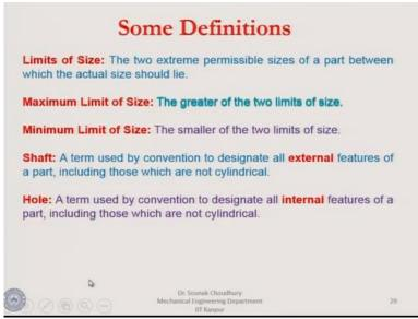
In the next diagrams, limit of size, maximum limit of size, minimum limit of size shaft and hole. These are some definitions. Limit of size is the two extreme permissible sizes of a part between which the actual size lies. Maximum limit, minimum limit these are variation of the limit of size. Shaft and hole terms are used by convention to designate all external features of a part including those which are not cylindrical and internal when they are mentioned through the hole term.
