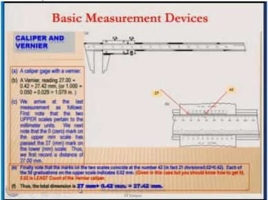
Here there is a normal vernier caliper what is shown here. So, here you can see that there is a main scale and there is a vernier scale; here there is a vernier scale as well. This can move along the length of the main scale and this is the jaw. Between these 2 jaws, the internal or the external diameter can be measured. Or the same vernier caliper can be used for measuring the diameter of the internal hole.
