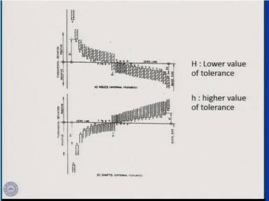
Here is the system given in more details. So, these are the internal holes and these the shafts, external features. Here you can see that H is the lower value of tolerance and h here is this
