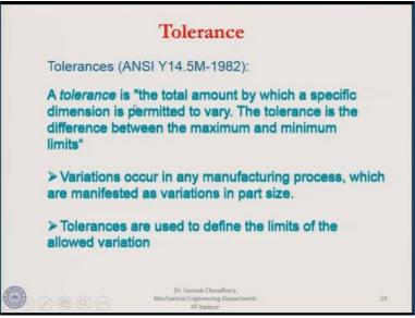
Therefore, a tolerance is the total amount by which specific dimension is permitted to vary. The tolerance is the difference between the maximum and the minimum limits. Variations occur in any manufacturing process, which are manifested as variation in the part size. Tolerances are used to define the limits of the allowed variation, how much we can allow; that is why it is called the tolerance - how much you can tolerate. This is the American society definition of the tolerance.
