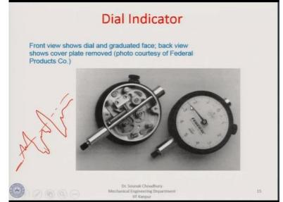
Here is the dial indicator, this is the probe and this probe is connected to the gear train and those gear trains are extremely sensitive. Therefore, as the probe goes up and down depending on that on the undulations in that case, this will be highly magnified by the gear train which is here and then accordingly the indicator will show you the deviation or the indicator will show you what are the discrepancies.
