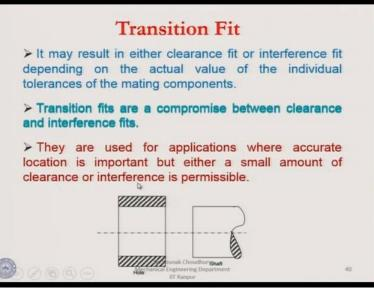
Transition fit it is neither very tight nor very loose. It is a compromise between the clearance and interference fit, they are used for applications where accurate location is important, location has to be very accurate, but either a small amount of clearance or interference is permissible.
