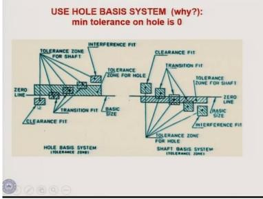
This is very important that we can use the dimension, which is a hole basis or the shaft basis. Normally we use the hole basis and why it is that it is shown here clearly. Use hole basis system so that the minimum tolerance on the hole is zero. Here you can see that this is the hole basis system. Minimum tolerance of this hole is zero and depending on that, we have the tolerance of the shaft. You can see that these are the different kinds of tolerances.
