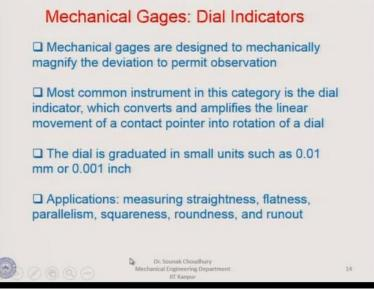
The mechanical gages, dial indicators are designed to mechanically magnify the deviation to permit observation. Most common instrument in this category is the dial indicator which converts and amplifies the linear movement of contact pointer into rotation of a dial. I will show you later what does it mean to convert and amplify the linear movement of a contact pointer into the rotation of a dial.
