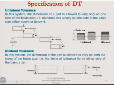
Tolerances are given as the unilateral tolerance in one side or it can be the bilateral tolerance where tolerance will be given from both sides.
