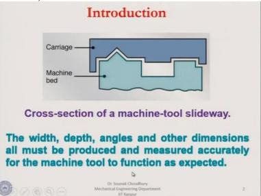
If you see the slides here, engineering metrology, if we have to define, before that that this is a machine tool carriage and this is the machine bed. The carriage moves over the bed on this length of the bed to and fro. This is the machine tool slide way. The width, depth, angles and other dimensions all must be produced and measured accurately for the machine tool to function as expected. Because it is a very lengthy machine bed and all along this the carriage has to move to and fro freely.
