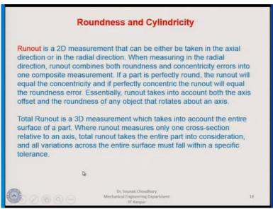
Runout is a 2 dimensional measurement that can either be taken in the axial direction or in the radial direction. Now, here this is the explanation given; runout takes into account both the axis offset and the roundness of any object that rotates about an axis, this is important. Now, here when measuring the radial direction run out combines both roundness and concentricity errors; this is also important here.
