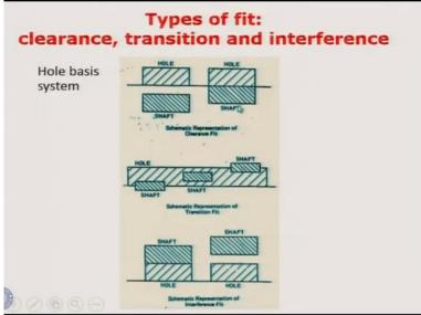
Types of fit are given here. This is the hole basis system and the hole is constant and then the shaft diameter is changing. Depending on that we have the clearance fit or the transition fit or the interference fit. We said that the clearance fit is when we have the clearance between them but that means the hole and shaft are relatively loosely fitted.
