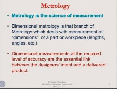
Metrology is the science of measurement, dimensional metrology is that branch of metrology which deals with measurement of dimensions, it can be length, it can be angles, it can be diameter. The dimensional measurements at the required level of accuracy are the essential link between the designer's intent and a delivered product.
