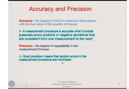
Let us see before we go into those details, let us talk about the accuracy of measurement. While using the concept of precision, we very often confuse between the concept of accuracy and the precision. Accuracy is the degree to which the measured value agrees with the true value of the quantity of interest; we have measured a value which may not be the true value of the quantity.
