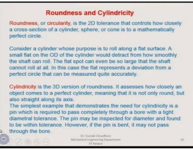
Roundness and cylindricity: let me give you a basic concept of the definition. Roundness or circularity is the 2 dimensional tolerance that controls how closely a cross section of a cylinder, sphere or cone is to a mathematically perfect circle. Roundness is a mathematically perfect circle where on the periphery all points will have a same radius from the centre.
