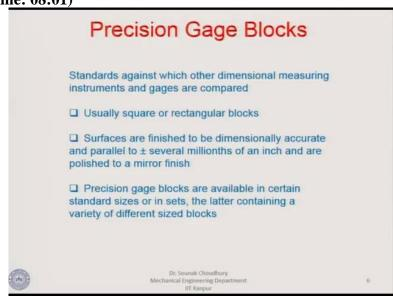
Precision gage blocks are standards against which other dimensional measuring instruments and gages are compared. Usually square or rectangular blocks since they are very precision then their sizes are very accurate. Surfaces are finished to be dimensionally accurate and parallel to plus minus several millionth of an inch and are polished to a mirror finish you may remember that these are the small blocks with absolutely smooth surface.
