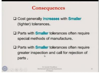
Cost generally increases with the smaller tolerances because if it is very tight tolerance, let us say 0.0001, you cannot really get it within that fine tolerance and if you have to get it then the machine has to be very accurate. Then the cost of the product will be very high. Parts with smaller tolerance also is called a tight tolerance often required special methods of manufacture. Parts with smaller tolerance often require greater inspection and call for rejection of the parts.
