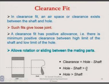
In one word, clearance is the hole minus shaft diameters. Clearance fit is that the shaft diameter is little less than the hole diameter, so, this is the loose joint. The clearance is the hole minus shaft and the hole is bigger than the shaft. So, hole minus shaft is more than zero.
