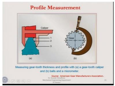
Next that we see is the profile measurement, so profile measurement is important particularly in the lab when we measured the gear profile it can be the bevel gear, it can be the spur gear it can be the worm and worm gear. This is important to exactly find out what is the profile. Here a gear tooth is shown. And this is how the gear tooth thickness can be measured with the help of vernier caliper.
