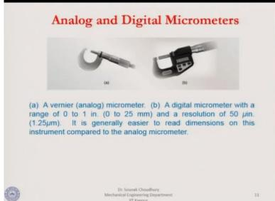
Now, these are the analog and the digital micrometres, analog micrometre has the main scale and round scale and rotating scale. Here it is round one and here it is the main scale. This is the vernier and then again depending on the dimension that is showing here, you can read from the main scale and the new round scale what is the actual reading up to the decimal level depending on the least count of the micrometre.
