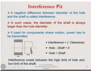
Similarly, we have the interference fit when we will have the hole minus shaft is less than zero that means the hole diameter is less than the shaft diameter. This is the interference fit, diameter of the shaft is always larger than the hole diameter. So, it snugly fits, tightly fits.
