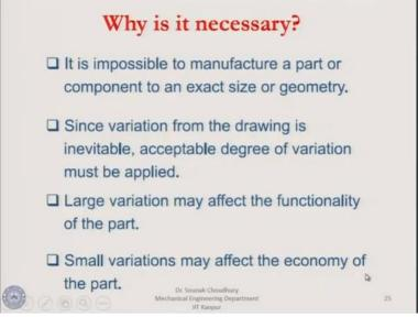
Why it is necessary because it is impossible to manufacture a part or a component as an exact size of geometry. Since the variation from the drawing is inevitable, acceptable degrees of variation must be applied. Large variation may affect the functionality of the part. Suppose if it is to be assembled, let us say that a shaft goes into the inner bore of the bearing.
