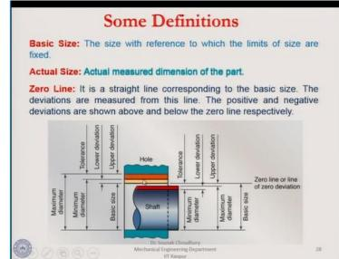
Let us see here. Here we have the hole, this is the hole and here is the shaft. For the shaft, this is the minimum diameter and this is the maximum diameter. So, this is the tolerance for the hole, the basic size of the hole is from here to here. This line we are calling as a zero line or line of zero deviation. Therefore, from this zero line how much we can have as the deviation we are saying that we can have up to this. Now, it is exaggerated .
