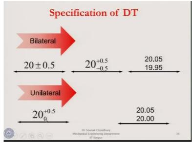
In case of unilateral tolerance, one side will be 0 and in case of bilateral tolerance, that both sides will be tolerance that means upper limit and lower limit both will have some limit.
