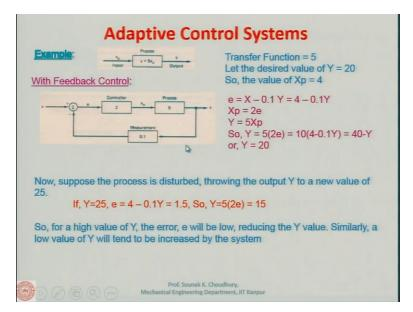
Now let me give you an example of the control systems and show you how the adaptive control system can be helpful in establishing or in controlling the output parameters. Whereas many of the NC systems, many of the closed loop systems even that we have discussed in the numerical control machines I mean earlier that they are also not capable of doing that let us take an example.
