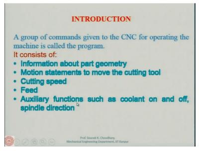
Let us say a group of commands given to the CNC for operating the machine is called the program, first of all. So, the program will consist of 5 points, that is the information about the part geometry, motion statements to move the cutting tool, cutting speed, feed and auxiliary functions such as coolant on and off spindle direction rotation of direction of the spindle clockwise or anti clockwise and so on.
