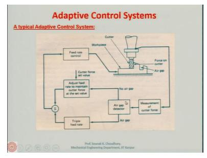
Let me give you an example of a typical adaptive control system. So, let us say we have the face milling cutter and this is the workpiece. Now here what happens that this is the interrupted cutting and in between we have some sort of air gap. The system contains a sensor which senses the cutting force, continuously the cutting force is measured.
