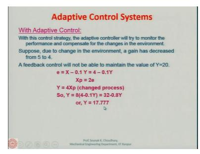
Now with adaptive control system the adaptive controller will try to monitor the performance and compensate for the changes in the environment. Suppose due to change in the environment again the gain has decreased from 5 to 4. In the next example we will see that in that process because of some disturbance from outside, this process gain has been changed from 5 to let us say 4, then what happens? Let us see.
