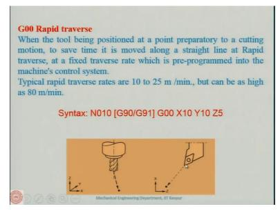
The rapid traverse is given here. There is a program for the rapid traverse and there is a code for the rapid traverse that means rapidly how to move the tool from the 0 position to the actual position that you want near the workpiece.
