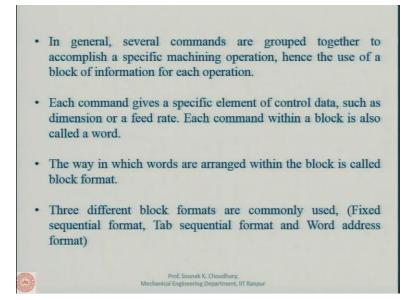
In general, several commands are grouped together to accomplish a specific machining operation, hence the use of a block of information for each operation each command gives a specific element of control data such as dimension or the feed rate. Each command within a block is also called a word. Now we have a block of few commands and each command is a word.
