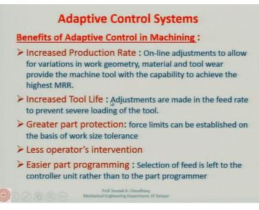
Benefits are many fold like the increased production rate, that is, the online adjustments to allow for variations in the work geometry material and tool wear provide the machine tool with the capability to achieve the highest MRR and highest MRR means the high production rate, increased tool life because adjustment can be made in the feed rate to prevent the severe loading of the tool.
