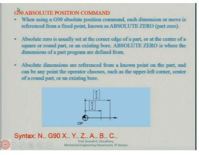
Absolute positioning: I already explained, the details are given in the slide. So, you have to say what is incremental what is absolute in the program, if it is absolute the code is G90 and so on. (Refer Slide Time: 57:40)
