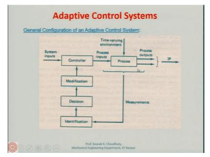
So, here you can see the general configuration of an adaptive control system in the block diagram. This is the process. Now in this process we have some process input and we are getting some output. On this process there are some time varying environment and by that we mean to say that there are certain kinds of disturbance.
