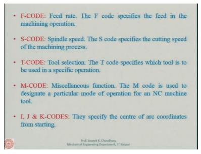
F-CODE is the feed, S-CODE is the spindle speed, T-CODE is the tool selection, M-CODE is a miscellaneous function I, J and K-CODES they specify the center of an arc and particularly it is when you are giving the circular interpolation. We will see that I, J and K codes can also be given as a circular interpolation.
