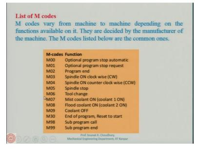
For example, this is the M code, M05 code is to stop the spindle, tool change will be M06 and so on. Even whether you want to do the mist coolant or the flood coolant that also should be given in the program because again there is no intervention of human beings. So, a human being is not there and cannot change the coolant from mist to flood.
