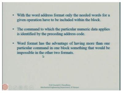
With the word address format only the needed words for a given operation have to be included within the block it and so on. So, what format has the advantage of having more than one particular command in one block over something that would be impossible in other 2 formats and so on. So, these are the differences between the 3 formats and how they differ from each other.
