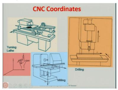
It has to be given in program and finally these are the coordinates. I told you already that in case of turning lathe the movement in this direction is considered to be x axis and in this direction is the z axis. In case of drilling this is z this is x this is y, in case of milling this is z this is the
