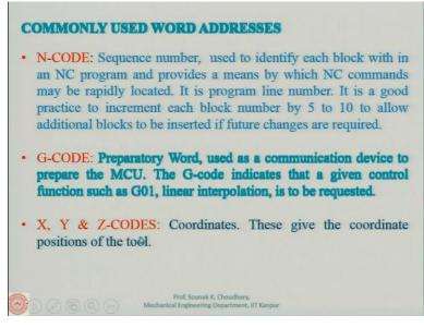
Commonly used addresses are the N-CODE which is the number here N is 50, N is 60, N is 70, so this is the number of this line each line is given by a number N-CODE, this is the sequence number; G-CODE is a preparatory word used as a communication device to prepare the MCU machine control unit. The G code indicates that a given control function such as G01 for example, stands for linear interpolation.
