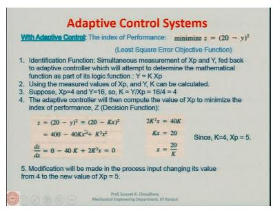
Now let us see with adaptive control. Here let us say the index of performance we will select is z which is  $(20 - y)^2$ . This is called the least square error objective function. 20 is the desired value this is the y which is output so  $(20 - y)^2$  is the index of performance and then our task as the adaptive control system will be to minimize this z.
