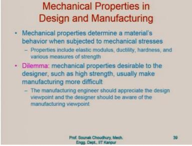
**Mechanical properties in design and manufacturing:** mechanical properties determine a material behaviour when subjected to mechanical stresses. Properties include elastic modulus, ductility, hardness and various measures of strength. Here the dilemma becomes that mechanical properties, desirable to the designer such as strength usually make manufacturing more difficult, what we mean to say is that there is a concept of machinability which indicates the ease of machining.
