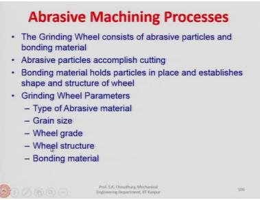
The grinding wheel consists of the abrasive particles and the bonding material because the materials have to be properly bound inside the grinding wheel. So the binding material is important because how strong the grinding wheel will depend on the binding material. Bonding material holds particles in place and establishes shape and structure of wheel
