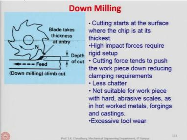
In down milling, the cutting starts from here. First of all, in down milling, the rotation of the milling cutter is in the same direction as in the feed given to the workpiece. Down milling is also
