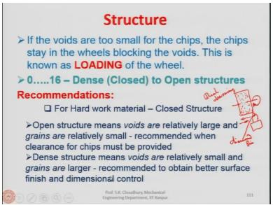
Ff the voids are too small for the chips to stay in the wheel blocking the voids and this is known as the loading of the wheel. So, wheel loading is also not desirable like the wheel glazing. So, in wheel loading case it is the layer of the clogged chips and in case of wheel glazing it is the layer of the board grains. Both of these have to be removed.
