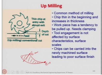
Here is the popular categorization of the milling. This is called the up milling. You must be familiar with that, this is the milling cutter and this is the workpiece. Up milling is when the direction rotation of the milling cutter and the feed movement given to the workpiece are different. This is a common method of milling mostly you will see in practice the up milling is used now.
