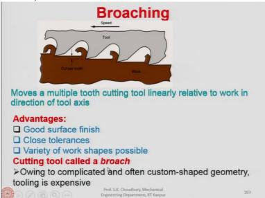
Next is the broaching operation and the broaching operation is very typical operation that we see it is somehow different than the other operations in the sense that here the feed is not given to the tool separately in the sense that for feeding like that concept which we had so far which we have seen in case of turning or milling, the feed in broaching is given by increasingly given the diameter of the teeth. Now, let me explain it to you.
