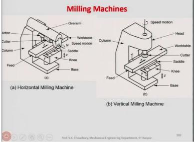
These are the milling machines, these machines we will see in the laboratory, this is the horizontal milling machine because the axis of the milling cutter is horizontal and here since the axis of the milling cutter is vertical, so, this is called a vertical milling machine. So, in the horizontal milling machine you will see that on the base the entire machine is located including the over arm on which we have the milling cutter.
