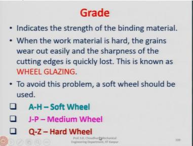
Next is the grade, the grade indicates the strength of the binding material. When the work piece material is hard, the grains wear out very easily and the sharpness of the cutting edges is quickly lost. This is known as the wheel glazing. I will explain to you why it is important. First of all the phenomena is that when the work piece material is hard and the grinding wheel is hard then the grinding wheel will be worn out because the surface is very hard or work material is hard.
