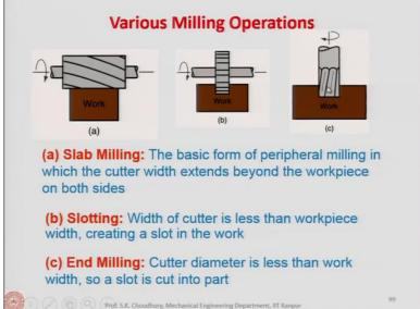
Various milling operations are categorized as the slab milling. This process is slab milling process which is the basic form of peripheral milling in which the cutter width extends beyond the workpiece on both sides. It means that the in the case of the slab milling in one go the entire width of the workpiece can be machined.
