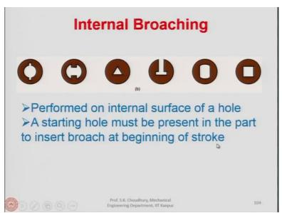
These are the internal broaching shapes. This is the hole with the slots. It may be used for the key holes, this hole is for different types, different types holes can be made here like triangular shape of the internal hole, this is a slot. This is a T-slot, this is another slot with the semi-circular shape and this is the square hole. If you see here that this is a cylindrical surface and this hole is the square hole and that the making an internal square hole is very difficult.
