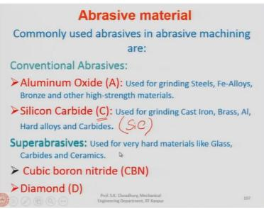
Commonly used abrasives making the grinding wheel or the honing or the lapping are of three types. Basically, we have three types of abrasives which are used: aluminum oxide which is designated by A, silicon carbide which is designated by C and rarely used are the cubic boron nitride CBN or the diamond.
