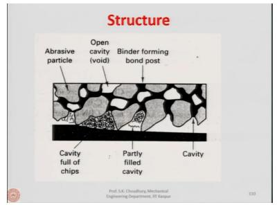
A very enlarged view of the surface of a grinding wheel is shown and you can see that in between the grains there is a void. Void is the space to accommodate the chips like in case of the milling cutters. In milling cutter, I have shown it to you when we were discussing the up milling, down milling that between the teeth there is a space that is called the void and that in those voids the chip is accommodated.
