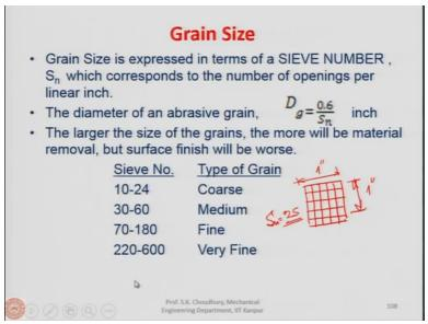
Regarding the grain size that means how we are defining the performance of the grinding wheel depending on the grain size. Grain size is expressed in terms of the sieve number. Sieve number is a  $S_n$  suppose, which corresponds to the number of openings per linear inch. What does it mean is the following that just imagine that if you have an opening which is 1 inch by 1 inch, let us say this is the square, this is 1 inch and this is 1 inch.
