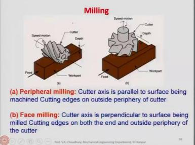
Here schematically we have shown the milling process, this one is the peripheral milling. Peripheral milling means that the cutter axis is parallel to the surface that is being milled and cutting edges on the outside periphery only. You can see that that this is the milling cutter, this is how it rotates and this is the axis of the milling cutter and this axis is parallel to the surface. Both are in the horizontal plane that is a surface that is being made and the cutter axis.
