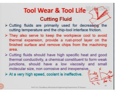
Cutting fluids are primarily used for decreasing the cutting temperature. I told you that and the chip tool interface friction. So, there are two actions of the cutting fluid, one that is when the
