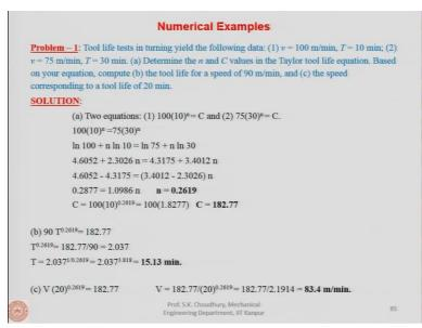
Numerical problems: How we can implement one of the tool life equation, the tool life theory that we have learned. Let us say tool life test in turning. In the following data, cutting speed is 100 *m/min* when the tool life has shown to be 10 *min* and as the cutting speed decreases to 75 *m/min* that tool life increases to 30 *min* from this data we have to determine the constants *n* and *C* values of the Taylor tool life equation.
