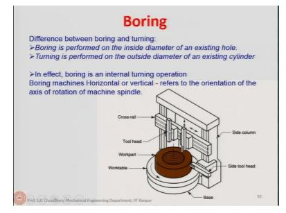
Now as I said about the boring, I will go quickly through this that the difference between the boring and turning is that boring is performed on the inside diameter of an existing hole, the hole already exists and boring is performed so that the internal hole is enlarged. Turning is performed on the outside diameter this is a turning and inside this the boring tool. The boring is made to enlarge that. In effect boring is an internal turning operation.
