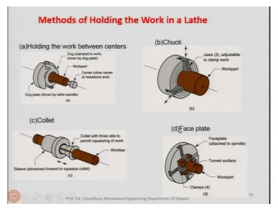
Here you can see the methods of holding the workpiece in a Lathe. Here is the holding between the centers. This is the center in the tailstock and this is the other side which is held on another center on the headstock. The rotation is given by a dog carrier. Here is the dog plate and this is called the dog and the dog carrier, this is the carrier dog plate which is fixed here with the workpiece.
