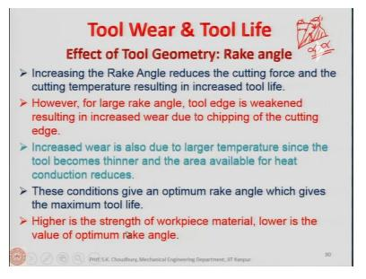
Then we said that increasing the rake angle reduces the cutting force. And then in the final conclusion, we said that higher the strength of workpiece material, lower is the value of the optimum rake angle.
