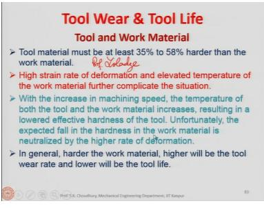
Now, next is tool and work material. The overall research says that the tool material must be at least 35% to 58% harder than the work material. This conclusion has been made by the research
