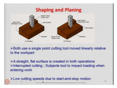
Shaping and planing both use a single point cutting tool and moved linearly relative to the workpiece. The shaping operation, we will show you in the lab also in more details. This is the shaping where the tool reciprocates and with each reciprocation that is going forward and going back. Once the feed is given to the workpiece and here it is opposite in case of planing when the workpiece reciprocates and the tool is given the feed.
