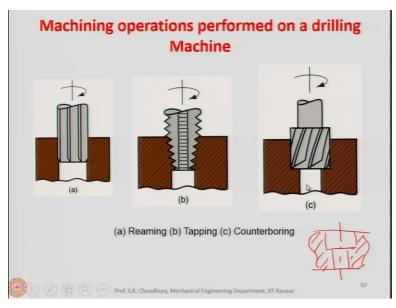
Here is what I was telling you about the reaming. The reaming process is done after the hole is drilled to increase the surface finish of the hole because after the drilling, the drill always will have the vibration, drilling machine will be having the vibration and normally the drilling operation is the rough operation because the entire material is to be removed and there was no hole the entire hole is made but in case of reaming the hole is already there.
