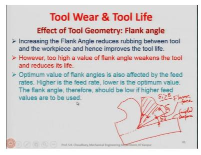
About the flank angle, I have shown it to you that as the flank angle is increasing then cutting angle of the tool is decreasing and the tool becomes weaker and the material available for the heat conduction will be less. We also said that the optimum value that we are getting for flank angle also affected by the feed rates. That means higher is the feed rate, lower is the optimum value the flank angle. Therefore, it should be low if higher feed values had to be used.
