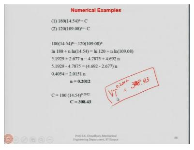
So, you can find out what is the  $VT^n = C$  in first and second cases. In both cases, V and T are different we have found out from these conditions that if the cutting speed is 3 *m/sec* then tool must be changed after 5 work parts and the second equation is if cutting speed is 2 *m/sec* then the tool must be producing 25 pieces, from here we can get these 2 equations.
