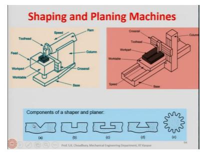
Shaping and planing machines are like this, this the shaping machine where the tool reciprocates and this is the planing machine where the workpiece is longer than in case of shaping machine and the workpiece reciprocates. This is the base of it. This is the worktable on which the workpiece is mounted and this is the cross slide, cross rail and it is the tool head. Similarly, this is the tool head and this ram reciprocates with the tool.
