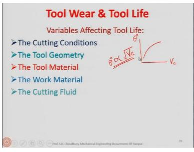
These are the 5 variables which affect the tool life. The temperature occurring during the machining process is proportional to  $\sqrt{V_c}$ .
