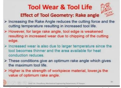
Now, effect of cutting conditions we are not discussing separately because here we have already shown that apart from the cutting velocity, the feed and the depth of cut also affect the tool life and this is in this way that the cutting speed has the greatest effect followed by the feed and then the depth of cut. How the tool geometry affects the tool life? Let us consider first the rake angle.
