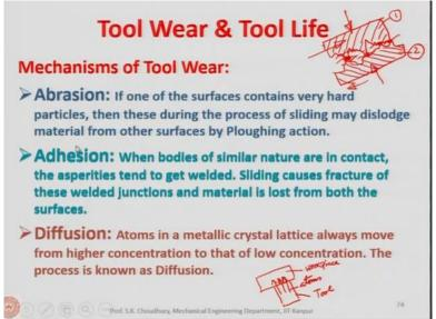
Mechanisms of tool wear: we have 3 main mechanisms. There are other mechanisms as well, but basic mechanisms of tool wear are the abrasion, adhesion and diffusion. Abrasion is when one of the surfaces contains very hard particles then these during the process of sliding may dislodge material from other surfaces by ploughing action. Let me give you an example. Suppose, you have a chalk which is with absolutely sharp edges and flat at the other end and you write something on the board.
