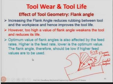
Now, let us discuss the flank angle. Increasing the flank angle reduces the rubbing between the tool and the workpiece and hence it improves the tool life. Once again, I will remind that this is the tool and here is the workpiece, this is the workpiece, this is the tool. So, this is the flank face or the flank surface or as I said that it is also known as the clearance face and this is the flank angle, flank angle we designated by  $\delta$ .
