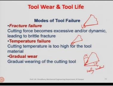
Now we will discuss our next topic which will be tool wear and tool life. Modes of tool failure: the tools during the machining process can fail, they can have fracture failure. So, excessive cutting force may lead to the brittle fracture of the tool. Temperature failure: cutting temperature is too high for the tool material. So, they get thermally deformed or the gradual wearing of the cutting tool takes place. To give you an example, let us say that we had a sharp tool.
