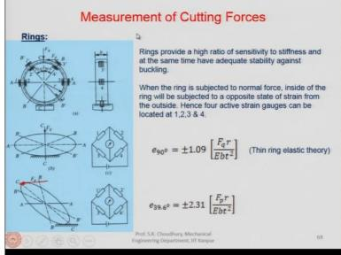
Now let us discuss the measurement of cutting forces when there is a ring type structure used. Here you can see that there is a ring type structure and this ring type structure is rigidly mounted on the base somewhere and this structure has the pitch circle diameter, this is 2r and it has the thickness *t* and the width of this is the *b* which has been shown in the side view
