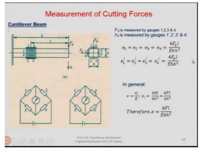
Next, let us discuss the measurement of cutting forces with the help of a cantilever beam. This is the cantilever beam shown; let us say on this cantilever beam, there are 2 opposite forces. If this is the cantilever beam which is fixed on one side then there are 2 loads, one vertically located another one is the vertical to that at a  $90^{0}$  angle to that that is located like this.
