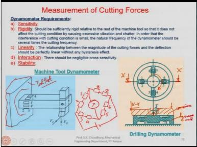
Now for the measurement of cutting forces, the dynamometers that are used have certain requirements. And whatever is the dynamometer it is either a ring type dynamometer or it is a cantilever beam dynamometer or it is an octagonal dynamometer all these requirements remained valid for all of them. First is the sensitivity
