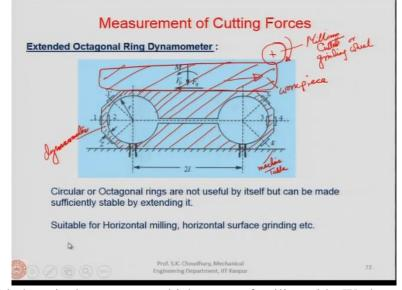
Sown in the slide here is the structure which we are familiar with. We have seen one of the smaller versions of that is the octagonal dynamometers and we said that it is a modification of the ring type dynamometer. Here the, octagonal dynamometer has been further modified you can see this. Now here the rigidity of the octagonal dynamometer has been further increased.
