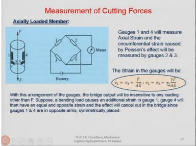
Then we started discussing if you look at this slide, we have discussed the axially loaded member and here is that axially loaded member; here is the load acting on the member. What was said is that there are strain gauges or as I said that this can be the piezoelectric elements.
