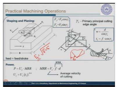
During the discussion on shaping and planing we said that the forces are different and we have shown the forces,  $F_n$  is perpendicular to the finished workpiece.  $F_f$  is along the feed direction and their sum is the  $F_T$  which is the thrust force which is given by  $\sqrt{F_f^2 + F_n^2} = F_T$ . By the way this  $F_T$  is perpendicular to the transient surface, this is the transient surface.
