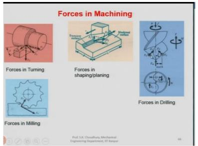
Let us see how forces in machining act. I have already shown you the forces acting during the turning process. In shaping and planing, it is like this, in milling it is the total tangential force and in drilling the thrust and torque are given by  $F_c$  and the thrust is given by the  $F_t$ . Now we will discuss how these forces can be measured.
