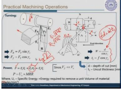
Let me remind you that we were discussing in the last discussion session the practical machining processes, practical machining operations and we discussed initially how the forces in turning are distributed. As you can see in this slide this is the workpiece and the forces are in the parallelopiped. Here is the pictorial view of the turning process; this is the feed which I said as the linear movement of the tool in mm per revolution of the workpiece.
