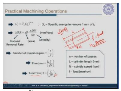
This is given as  $U_c = U_0 (t_1)^{-0.4}$ . This is an empirical formula empirical formula means that this is obtained experimentally. You cannot derive this formula because it is obtained experimentally;  $t_1$  is uncut thickness and this is the coefficient (-0.4) obtained experimentally as an exponent. Now  $U_0$  which we said as the specific energy coefficient, by definition it is the specific energy to remove 1 mm of  $t_1$ .
