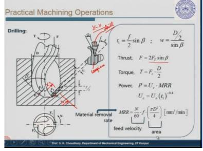
Next is the in the practical machining operations t is the drilling. The tool which is used for drilling a hole, of course, you understand that the drilling process is used for making the hole, the hole maybe the blind hole or it may be a through hole and the tool is the drill. Here you can see the schematic of the drill. In drilling one difference is that here there are 2 teeth. this is the difference between the single point cutting tool in turning where the cutting tool has a single point.
