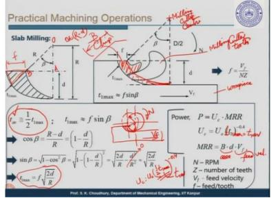
Now, let us discuss the milling process. We will take the example of the slab milling. In slab milling, this is the schematic of this slab milling where this is the workpiece, and this is the milling cutter for which one tooth has been shown. The milling cutter will be like this with all the teeth and this is the diameter, this is the center of the milling cutter. Milling cutter is rotating like this. It will have other teeth all over the periphery of the milling cutter.
