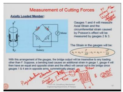
Let us see how the forces are measured for the axially loaded member. The member is like this as shown in the slide. This is a cylindrical job and it is loaded axially. The force is applied from both ends; it is being pulled. This is a cylindrical job and from both sides it is being pulled by some kind of a device. Here we have the sensors which are called the gauges, a gauge which will measure the forces.
