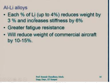
In aluminium lithium alloys, each percentage of lithium up to 4% reduces weight by 3% and increases stiffness by 6%. This is the experimental results and you can see the effect of each percent up to 4% reduces weight by 3% this is a drastic reduction in the weight and increases the stiffness by 6%. So, both these characteristics like the weight and increased stiffness are desirable in the engineering materials and in the engineering parts.
