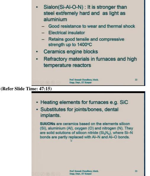
Sialon is a relatively new material. Definition of sialons is that it is ceramics based on the elements silicon, aluminium, oxygen and nitrogen that is why the name evolved as sialon. They are solid solutions of silicon nitride Si 3 and 4 where silicon nitrogen bonds are partly replaced with the aluminium nitrogen and aluminium oxygen bonds. This is how the sialon has been invented that silicon nitride bonds are partly replaced by the aluminium nitrogen and the aluminium oxygen bonds.
