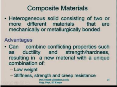
Now composite materials are the materials which have lately started being used very extensively because of their unique properties particularly they are light and strong and they are relatively less expensive, and can be produced relatively easily. Heterogeneous solid consisting of two or more different materials that are mechanically or metallurgically bonded are the composite materials. Once again, these are the heterogeneous solid.
