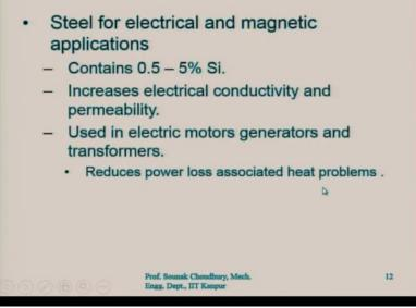
Steel for electrical and magnetic applications: those compositions will be different because the demands from those deals in the area of electrical and the magnetic applications will be different. Those kinds of steels may have 0.5 to 5% of silicon that increases the electrical conductivity because we need it for electrical application and permeability. So, because of that these two properties such as conductivity and permeability are given by the silicon.
