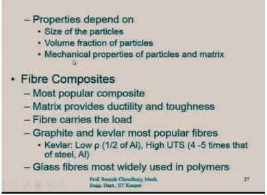
Properties also depend on the size of the particles, volume fraction of particles. That means, how much which particles are in which volume, i.e. what is the fraction of this volume, fraction of those particles in that volume and the mechanical properties of the particles and the matrix both. In the composite material, the properties of these particles or the matrix may not be retained.
