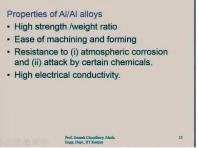
Properties of aluminium and aluminium alloys: First of all, high strength to weight ratio. The ratio of the strength to weight is very high. So, we understand that for less weight very high strength can be achieved. Next is the ease of machining and forming because it is relatively softer material. Therefore, the machinability is good and the formability is better.
