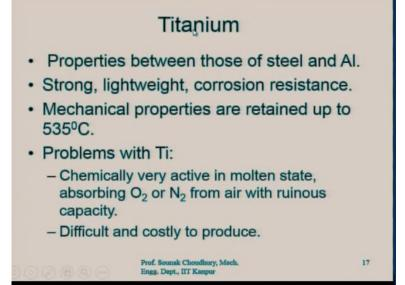
Titanium properties are between those of steel and aluminium. So, you understand that all the properties that the steel and the aluminium have, the properties of the titanium will be in between. We will discuss in details what are those strong, lightweight, corrosion resistance. These are the three properties which are also very important for the field of engineering materials because materials have to be stronger and the weight has to be lighter.
