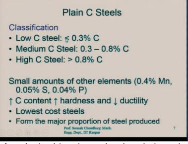
**Plain carbon steels**: under the plain carbon steel we have the low carbon steel where we have the percentage of carbon less than 0.3%. Then we have the medium carbon steel. Medium carbon steel is a little more than the low carbon steel in terms of carbon content and it is between 0.3 and 0.8%. So, you understand that the medium carbon steels have different grades depending on the percentage of carbon. In some grades it may be 0.3 and 0.4, 0.5 and so on but not more than 0.8% of the carbon.
