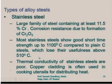
Now, the types of alloy steels. There is stainless steel; stainless steel as you everybody know that nowadays it is very useful and very widely used. Large family of steel containing at least 11.5% of chromium, this is one of the alloying materials in the stainless steel. Corrosion resistance is due to the formation of chromium oxide since there is chromium. Therefore, it does not allow the corrosion since the chromium oxide is fromed.
