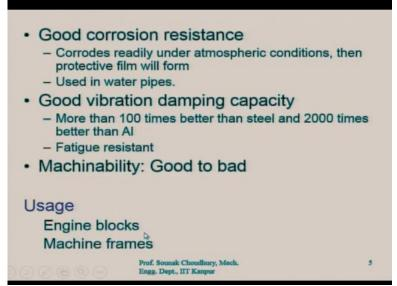
The cast iron has good corrosion resistance. What happens is it corrodes readily under the atmospheric conditions and then that is used as a protective film, a protective layer. So, further the material underneath will not be corroded. The corrosion happens at the top and after that it does not allow the corrosion to go in. Therefore, it is used in the water pipes which are made, as you know, in huge quantities.
