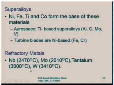
Therefore, materials like super alloys are invented. Nickel, ferrous, titanium and cobalt form the base of these materials. These are the super alloys formed by nickel, ferrous, titanium and cobalt. In aerospace particularly the titanium based super alloys, for example aluminium made of aluminium carbon, molybdenum, vanadium along with the titanium. Titanium will be the base which is very widely used in the aerospace particularly because they are very light.
