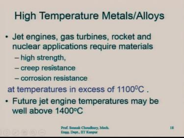
High temperature metals and alloys, jet engines, gas turbines, rocket and nuclear applications, require the materials with high strength, creep resistance, corrosion resistance since they are working at a very high temperature. So, the forces exerted will also be higher, and the temperature rise will be higher.
