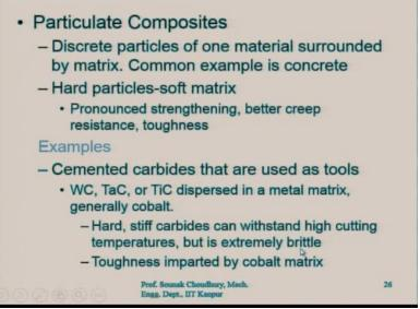
Particulate composites are there, particulate composites are the discrete particles of one material surrounded by a matrix. Common example is a concrete it is a discrete particle of one material like cement, surrounded by matrix. So, this can be the cement and the granules and then the sand. That will be the concrete having pronounced strengthening, better creep resistance and toughness.
