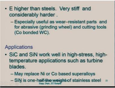
Young's modulus is higher than the steel; Ceramics are very stiff and considerably harder, especially useful as wear resistant parts and for abrasive. Very often ceramic particles are used as abrasive material (silicon carbide for example). Silicon carbide, silicon nitride have the moderate toughness. Those silicon carbide particles are also used as the grinding wheel grits.
