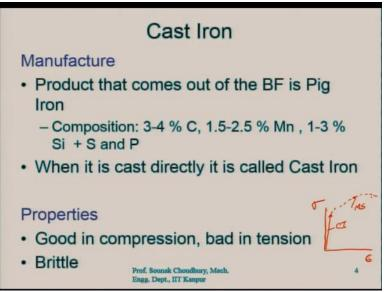
Now, let us discuss the ferrous metals first. Under the ferrous metal the most popular is the **cast iron**, and the cast iron is the product which comes out of the blast furnace that is the pig iron initially. The composition of the pig iron is about 3 to 4% of carbon, 1.5 to 2.5% of manganese, 1 to 3% of silicon and sulphur and phosphorus additionally. So, this is the product which comes out of the blast furnace which is known as the pig iron.
