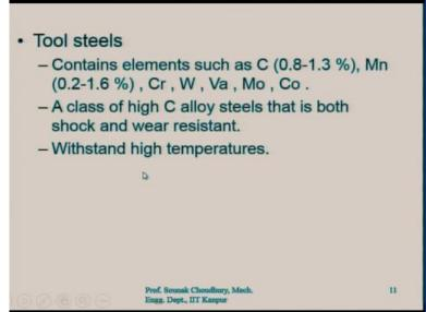
**Tool steels**: by name itself it means that the steels are used to make different kinds of tools for the conventional cutting process - single point cutting, tool milling cutter, drills and also for the metal forming operations dies, punches and so on. Now, tool steels contain elements such as carbon up to 1.3%, it is 0.8 to 1.3%, manganese, up to 1.6% starting from 0.2%. So, it is 0.2 to 1.6% of manganese, chromium then the wolfram that is the tungsten.
