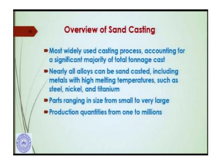
Overview of sand casting: I have already shown it to you the features of sand casting. Most widely used casting process, accounting for a significant majority of the total tonnage cast. Mostly the sand casting is used.
