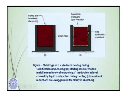
Here it is shown that molten metal is just poured into the mould cavity. Immediately after pouring of course, the level will be filled up I mean like this, there is no shrinkage, it is just filled up.
