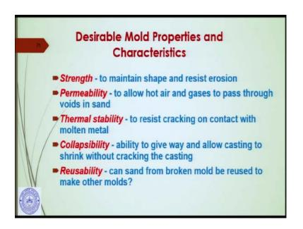
Desirable mould properties and characteristics: these five characteristics or properties are very important. One is the strength that is to maintain shape and resist erosion, because when the molten metal goes in it is very heavy and it may create turbulence, it will have a particular velocity, initial pouring velocity that may actually destroy the mould if it does not have the appropriate strength. We are talking about the sand mould, expendable mould.
