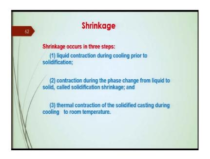
It will happen during the liquid contraction, during cooling prior to the solidification. Just before the solidification starts, the cooling process started in the molten metal. And, because of that the contraction happens.
