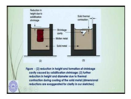
Reduction in the height due to solidification has taken place and here we have the shrinkage cavity. All around this is actually solidified and this is the area where the molten metal is left over. And, then it can be shrinkage cavity like this. When this will be solidified finally, there will be a shrinkage cavity, this kind of a shrinkage cavity.
