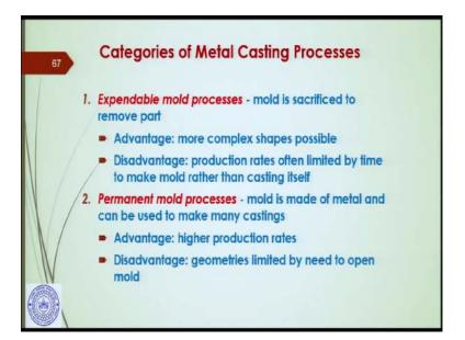
Now, let us see the categories of metal casting processes. These are basically two types expendable mould processes and permanent mould processes. I already told you in the very beginning that there are two types of moulds; expendable moulds and the permanent mould.
