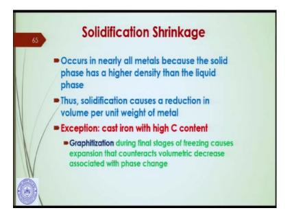
Solidification shrinkage occurs in nearly all metals, because the solid phase has a higher density than the liquid phase. Thus, solidification causes a reduction in the volume per unit weight of metal; this will always happen because the solid phase will always have a higher density than the liquid phase.
