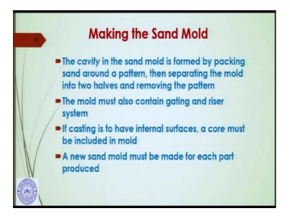
Making the sand mould: you have seen the steps in the video clips. Now, I am repeating so that it stays in your mind. The cavity in the sand mould is formed by packing sand
