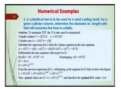
Now, the second example based on the same principle, that is the Chvorinov's rule. It says, a cylindrical riser is to be used for a sand-casting mold. For a given cylinder volume, determine the diameter to length ratio that will maximize the time to solidify. This question is little tricky, little different than the earlier one.
