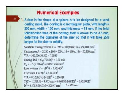
This is a direct application of the Chvorinov's rule in practice through the numerical example. It says that a riser had to be designed in the shape of a sphere, that is for the sand mold casting and the casting has to be a rectangular plate with 200 millimeter length, 100 millimeter width and the 18 millimeter thickness.
