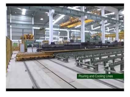
So, in those cavities the molten metal is poured and then it is cooling down. So, the solidification takes place.
