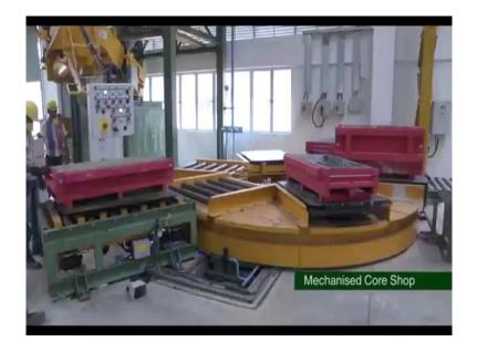
That is very big. So, this is a mechanized core shop where the cores are made. And, cores are introduced, you can see that these are the carousels.
