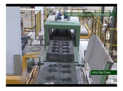
And they are getting into the automatic line here. Mould are going to the infrared oven for baking.
