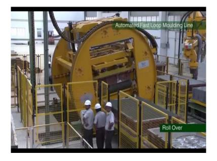
Here, you can see the turning; see now it is getting rolled over. And, you have seen in the first video that this is done manually, but here it is the automated first loop molding line. This is the rolling over of the mould.
