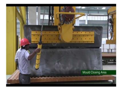
This is the closing of the mould. So, this is called the mould closing area. Here it is turned around.
