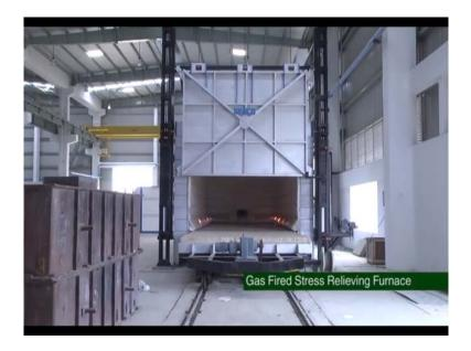
And, the gas fired stress relieving furnace, because after casting there could be some internal stresses remaining.
