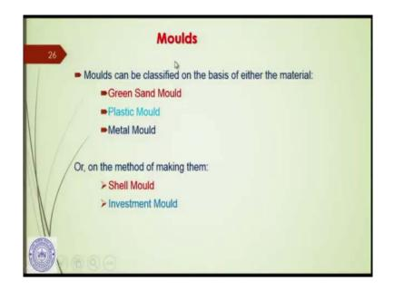
Moulds can be classified on the basis of green sand mould, plastic mould, and the metal mould. Depending on what kind of parts that you are getting, what kind of castings that you will be getting.
