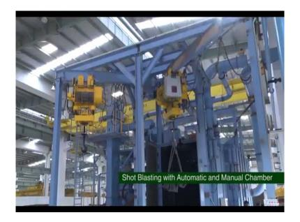
After taking the castings out, they go through the sand blasting with automatic and the manual chambers. With the help of the sand blasting the appropriate surface finish is obtained.
