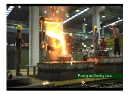
So, the pouring of the molten metal is done; you have seen earlier that the cavity has been made.
