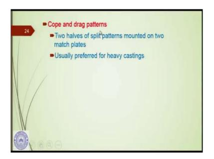
Cope and drag patterns: these are two halves of split patterns mounted on two match plates. So, this is the kind of the match plate, that I have shown to you earlier; usually preferred for heavy casting. So, when the casting is very heavy along with the match plate, there are two halves of the split pattern mounted on the two match plates additionally.
