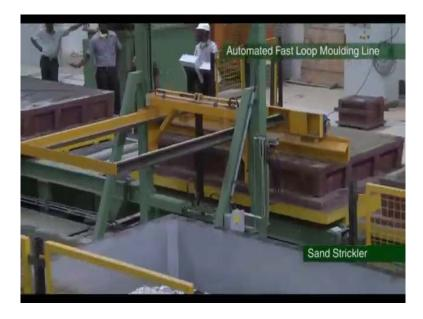
Here the cores and the pattern are placed; sand is poured on top and this is rammed.
