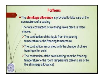
Now, the shrinkage allowance is provided to take care of the contractions of casting, I already told you. During the solidification it contracts. The total contraction of a casting takes place in three stages during its solidification. The contraction of the liquid from the pouring temperature to the freezing temperature. As soon as it is poured, from the pouring temperature up to the freezing temperature there is a contraction.
