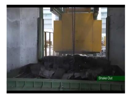
Because, it is a sand mould, so, the final product or the casting will be taken out.
