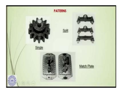
Here are different kind of patterns which are shown for example, this is a single pattern. Now, in the single pattern, this is one pattern which will make a cavity of this shape, where we have the shape of a gear or it can be split more than 1.
