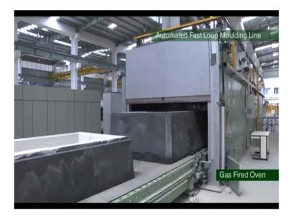
So, now the mould is made for the pouring of the molten metal, and placing of the cores and so on,
