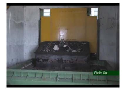
And, here with the help of vibration it is being shaken and the mould is broken.
