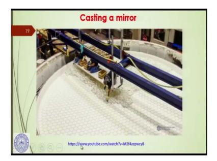
Here, again there is a link given and you can use this link to see this video in the YouTube, this is very important and very interesting video; this is casting of a mirror. How the casting of a mirror is made. And, just imagine that this is also made by the casting process. You can see the entire process; there is a good video, here is the link.
