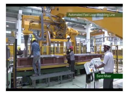
This is for the pouring of the sand in the mould. So, this is the sand mixer and you can see this is all automated.
