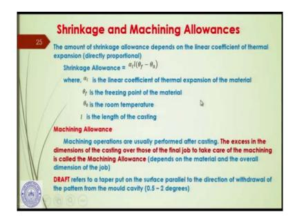
Now, let us see the shrinkage and machining allowances, how they can be estimated, and which factors should be taken into consideration while calculating, while giving the shrinkage and the machining allowance. Because, as you understand that depending on the amount of shrinkage
