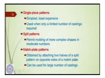
Single piece patterns like this, are the simplest, least expensive of course, because it is easy to machine, and it is simple. Used when only a limited number of castings required. So, they are not very complicated. One single pattern will actually make the cavity and they are used for the limited number of castings not in large number.
