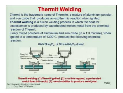
This is another interesting welding process which is called the Thermit welding. This thermit welding is schematically shown here. This is used popularly for welding of the railway tracks. Wherever there is a defect, it can be carried to that place. This is the mold
