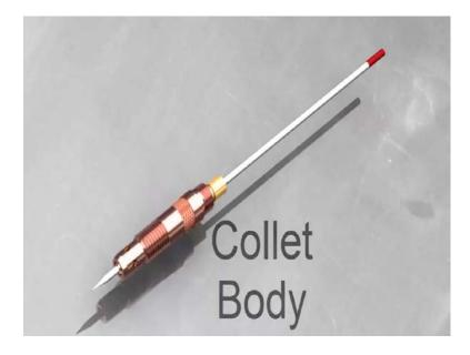
You can adjust the length that the electrode sticks out of the holder by loosening up the end cap.
