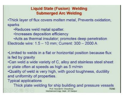
The characteristics are the following. Thick layer of flux covers the molten metal, prevents oxidation and the sparks, reduces weld metal spatter, increases deposition efficiency; acts as thermal insulator. The heat is not going out, it will be staying inside.
