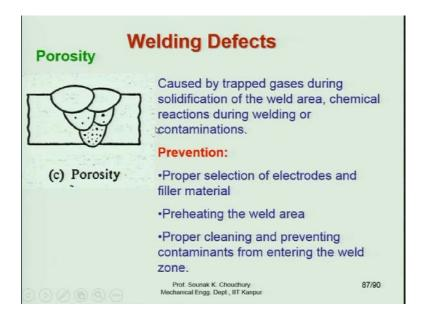
Porosity is another welding defect and in case of casting we have seen that porosity occurs because of the gas which is evolved and here are the three ways how to prevent them; proper selection of the weld of electrodes, preheating the weld area, proper cleaning and preventing the contaminants.
