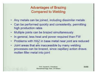
Problems with the heat affected zone in the base metal near the joint are reduced here in this case. This is one important point here.
