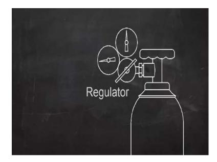
The pressure is reduced to a usable level by a device called a Regulator.
