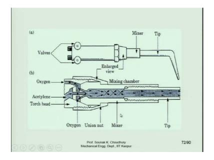
Here is the gun. There are valves to adjust, mixer, this is the tip and then, oxygen and acetylene will be passed through as you can see here in the cross section and here, it will be burned. They are mixed together, and the gas will be burn here. This is the mixer, this the union, this is the union nut so that the flow can be regulated, this is the torch head through which the oxygen and the acetylene gases pass through in the mixing chamber.
