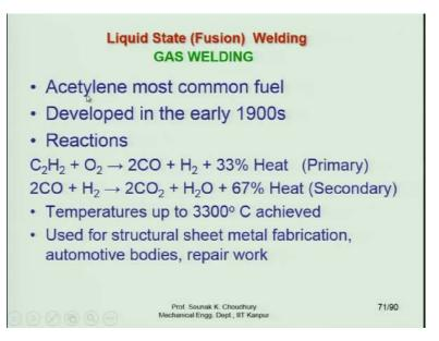
The acetylene is most commonly used for the gas welding. This is also a fusion welding or the liquid-state welding as I mentioned earlier. This gas welding was developed in the early 1900s and you will find this welding process in most of the road-side repairing shops, for automobile repairing or scooter repairing, gas welding is very popularly used.
