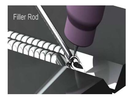
Now, you can TIG weld with or without filler metal and that is not a choice, you have in a lot of other processes. If you want to add filler metal to a TIG weld, you use a filler rod which is just a rod of metal with a specific Galloway. You want to make sure that the filler metal, you are using is compatible with the base metal and that it has the strength required to do the job.
