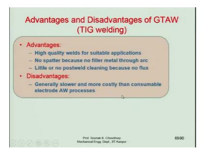
Advantages and disadvantages of the TIG welding are the following. Advantages: these are the high-quality welds for suitable applications. A high-quality weld basically because you do not have the slag on top of that, that is once again I am repeating, there is no slag so there is no further processing required and the surface quality will be better. No spatter because no filler metal through the arc is used.
