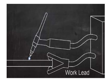
The current has to flow in a complete circle from the machine to the torch into the work and back to the machine. A work lead is clamped to the work to complete the circuit from the work piece back to the machine.
