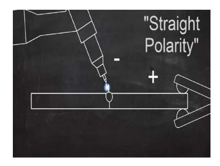
The DCEN is a more descriptive term. DCEN put most of the heat on the work piece.
