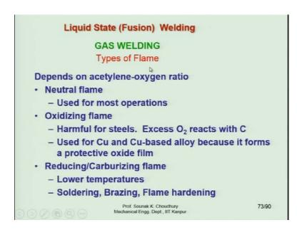
Types of flame: This is very important in the gas welding that depends on the acetylene and oxygen ratio. A neutral flame is used in most operations. Oxidizing flame is harmful for steels because excess oxygen reacts with the carbon. Used for copper and copperbased alloy because it forms a protective oxide film. Reducing or carburizing flame has lower temperature. It is used in the soldering, brazing, flame hardening because there the temperature required is not very high.
