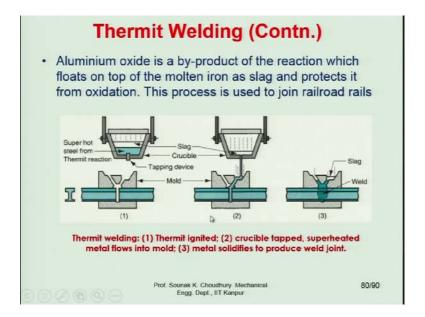
Aluminum oxide is a byproduct of the reaction, which floats on top of the molten iron slag and protects it from oxidation. The process is simple. This is the diagram, and you can see that these are the three stages which are shown here.
