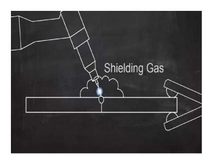
In TIG welding, the molten metal is protected by a shielding gas. This gas usually argon and sometimes helium or other gases, keeps the molten metal from reacting with oxygen water vapor in the atmosphere.
