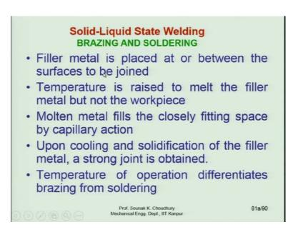
Filler metal is placed at or between the surfaces to be joined. Temperature is raised to melt the filler metal, but not the work piece. This is important here. Molten metal fills the closely fitting space by capillary action.
