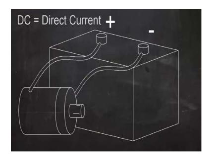
For most metals, the current is direct current or DC. DC is like the current flowing from a car battery; one wire is always the negative and one is always the positive. DC TIG welding, the electrode is usually negative and the workpiece is positive.
