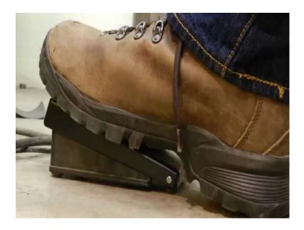
You can control the amount of heat with a foot pedal or with a thumbwheel on the torch.
