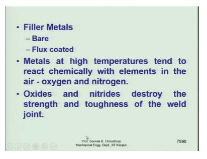
Filler metals: they are either bare or flux coated. Metals at high temperatures tend to react chemically with elements in the air oxygen and the nitrogen. Oxides and nitrides destroy the strength and toughness of the weld joint of course. So, this is the disadvantage.
