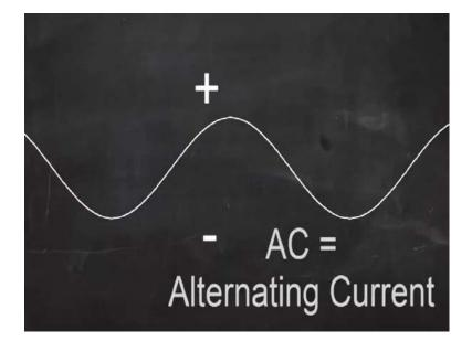
When welding aluminum, however, AC is used. In AC, the positive and negative voltages switch back and forth between the electrode and the workpiece and this puts more heat on the electrode, but it has a cleaning effect on the workpiece. You see aluminum forms oxides that floats to the top of the weld pool and prevent a good weld. AC current helps control these oxides.
