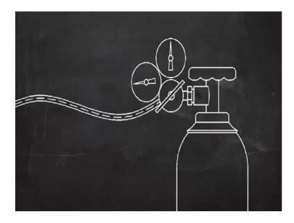
The shielding gas flows through a hose and comes out right at the point of the weld.
