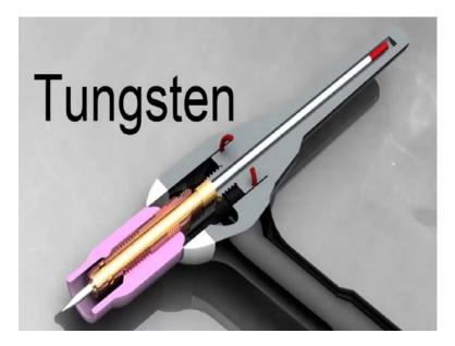
And tungsten has an extremely high melting point, when you TIG weld, the electrode gets hot; but it does not melt. We say that it is a non-consumable electrode.
