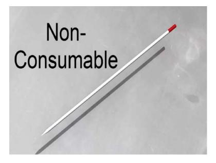
And it does not mean it lasts forever that just means that it does not melt and become part of the weld.
