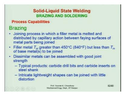
In case of brazing, the important thing is that filler metal temperature is greater than  $450^{\circ}$  C; but less than the melting temperature of the base metal. Dissimilar metals can be assembled with good joint. Typical products are carbide drill bits, where you cannot have the high temperature to avoid the thermal distortion.
