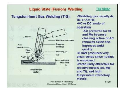
This is the schematic diagram. I will show you a small video as well. The Tungsten-Inert Gas welding: here the shielding gas normally used is argon, helium or together argon and helium. Both AC or DC mode of operation can be used. AC preferred for aluminum and magnesium because as aluminum and magnesium when it is available normally, a layer of oxide is formed on the surface; aluminum oxide or magnesium oxide.
