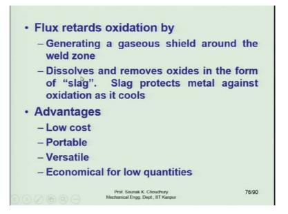
Flux retards oxidation by generating a gaseous shield around the weld zone and this is the "slag"; advantages are that it is low cost; portable, it can be taken to any places; versatile; economical for the low quantities. (Refer Slide Time: 19:31)
