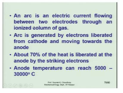
An arc is an electric current flowing between the two electrodes and 70% of the heat is liberated at the anode striking electron and the anode temperature can reach up to  $30000^{\circ}$ C.
