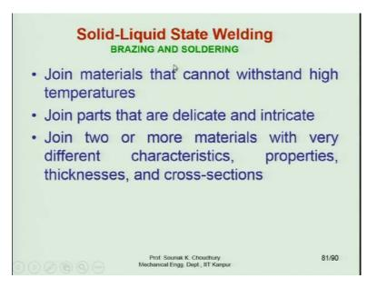
Brazing and soldering, as I said in the beginning, are performed at a lower temperature that join materials that cannot withstand high temperature.
