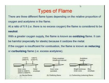
These are the three types of flames that you have seen; here it is the bright luminous inner cone in the carburizing flame. In the oxidizing flame this inner cone is pointed and here is the outer envelope that is small and narrow. Here, you can see that there is a blue envelope and inside that is called the acetylene feather.
