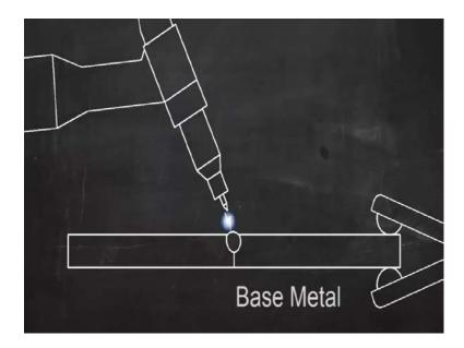
That is the metal that makes up the two pieces that are to be joined the heat is generated by an electric arc that forms between the base metal and the tungsten electrode.
