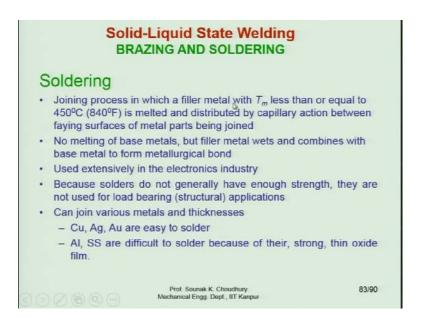
Soldering is a joining process in which a filler metal is used with the melting temperature less than or equal to the  $450^{\circ}$  C. In case of brazing, it is greater than  $450^{\circ}$  C, but much less than the melting point of the base metal. Here, it is less than or equal to  $450^{\circ}$  C.
