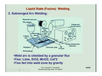
Submerged arc welding: this is the simple process, which is very popularly used, and this is the entire setup. It is shown schematically. There is a flux hopper through which the solid flux material is delivered to the welding zone. This is the wire feed motor which feeds the motor from the spool. This is the wire reel, and this wire is the electrode.
