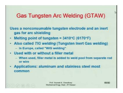
I will remind you that in our last session, we started discussing the Gas Tungsten Arc Welding and which is also called the TIG welding or WIG welding. this is used with or without a filler metal as I said and then, the application is for aluminum and stainless steel. These are the most common materials.
