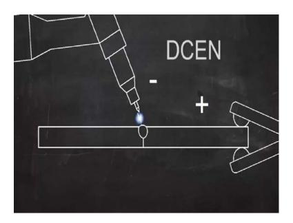
The term DCEN is used for this indicating that the current is DC and the electrode is negative. This is also called "Straight polarity".
