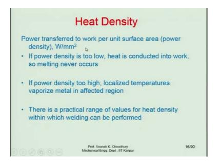
Heat density; power transferred to work per unit surface area. This is  $\left[\frac{Watt}{mm^2}\right]$ . I already told you that in some of the welding processes, I showed it to you in a tabulated form how different kind of welding processes, how much power they need or the power density they need. This is in  $\left[\frac{Watt}{mm^2}\right]$ . If power density is too low, heat is conducted into work.
