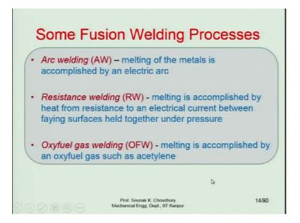
Some fusion welding processes are the following. Arc welding; arc welding is probably one of the most commonly used welding processes. Melting of the metal is accomplished by an electric arc. An electric arc is produced by the anode and the cathode positive and the negatively charged electrodes. Resistance welding is another process where melting is accomplished by heat from the resistance to an electric current between the faying surfaces, held together under the pressure that we will discuss.
