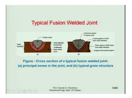
Here we can see the fusion zone, where the fusion process taking place. This is the fusion zone. Weld interface is here; weld interface is between the fusion zone and the heat affected zone. Heat affected zone is the zone, where the structure of the material has
