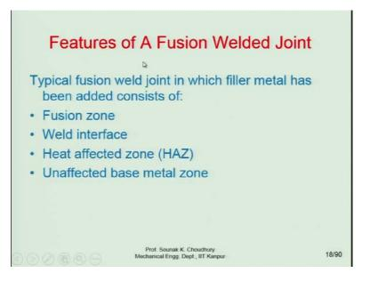
Features of a fusion welding welded joint: These are the following four features. Typical fusion weld joint in which filler metal has been added consists of the fusion zone one, weld interface, heat affected zone and the unaffected base metal zone. These are the basic four features in the fusion welding process.
