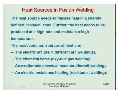
Heat source; the heat source needs to release heat in a sharply defined isolated zone. Further, the heat needs to be produced at a high rate and maintain a high temperature. This is the characteristic of the heat source. It has to be sharply defined, isolated zone and it has to be produced at a high rate and this also should maintain a high temperature. It should not lose its temperature.
