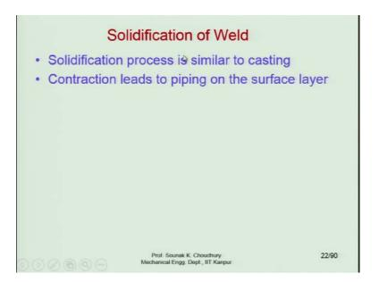
Solidification of weld: the solidification process is similar to casting as I said. Contraction leads to piping on the surface layer.
