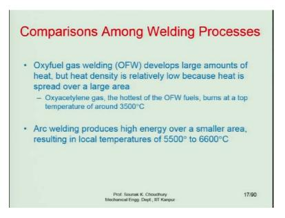
Comparison among the welding processes: the oxyfuel gas welding develops large amount of heat, but the heat density is relatively low in the case of the oxy fuel gas welding. Because the heat is spread over a large area. Now, as an example, I told you about those ion beams or the beam technology. In beam technology, it is concentrating at a very tiny spot and by tiny, very tiny I mean to say that it can be in micron level.
