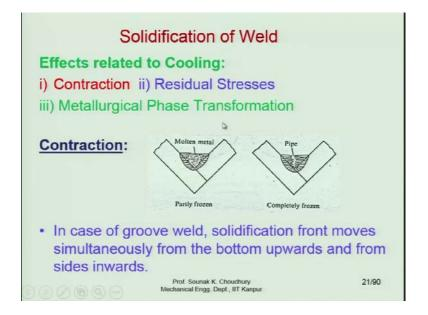
When cooling down, like in casting, in welding also in the welded zone, it can have the contraction or the shrinkage, that we have seen in casting. Therefore, it may have residual stresses and the residual stresses can adversely affect.
