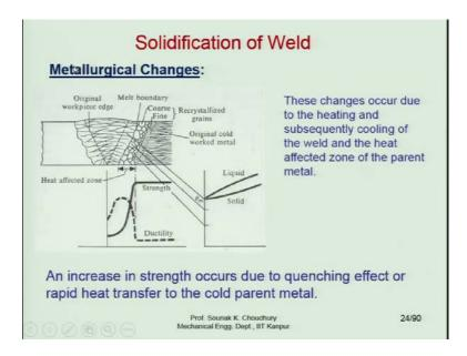
Now, the third feature in the metallurgical changes. Here are the metallurgical changes given in details and here if you see the original work piece edge here given in the dotted line. This is the melt weld pool and the melt boundary is here. This has been melted. Here we have the coarse grain in the heat affected zone. This is the heat affected zone and we have mentioned that in heat affected zone, we will have both cold grains and the finer grains.
