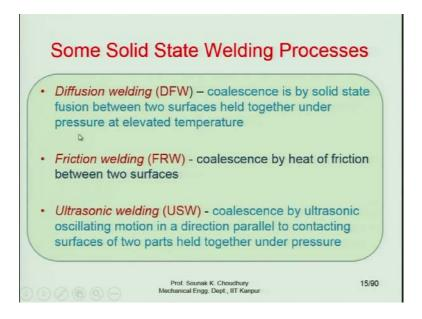
And these are the processes like diffusion welding, friction welding and the ultrasonic welding, where we weld the parts in the solid state. Here, the base metal is not melted. The diffusion welding coalescence is by solid state fusion between the two surfaces held together, under pressure at an elevated temperatures. Temperature is higher and at certain pressure which is exerted to the two parts that are joined together.
