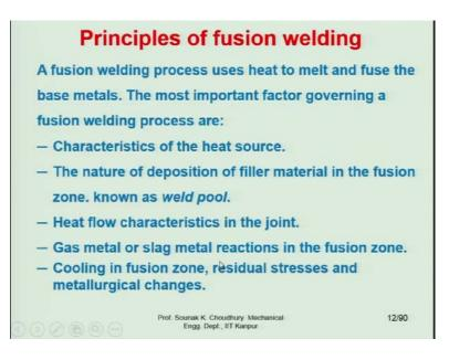
Now, let us see the principles of fusion welding. A fusion welding process uses heat to melt and fuse the base metal. The name itself says that this is the fusion welding. The base metal has to be fused, has to be melted. These are the five very important factors for the fusion welding.
