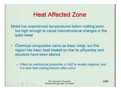
Heat affected zone: metal has experienced temperatures below melting point. It is not yet melted, but high enough to cause micro structural changes in the solid metal. Keep in mind that the heat affected zone is highly heated up because of the fusion taking place in the adjoining areas.
