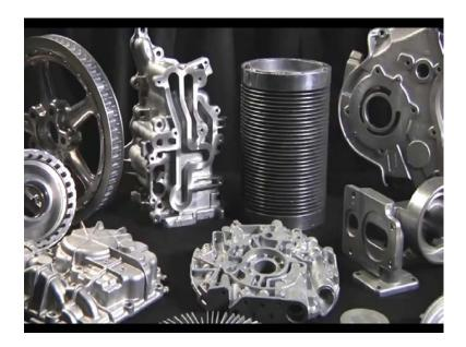
Die cast parts can be sharply defined with smooth or textured surfaces and are suitable for a wide variety of finishes.
