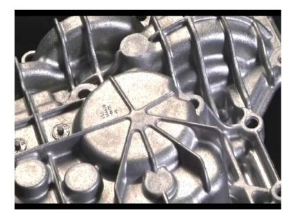
These dies can be engineered to produce complex shapes with a high degree of accuracy and repeatability.
