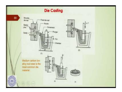
If you see the slide here, these are the two parts; one is fixed, one is movable. And there are ejector pins to facilitate the ejection of the part, which is here, which will be formed here. After the molten metal is solidified, this is the cavity. Now, when the two halves are joined together, the cavity is formed and the molten metal can be forced into this cavity; normally it is pumped from at a high pressure from chamber .
