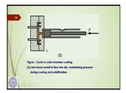
Cycle in cold chamber - second cycle is the ram forces metal to flow into the die; maintaining pressure during the cooling and the solidification. So, it will stay like this for sometimes till the molten metal gets solidified. Here also you can see that ejector pins and as it moves towards the left, ejector pin will help in removing the casting from the cavity.
