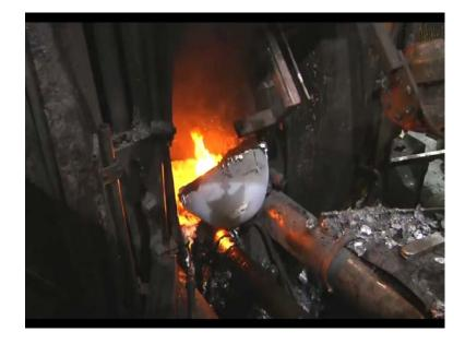
Next pre-measured amounts of molten metal are injected into the dies at extremely high pressures.
