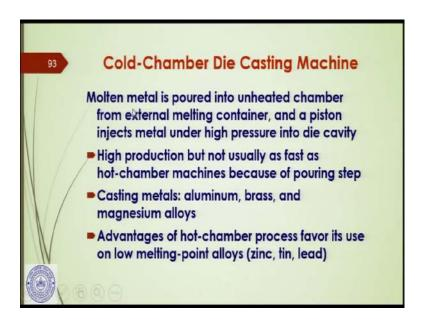
Now, molten metal is poured into the unheated chamber, this is the cold chamber; we have talked about the hot chamber, when it is heated up. And when it is cold chamber,
