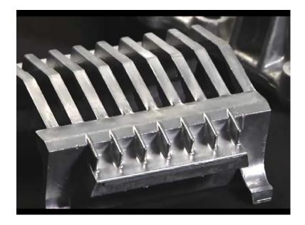
This high pressure process produces a dense, fine grained surface structure with a wide range of physical and mechanical properties, such as fatigue strength.
