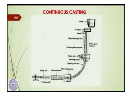
This is another type of casting, which is popularly used when we need very long rods for example or railway lines for example, this is a continuous casting. Here we have the ladle, where the metal is melted, and the molten metal is kept here.
