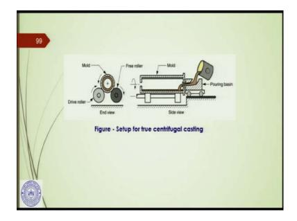
Here is the setup. For giving you an idea, this is the side view. What we have here in the centrifugal casting is the mold; as you can see that this is a cylindrical mold with a cavity inside. And this is rotated by the drive roller and this is the mold shown in sectional view.
