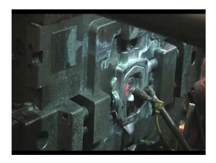
The newly formed part is then removed from the dies and the cycle is repeated after the die cools.
