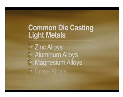
The ones that are often used for die casting are zinc, aluminium, magnesium and brass alloys. So, this is a small clip through which you could see how intricate shapes and how good accuracy parts can be produced, castings can be produced in the die casting. Either it is a hot chamber, or it is a cold chamber process.
