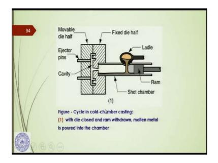
Here are the cycles in the cold chamber casting; this is the fixed die, and themoveable die half, like in the case of the hot chamber. But here this is absolutely different as you can see.
