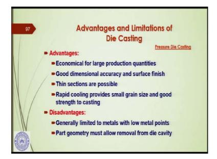
Now, the advantages and the limitations of die casting are the following. Advantages are the economical for large production quantities, good dimensional accuracy, and surface finish; because it is the permanent mold casting. Its characteristic feature I told you earlier of the permanent mold casting.
