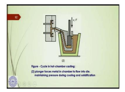
Cycle in hot chamber casting - continuing plunger forces metal in chamber to flow into the die, maintaining pressure during the cooling and the solidification. What is said here is that the die is closed, and plunger withdrawn, molten metal flows into the chamber.
