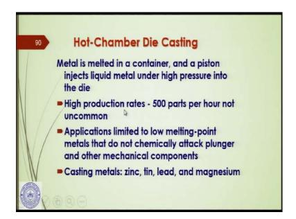
And here it is written what I have said already. In case of the hot chamber die casting, metal is melted in a container and a piston injects liquid metal under the high pressure into the die. The high production rate up to 500 parts per hour, this is not uncommon.
