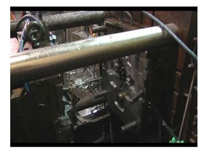
In the die casting process, the reusable steel dies or molds are preheated and coated with a die release agent to lubricate and protect the surfaces of the dies before each use.
