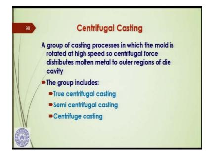
Now, there is another method of the casting which is also very important, and which is also very widely used, this is called a centrifugal casting. The name itself says that there is a certain centrifugal force that is used for forcing the metal into the cavity. A group of casting processes in which the mold is rotated at high speed, so centrifugal force distributes molten metal to outer region of the die cavity.
