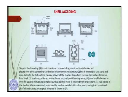
So, let us see what is the shell moulding and how the shell moulding process is performed. It is an interesting process, if you see there are six steps shown here. In the first step, there is a box; inside the box, the sand with the resin binder is kept dry.
