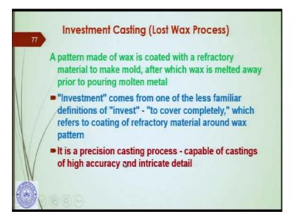
Let us now discuss the investment casting; as, I said that investment casting is called the Lost Wax Process. Now this is one of the oldest processes, a pattern made of wax is coated with a refractory material to make the mould, after which the wax is melted away prior to pouring molten metal.
