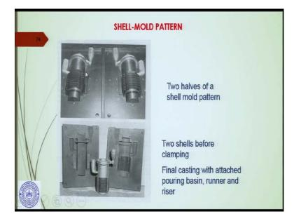
Now, these are the different kind of shell mould patterns. These are the two halves of a shell mould pattern. And, this is how the final casting is made. This is the mould cavity that you are making; two shells before clamping, final casting with attached pouring basin, this is the pouring basin which has to be segregated along with the runner and the riser.
