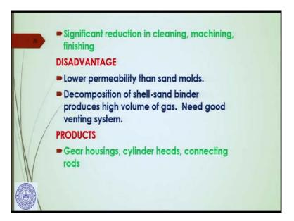
Significant reduction in the cleaning, machining, and finishing; therefore, because the surfaces are smoother than in case of the sand moulding; so, the cleaning process, machining process, finishing process are reduced. Disadvantages are there. First of all, the lower permeability than the sand mould, because the sands are closely packed here in case of the shell moulding, than in case of the sand moulding.
