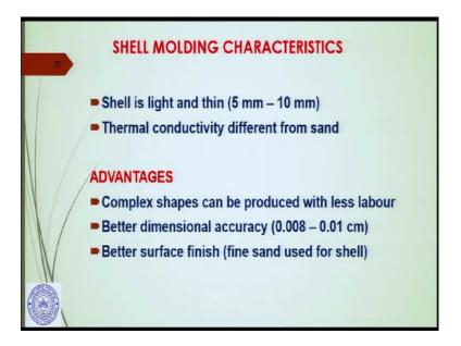
Now, the shell moulding characteristics are the following - that shell is light and thin. So, the shell thickness is about 5 to 10 millimetres. As you can see that with the material being sand and the clay and with 5 millimetres to 10 millimetres thickness, the shell itself will be very light.
