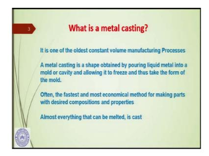
Now, let us see what is metal casting? How we can define casting? It is one of the oldest constant volume manufacturing processes where, as I said, the volume remains the same for the final product and the initial blank, there is no change in volume, A metal casting is a shape obtained by pouring liquid metal into a mold or a cavity and allowing it to freeze, after which it takes the form of the mold.
