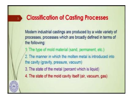
Let us see how the casting processes are classified. Modern industrial castings are produced by a wide variety of processes, which are broadly defined in terms of the mold material first of all. By mold material we mean to say that, what kind of sand materials, sand we are using; whether the mold will be permanent, or the mold will be once used type?
