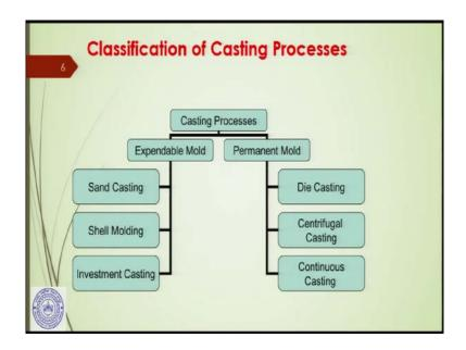
Here is the full classification. This diagram shows that casting processes are basically classified into two groups; one is the expendable mold and another is the permanent mold. I just told you about the expendable mold that, this is expended, that is, it cannot be used more than once.
